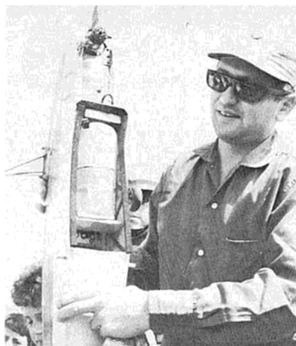
Fuel system arrangement, simple. Planes carried 63 oz. Feiner checks fuel remaining after 73 mile trek. K&B consumed .4 oz./min. for 1 hr.-34 min. duration.
