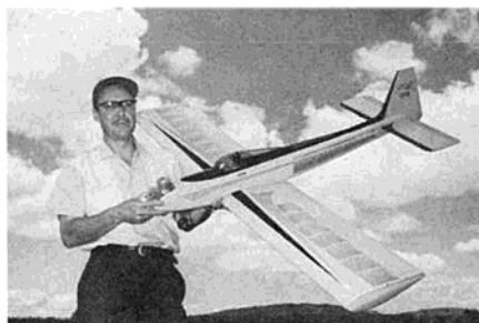
Kwik-Fli I & III combination of Amelio Lozano showed outstanding workmanship seen in many Mexican models. Slimmer 15% airfoil, Super Tigre 60G effective for Mexican altitudes.
