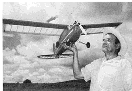
Spirit , from German plans by Jose Lomeli of San Luis Potosi, was 6 year old escapement rudder ship. Uses Orbit relay tube receiver with Bonner SN and compound escapements. Fox 19, 3 lbs., 54".
