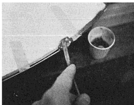
Neatness in applying putty will greatly reduce the chore of finishing the deck edge.
