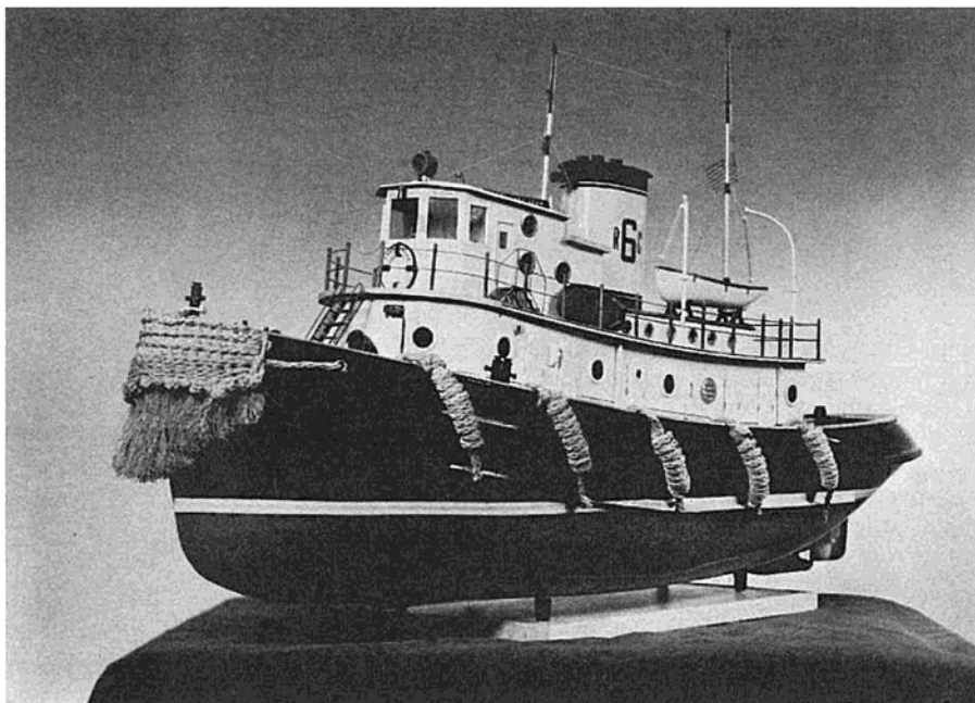
Alan Boyer's magnificent scratch-built 48" version of the Wilmington, Delaware tug "Long Beach." Citizen-Ship 10, twin Pittman 12V motors.
