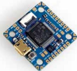
**Flight Control OMNIBUS F4 Nano V7**
