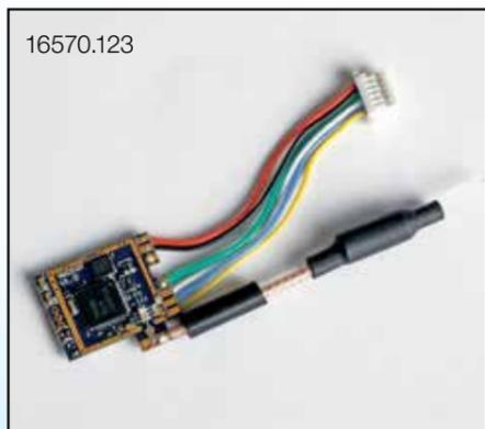
**FPV Sender Raceband 5,8 GHz 25 mW**
