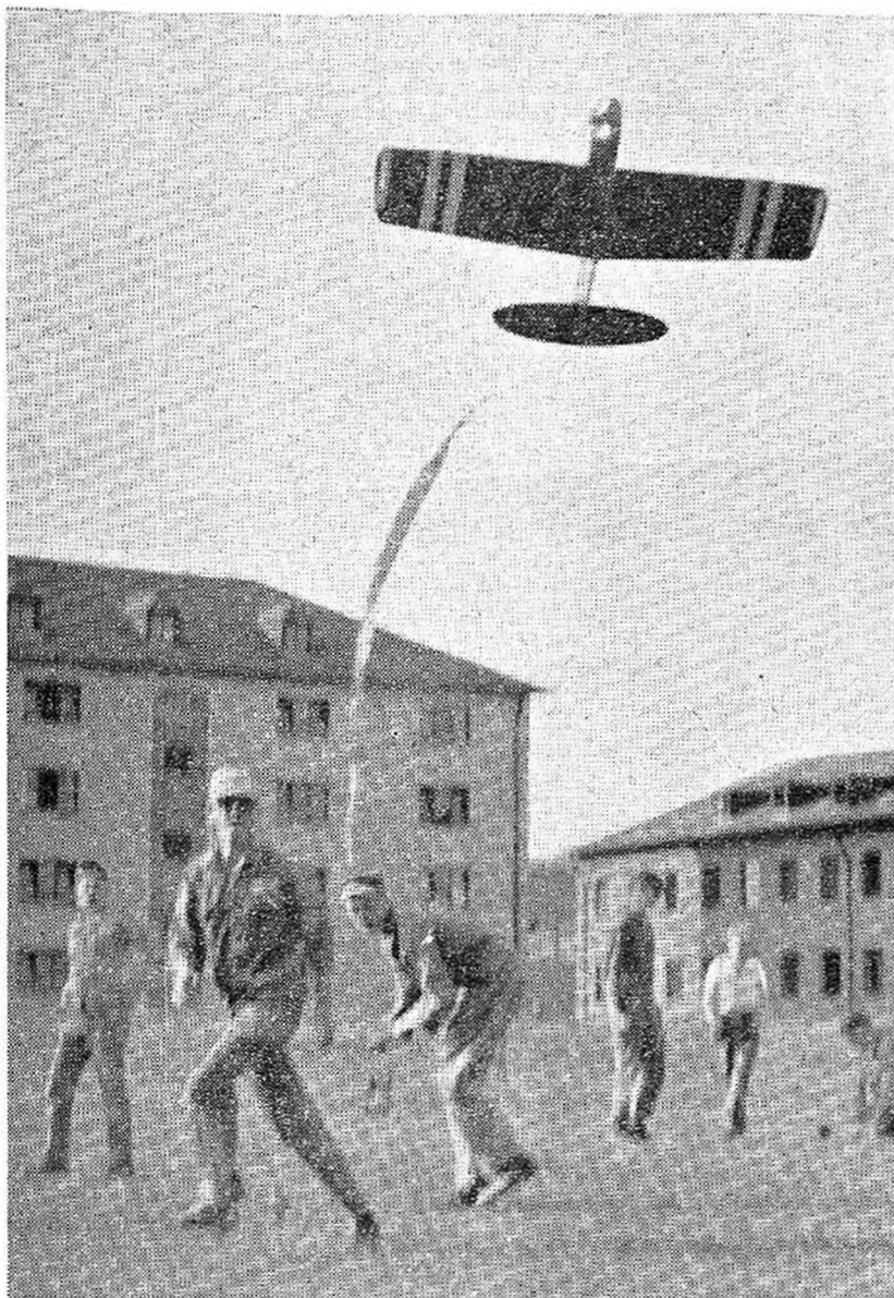
Action launch at the U.S.A.F.E. Championships, Wiesbaden. Model is a commercial design for .35 cu. in. engines and has a cast alloy fuselage to make it unbreakable. Two helpers are needed for launch to see that streamer gets a clear release
