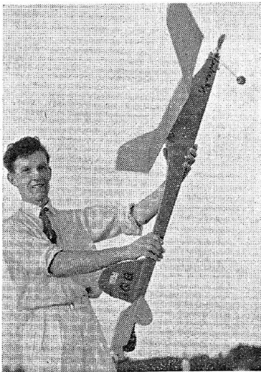
At left, the Loughborough College pendulum-controlled elevator is demonstrated by Max Byrd. Elevator goes down at this angle of climb. Below is the Austrian approach to a forward keel with a large fin over centre section
