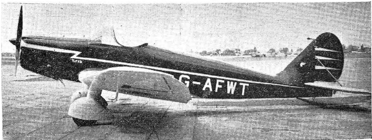
BELGIAN 2-seater. Built in England pre-war, the aerobatic 62 h.p. Topsy Trainer has built-in slots and pronounced washout.
