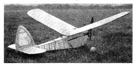
Steep dihedral, deep belly and large fin, typify Colonel Bowden's model designs, this one being the Porlock Puffin of 1939/40 vintage. Introducing streamlining to the power model, yet still retaining a cabin on a performance model, was the famous Elbert J. Weathers' "Mystery Man". Unique features were "vee" tailplane, dropoff dolly undercarriage and eliptical dihedral for wings.
