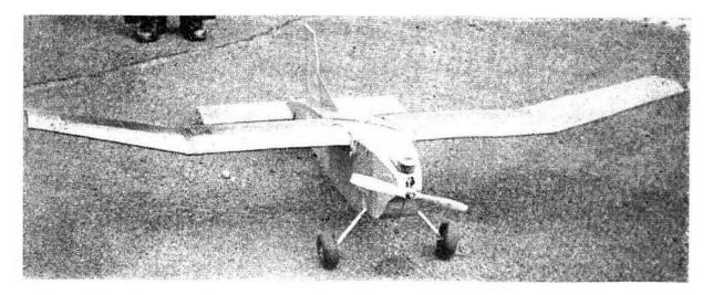
Completely re-designed model which won King of the Belgians Cup for the Equipe Gobeaux. Micron 60 engine is retained, still without engine control, u/c is fully sprung, and full length of elevator span utilised for control movement.
