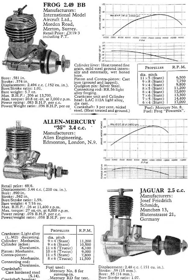
Crankshaft bearing: Meehanite bush.
