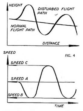
On the way up it will fly slower, point B of Fig. 1, on the way down it will pass through the correct speed, point A of Fig. 1, and then go on to or beyond the speed of point C in Fig. 1.
