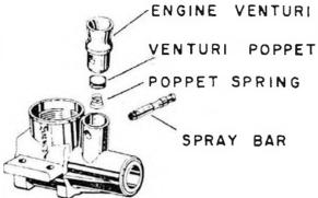
ENGINE VENTURI of which may sound confusing, so we shall deal with one at a time.
