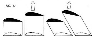
Fig. 17. Diagrammatic comparison of torsional stresses on normal and swept forward wings. When sweeping angle is positive (sweepback) the wing tips generate more lift, due to boundary layer density increase. This means a higher stress (statically) on wing structure ( $C_1$  factor is stepped up) and the stall will occur earlier. To counteract this, wing must be washed out, which means, again a *lesser* overall lift generated from the total wing.
