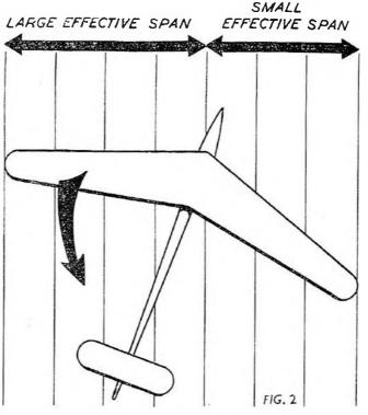
This induces a greater number of boundary layer particles at wingtips, which in turn produce a very early wing stall. With a model, such an early stalling tendency is even more evident, owing to the boundary layer being more sensitive and critical and less "adherent" to wing, in view of reduced air speed. However, to obtain the lowest sinking speed, one should have the maximum overall lift possible.
