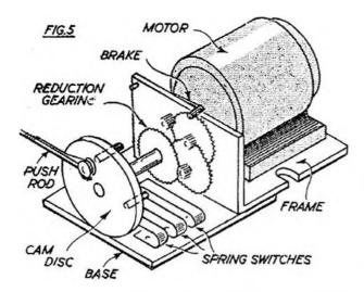
torily, even a simple pulley drive, although this is getting away from one of the basic advantages of motor servos of positive power drive. More intricate gearing schemes bring us back to the "watchmaking" class of precision work again.
