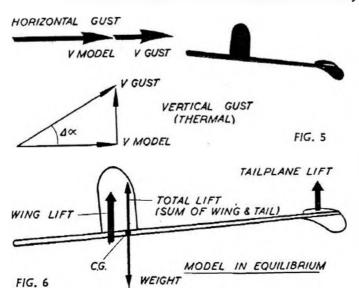
a change in lift on wing and tail. The horizontal gust causes this by the increase in windspeed, while the vertical gust increases the angle of attack.
