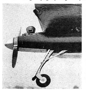
conventional spark - ignition motors. The glow versions ran faster and because they needed no ancillary equipment other than a starting battery, represented a considerable saving in weight. American ideas on engine design and production being geared to lightweight construction for engines, glow ignition was therefore doubly a more attractive feature.
