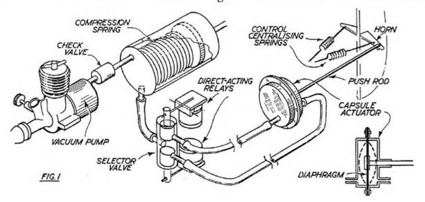
diaphragm. Depending on the pressure in the system and the area of the diaphragm, the actual force transmitted by the pushpull rod can be adjusted, as necessary.
