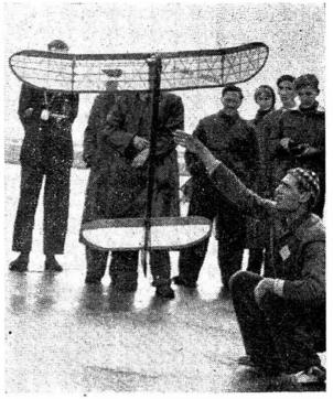
He bows to conquer! Coventry's Ron Draper, the 1956 World Power Champion ducks his head at every vertical launch. This is to get out of the way of the screaming OS MAX-1. IS engine and to ensure that all three VTO points were well and truly in contact with terra firma. Model is all-red, known as Crescendo, and climbs in a steep wide spiral. Timer operates both the cut-out and an automatic rudder for the glide.
