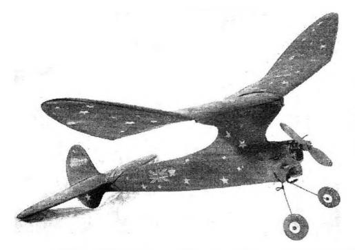
the fabulous Goldberg "Zipper" forerunner of the modern small pylon model and here as originally designed with a 6 c.c. Baby Cyclone petrol engine.
