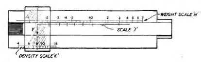
slide so that the thickness on scale J is against the weight found on scale H. Align the cursor with arrow Y and read off the corresponding density on scale K.
