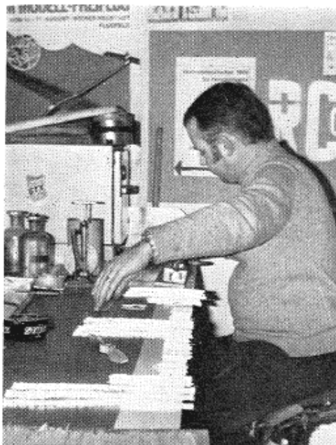
Starting the process, after cutting the glass strips and mixing epoxy.
