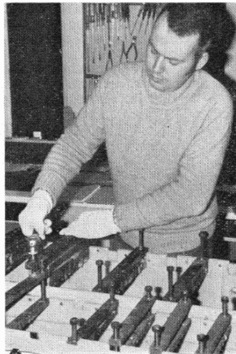
Below left: Fitting the upper mould half. Below right: Pressing out the excess epoxy from the mould and heating to 100°C.
