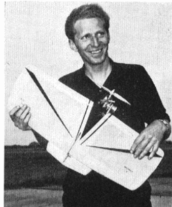
Pete Tribe developed his original Razor Blade until it looked like this (left) but still the basic layout remained, with \frac{3}{8} in thick section, \frac{1}{4} in sheet trailing edge and spruce spars. Mike Davis (right) simplified combat models with his Dominator - no spars, hefty leading edge and almost unbreakable when nylon covered.
