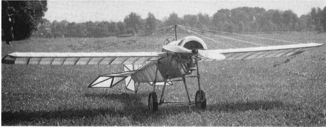
A nice slow, realistic flier is this Blackburn I912 Monoplane for Fox 25 R/C power – throttle control makes it all the more interesting in flight. The Aero Modeller free flight plan (FSP 567, price £1.15) could be adapted with hardwood spars, no wing incidence and stronger engine bearers.
