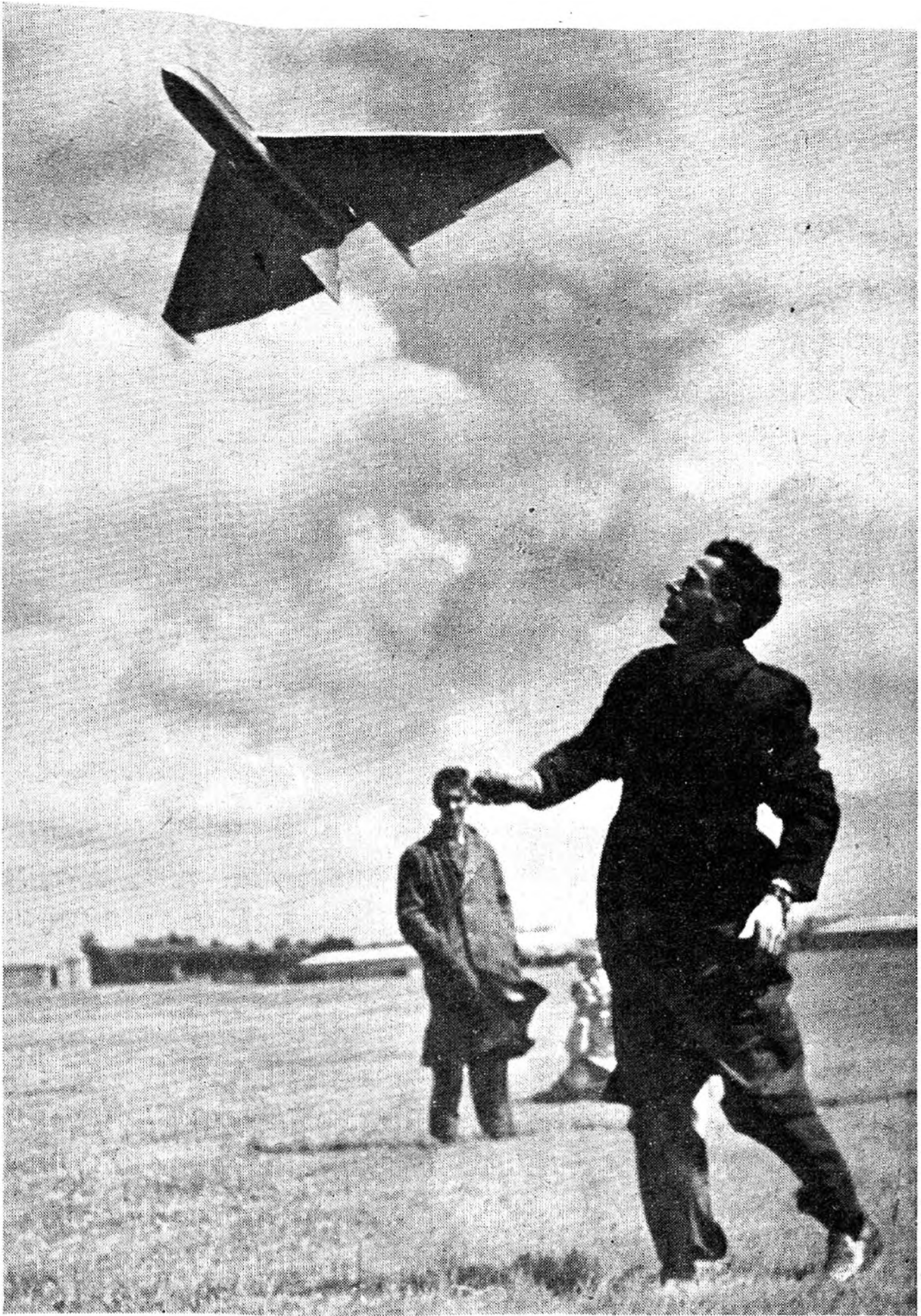
Typical of a Delta Year! Squadron Leader Laurie Ellis of Debden launching his version of this increasingly popular wing planform. Model is powered with an Ailbon Spitfire 1 cc. engine, has Clark Y airfoil section and an all-up flying weight of 30½ ozs.
