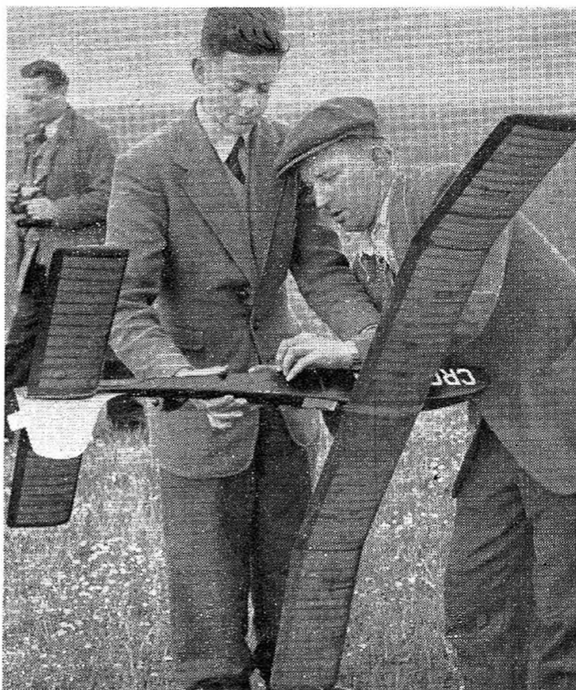
Jack North came second in trials with this 1950 sparless A/2, which has lin. rib spacing typical of such pastmasters as Chasteneuf, with whom he was fellow clubman in pre-war days.
