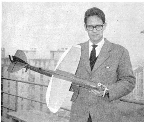
Franco Bugada and his remarkable Pagna P.C.7 model. Structural difficulty is that of balance with such a long nose using Super Tigre G20 15 glow engine.
