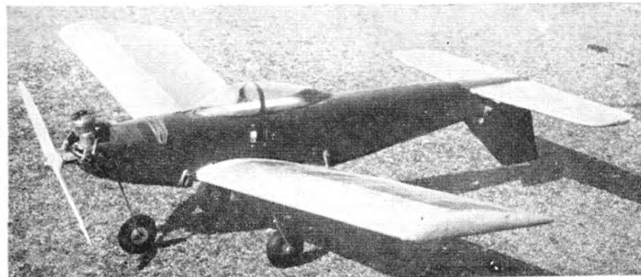
J. Singleton's small, rudder only, model using two channels of Orbit-10 Relayless and Bonner Transmice servo. Enya 15 engine.
