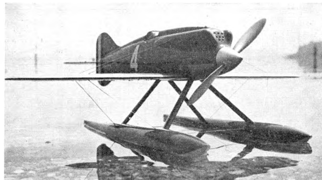
This is a model! Silvio Taberna's beautifully constructed winner of the first model Schneider Cup Race, as seen after a flight, note water droplets on under-surface of wing, also the opposite hand propeller to give torque assistance during the take-off stage, but still maintaining traditional anti-clockwise flight path.
