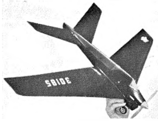
Swept wing F.A.I. team racer by Atkinson and Crofes qualified for semi-finals at Nationals with 4:34 using an Eta 15 engine.
