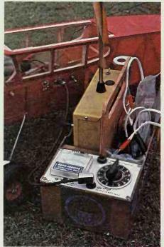
Above: A neat field-box carrying transmitter and test and charging equipment. Fast re-charge cells allow many flights during a session at the flying field.
