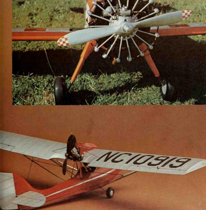
*Top left*. A four-stroke Kittiwake 10cc engine, designed in the 1930s, installed in a 2.5m (8ft) Vulcan model of similar vintage.
