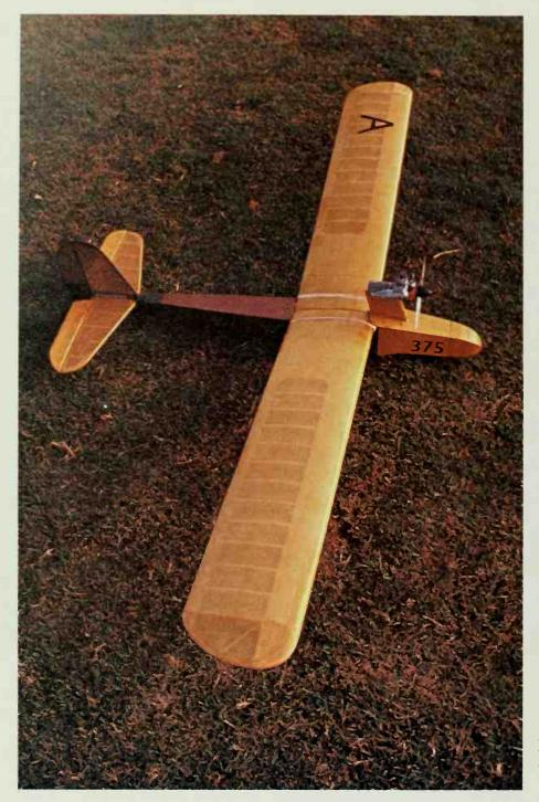
*Above:* A simple boxy model equipped with a power pod. The engine is a means of gaining height in place of a towline.
