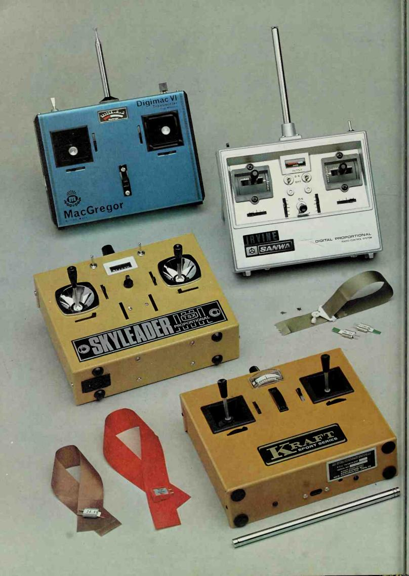
Probably the most frequently used aircraft radio is the four-function set, usually used to control rudder, elevators, ailerons, and engine. Examples of such sets, from Britain, Japan and the USA, are illustrated; the basic form is common, but there are detail differences in circuitry and mechanics and, to some extent, in size and weight. The standard of performance and reliability of modern equipment is remarkably high.
