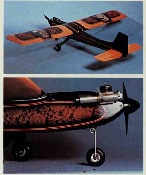
that requires only one or two thin coats of clear dope to provide the final tautening and fill the pores. Fragile structures achieve most of their strength from this method of covering but it must be approached with care. Light structures should always be carefully pinned down flat during shrinking to avoid warping.
