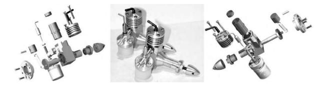
The scheme that uses the piston to control timing for inlet, exhaust and transfer is, for some reason, called "side-port", even though most all examples place the inlet at the back.
