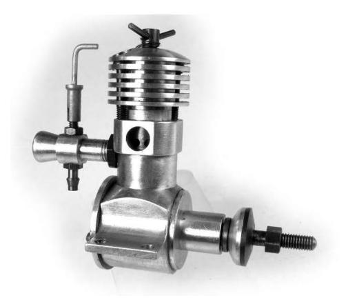
The EMBEE was made in Leicester by Moore and Bailey. It is a barstock engine, and quite nicely made and finished, inside and out. Sadly in the hand, in my view, it is an ugly lump.
