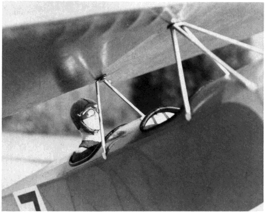
Two or three channels guide the 1/2A Sparrow II by Don Srull (at left). To simplify final finish and covering, Don builds aluminum tubes into the fuselage to receive plug-in wires such as the cabanes (above).
