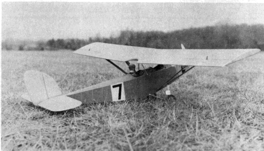
Schoolyard Scale returns to FLYING MODELS' pages with Don Srull's design of the Supermarine Sparrow II for 1/2A and two or three channel control. Don's plane keeps a promise he made in the October '82 issue.
