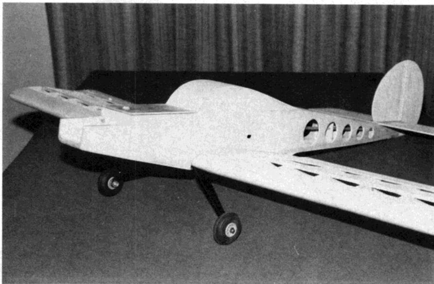
The completed framework shows the lightening holes in the fuselage sides. They're made of poplar ply and require no additional doubling. However, as a precaution, the author added bracing to the tail.
