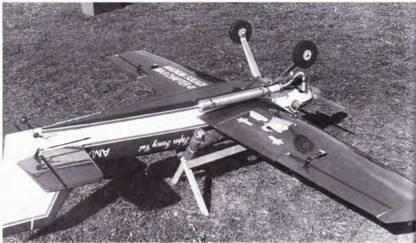
Large planes require more robust control linkages and servos. Don't skimp at this point, or the results could be a very large hole in the old flying field...or worse
