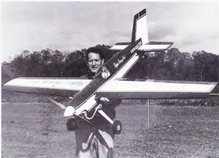
With Dave holding onto it, you can easily see the relative size of this great looking bird. It has a wingspan of 92 inches, and a very generous 1540 square inches of wing area. Build it light, and it will perform well.
