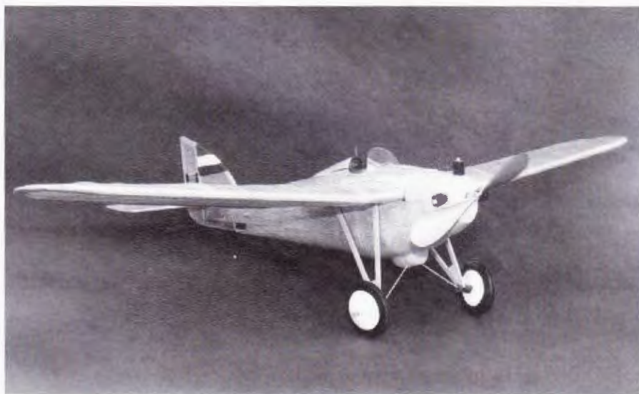
This "rare bird" is a 26-inch wingspan rubber-powered model of the Pander D, a Dutch lightplane of the 1920s. Harry Brown built this one, and covered the fuselage with 1/32 balsa sheet.
