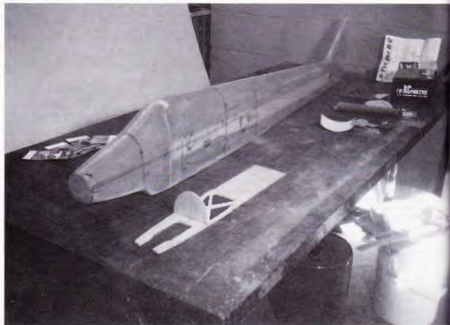
A 5-ply birch plywood crutch is fabricated. This crutch was layed out to be \frac{3}{8} inch above the thrust line, and is angled to coincide with the downthrust molded into the fuselage front. Note the lightening holes.
