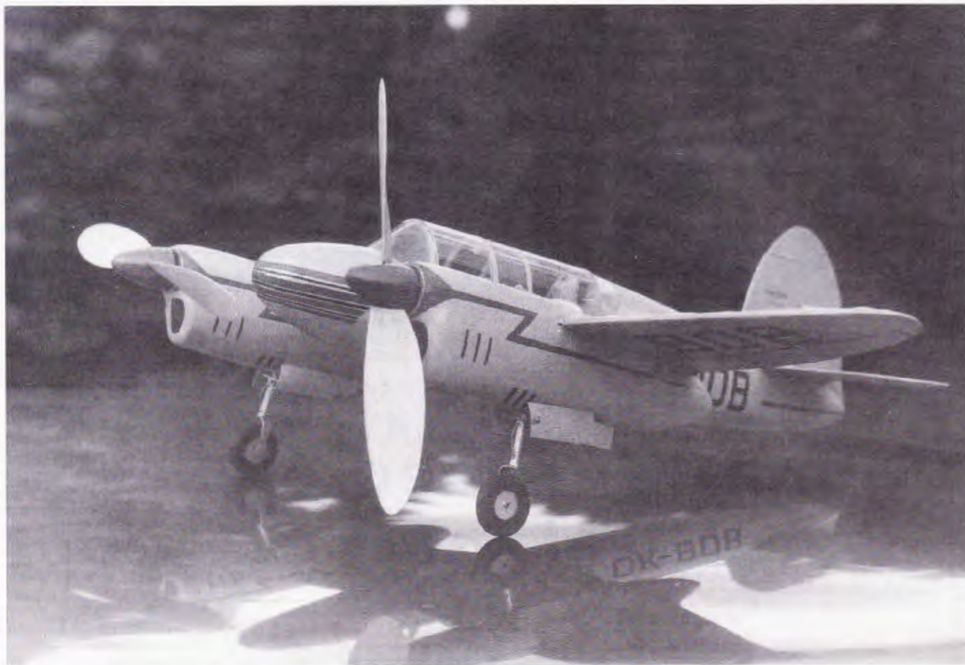
The author cuts his prop blades from \frac{3}{32} sheet balsa, and sands the airfoil shapes in. A bamboo dowel is embedded for strength.
