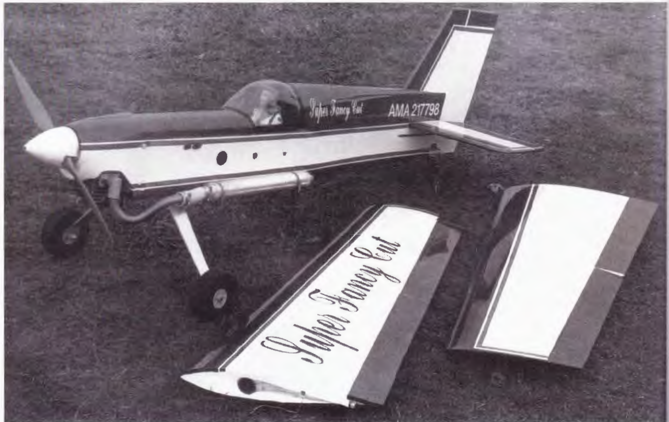
Two-piece plug-in wings make the Fancy Cut Plus very easy to transport and maintain. The pieces are easier to finish this way, too!
