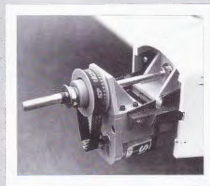
With the help of a pair of Carl Goldberg mounts, the H-1000 belt drive is easily radially mounted to the Cloud Dancer's firewall. A $28.00 Graupner Speed 700 motor with plain bearing is shown here.
