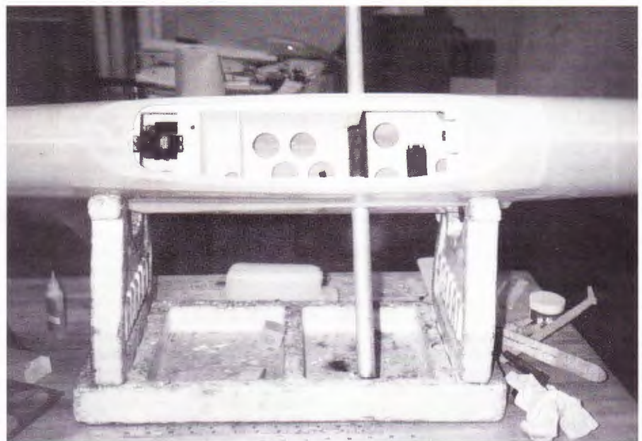
Here's a better look at the top of the crutch assembly in Dean's Malibu , the subject of last month's column. The servos nestle neatly into this plate and will never shift or loosen from stress and vibration.
