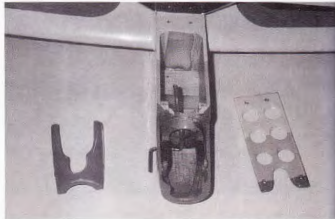
be powered by a muffled .35 engine. A simple, functional and serviceable front end treatment (above right). Note the cooling holes in the tank hatch. Smart
