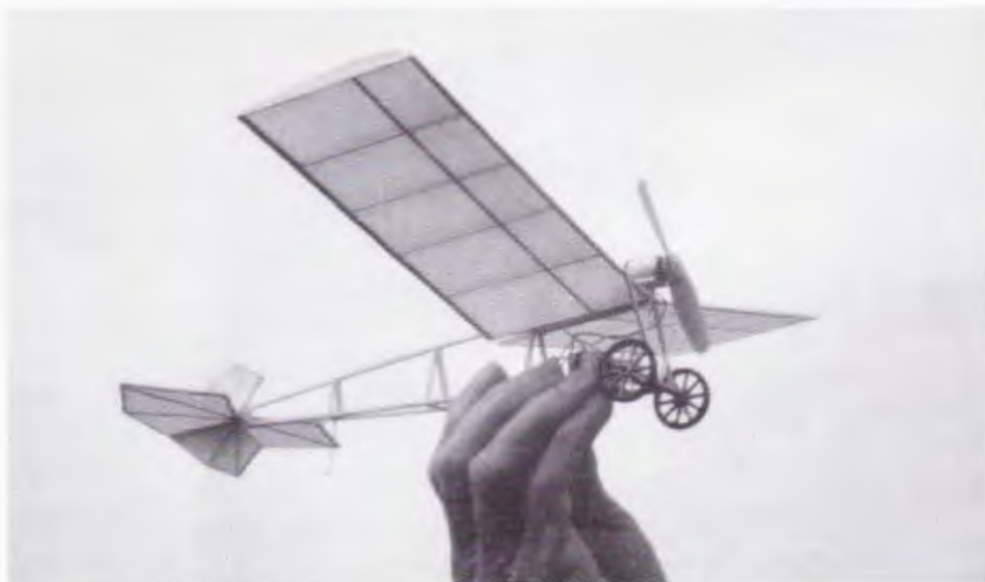
Tom Seum's 46 square inch Demoiselle , built from 3D drawings, uses a Kenway KR-1 and a 2-cell 50 mAh battery pack. These minimal material designs are naturals for electric freeflight treatment.
