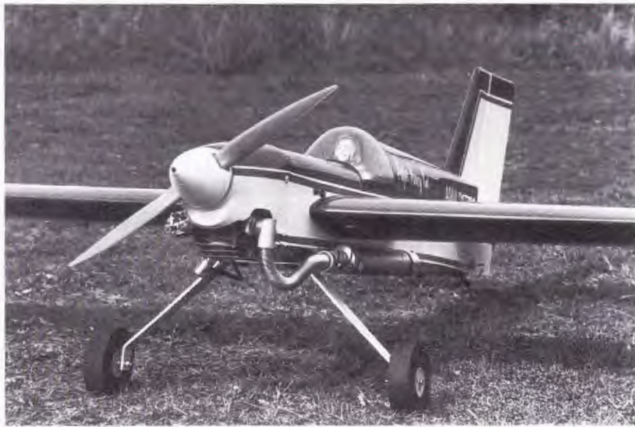
The Davis muffler and the APC prop combine to keep this big bird extremely quiet and neighbor friendly! This photo also shows to good effect the very robust aluminum gear. Wheelpants would help dress it up.
