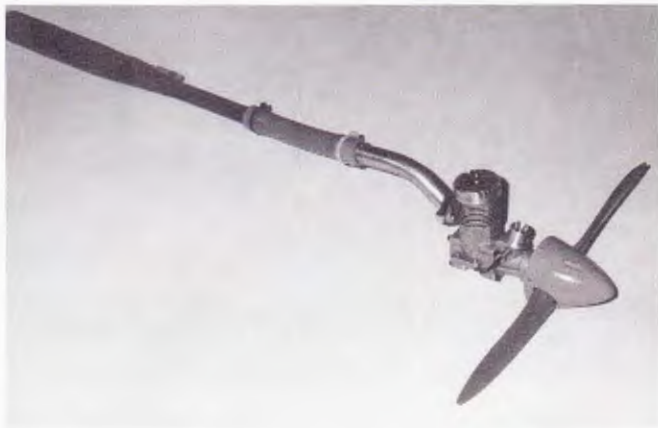
The potent power system for the Eliminator is this OS .25 VF (rear exhaust) engine coupled to a carbon fiber tuned pipe (above left). The model can also
