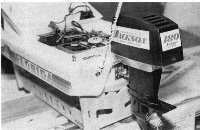
The servos and other radio gear mount in molded foam pockets (above). The antenna support mounts to the transom and the antenna is wound around it (below).
