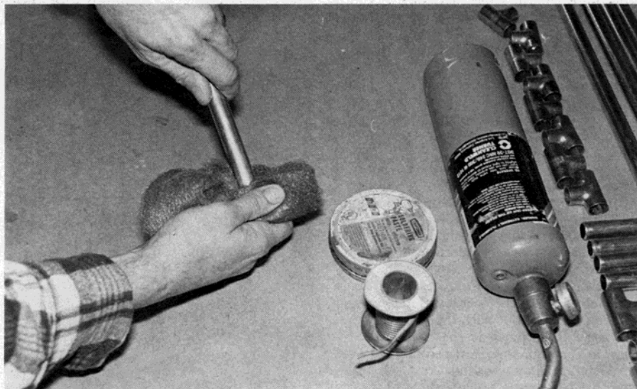
First lesson learned in "soldering school" is clean and bright. No amount of heat or flux will give a good strong joint unless you thoroughly clean all grease, oil, or oxide off parts to be soldered.
