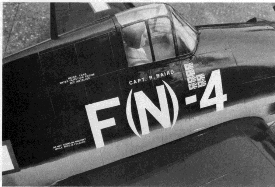
The graphics shown above were a combination of techniques. Large squadron marking was masked and sprayed; the small lettering was from dry transfer sheets; and, the Japanese flags from the kit decals.
