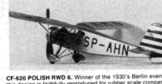
CF-620 POLISH RWD 6. Winner of the 1930's Berlin event, this design is faithfully reproduced for rubber scale competition events. Features include a 32 1/2 inch span with 150 square inches of area. By Hurst Bowers. FM 1-83. $5.00
