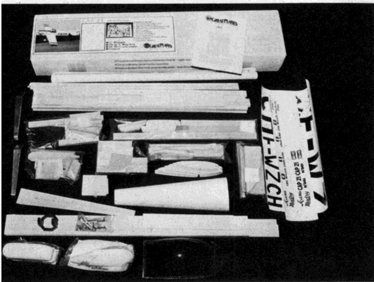
Complete Great Planes CAP-21 kit (catalog No. CP-60) is all balsa construction (above) and includes most hardware. The fuselage being framed up on the building board (below). "C" clamp joins tail tail post while glue sets.
