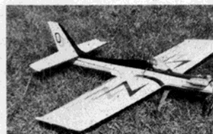
CF-625 ROOKIE. This C/L stunter features an upright mounted motor in a profile fuselage design. The ship features a 60 inch span. By Don Winfree. FM 3-83. $6.00
