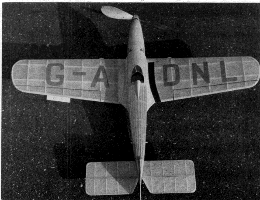
The Sparrowhawk's planform is perfect for rubber power. Ample wing and stabilizer area assure rewarding and enduring flights. The secret is all in the trimming. Do it methodically, one change at a time.
