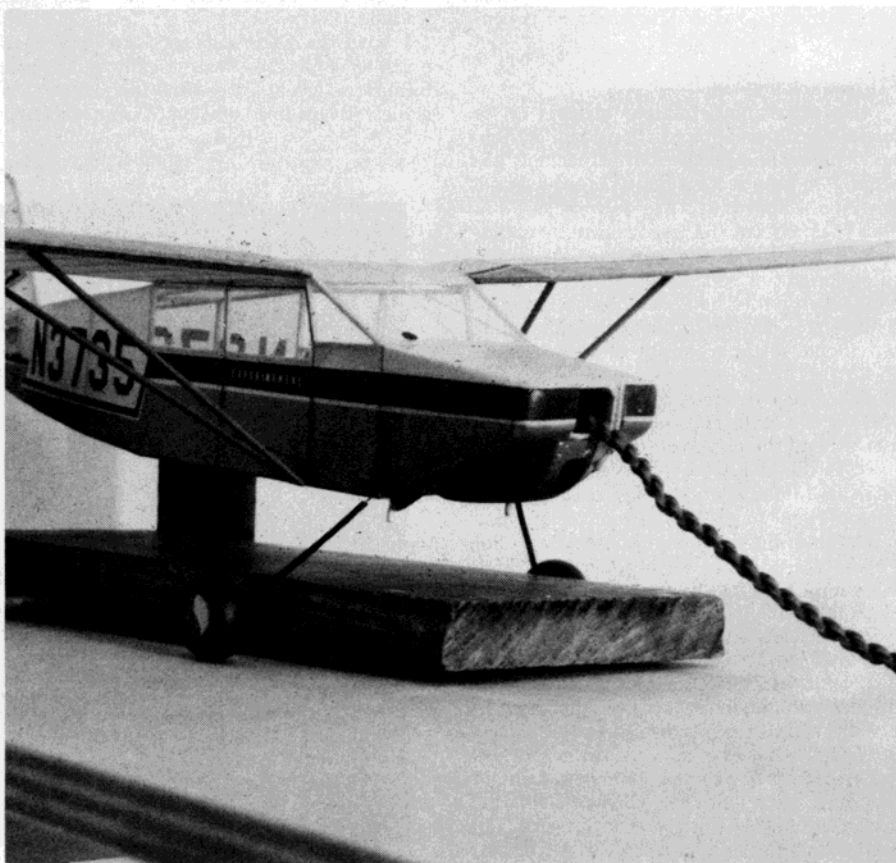
This is not a true braiding process but the pretensioning described here sure looks like it. The method works only on motors with an even number of strands, four strands or more.
