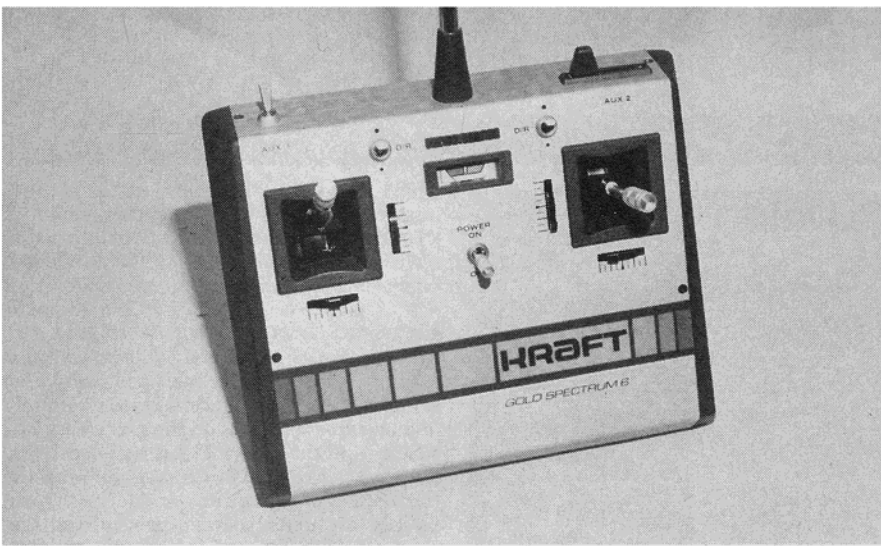
The Gold Spectrum KPT-6c transmitters styling is influenced by the European look (above). The front and rear covers are made from a gold anodized aluminum. The antenna can be stored in a tube in the bottom of the case (right). There is enough of a friction fit to prevent the antenna from accidentally sliding out of the storage tube. The transmitter side pieces are a dark brown high impact plastic.
