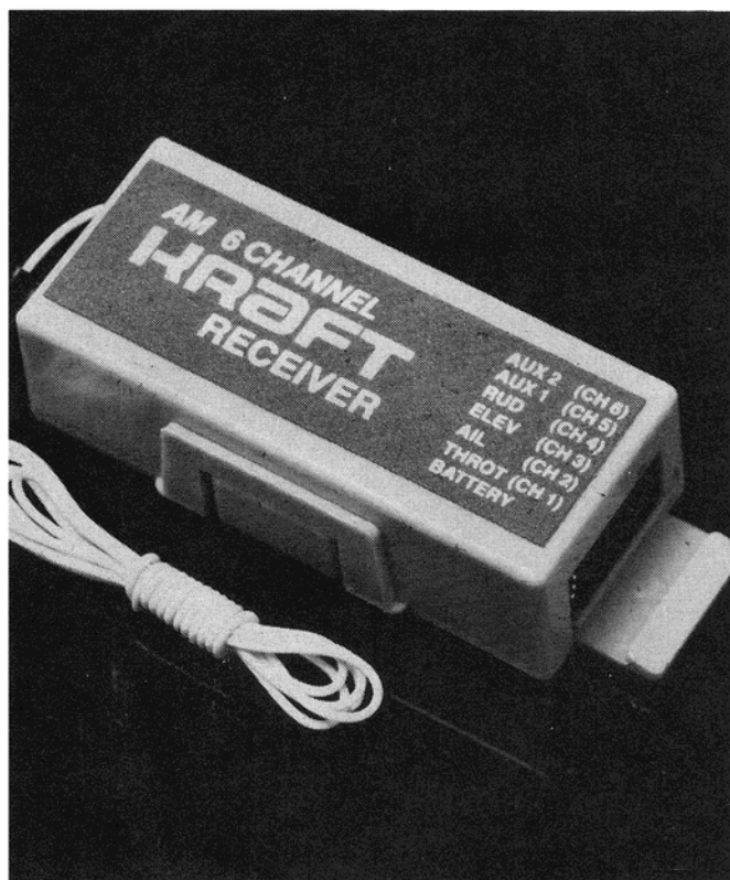
This is a close-up shot of the new KPR-6c Gold Spectrum-6 six channel receiver (left). The decal contains the channel function callouts, which is a great convenience. This is the connector block end of the receiver (above). The connectors are the popular Kraft Multicons. Standard wiring!
