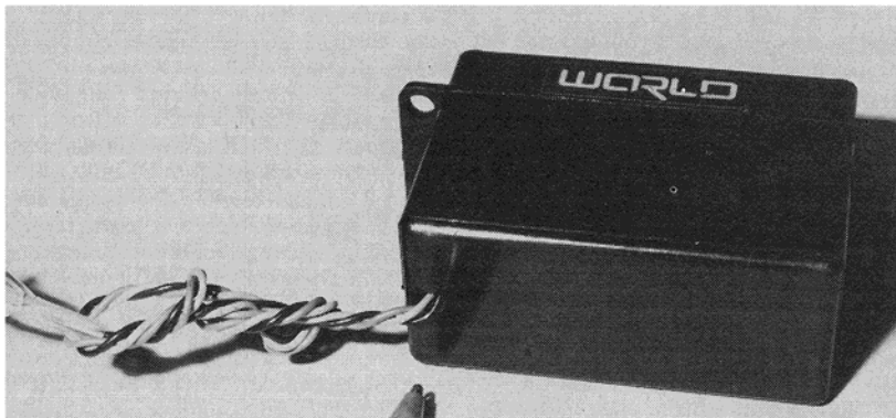
The S-12C (shown here) and the S-11 servos have their cable exit out the bottom of the case. Bob likes this feature because it doesn't let the cable get in the way of the tray or beam mounting.
