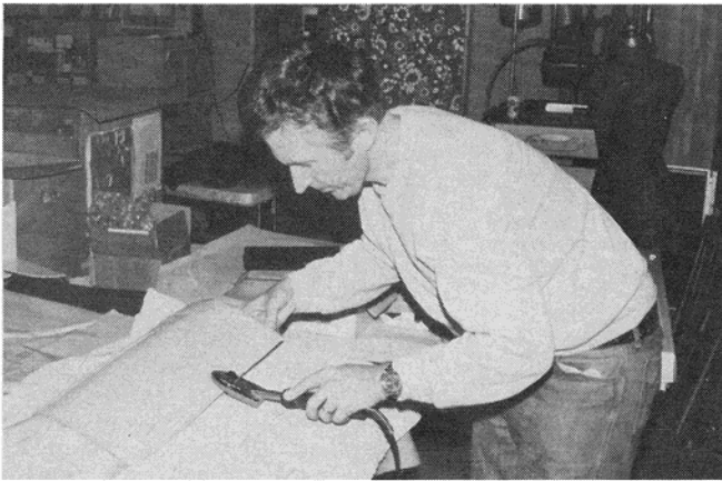
Bob stresses that \frac{1}{16} " vertical grain balsa webbing must be added between every rib station at the main spar and at the beginning of the trailing edge sheeting (above). Bob is shown here ironing Top Flite's Super Monokote onto a wing panel (left). It's the light way to go.
