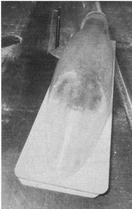
The cowl is glued to a piece of \frac{1}{16} " plywood and then another piece of \frac{1}{16} " plywood is glued to the bottom to form a lip (above left). "L" brackets allow the rear sponsons to be adjusted (above right). The motor mounts are shown here (below). Note the corner bracing. Holes in mounts aid gluing (below right).
