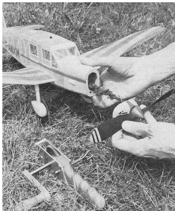
The powerplant of the Caudron is shown here. Notice the braided motor which keeps the rubber from bunching at either the nose or tail and upsetting the trim. The nylon bobbin prevents rubber stress at the prop hook. The 10 to 1 winder is a must for winding such big motors.
