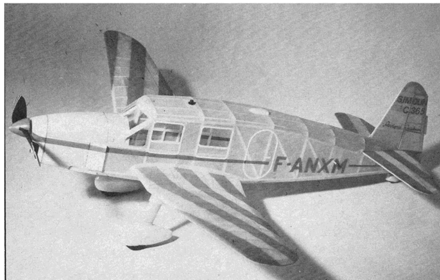
The sheeting and hollowed blocks at the nose distribute the stresses to the rest of the airframe (top). Tissue covering on acetate windows gives a realistic appearance (above).
