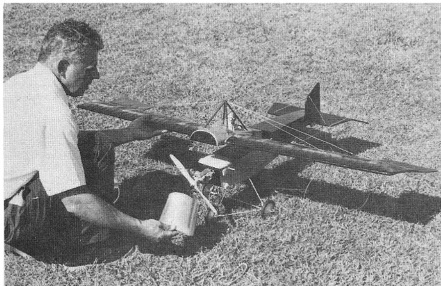
The radio compartment is well designed and spacious. The Enya .35 can be seen here. Al chose to use dowels for the wing hold down as there was no solid bolt anchor available. The tail feathers with their flying wires attached ( top ). Note the placement of the Nyrod pushrods, skid and control horns. Al removes the wing and cowling for access to the radio compartment ( below ).
