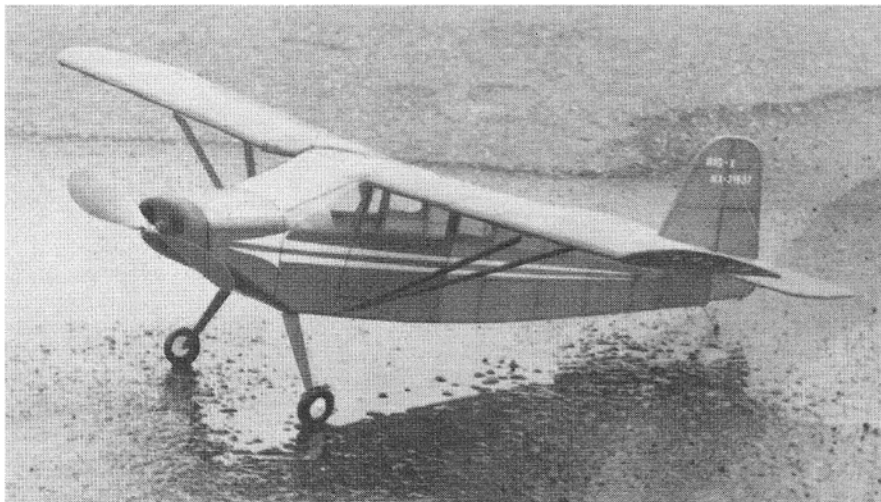
The long landing gear assure prop clearance for those long prototype takeoffs. The Big X climbs out for another long flight (top). The author reports good stability and glide characteristics. Try one soon.
