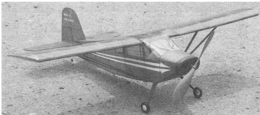
The long landing gear assure prop clearance for those long prototype takeoffs. The Big X climbs out for another long flight (top). The author reports good stability and glide characteristics. Try one soon.
