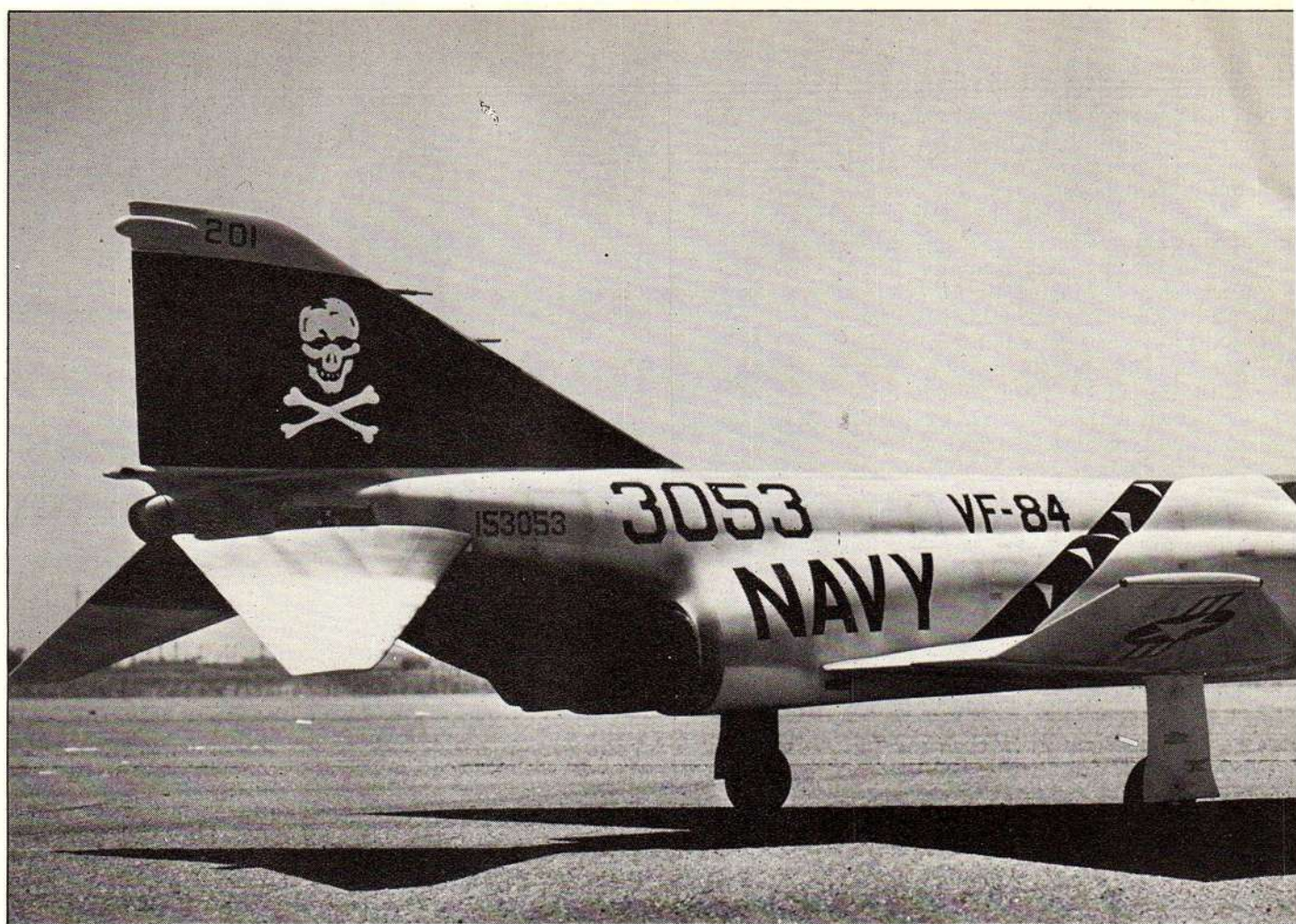
The F-4B is just a large glass-and-foam kit, comparable to any Pattern ship, according to the author. The fuse is over seven feet long, and comes in one piece!
