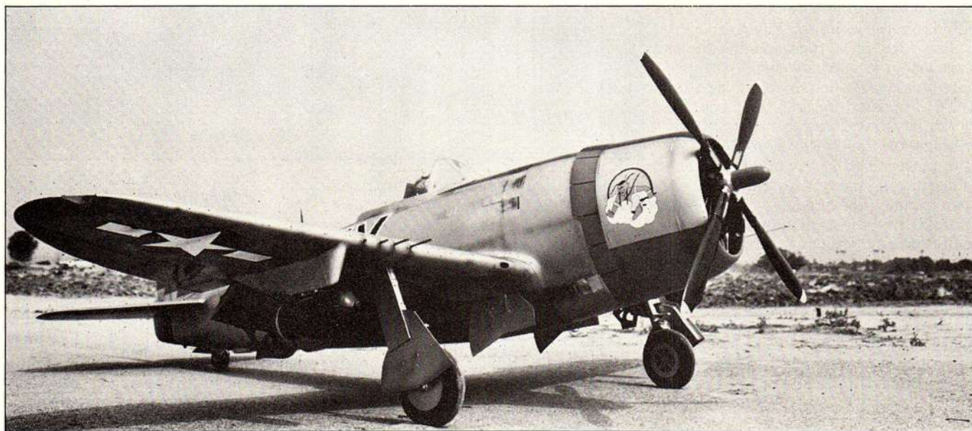
Shane's Thunderbolt was repaired several times, and finally wound up weighing 25 pounds, but it still flies well on a .90.
