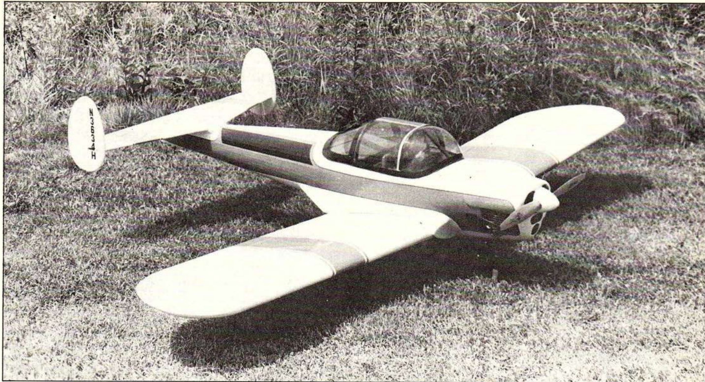
Chris Dascano's Ercoupe was built from a kit. The 92" span ship uses a Quadra for power.
