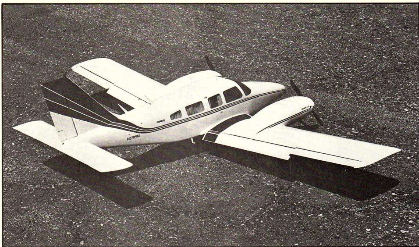
The Seneca is a huge model, with an 85" span. Two .40s flew it easily at half throttle.
