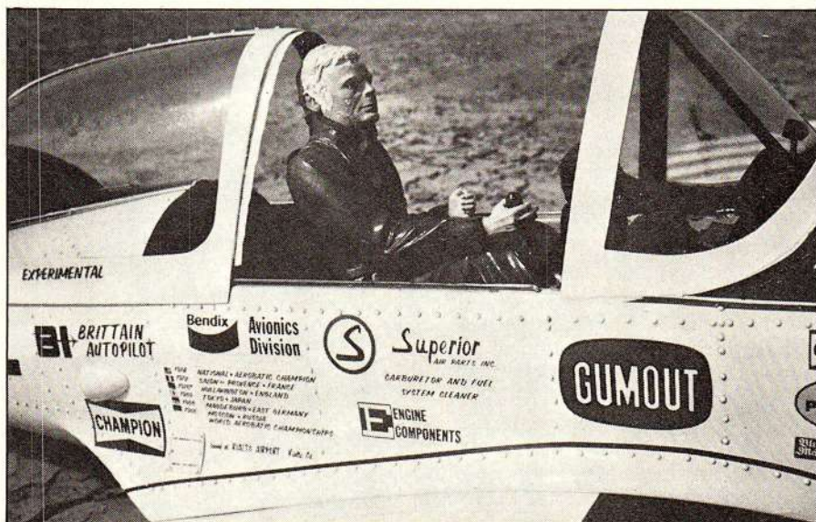
John Bashore really loaded down the model with scale detailing. Even the canopy slides, yet the model just weighs slightly over 20 pounds.
