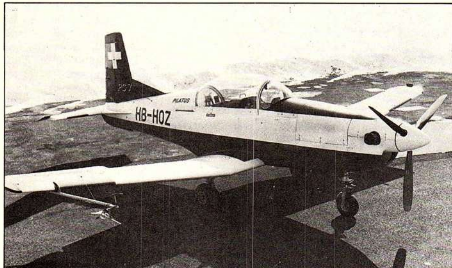
Civilian versions have a clear bubble canopy, while military ones have a reinforced cage.
