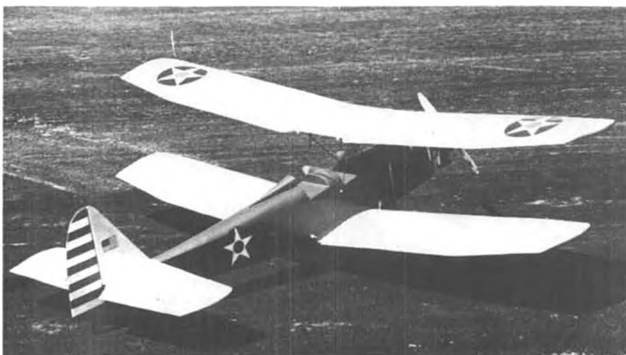
Duane Thomas' high altitude Bi-Prentice. OS Gold Head 60 power and MRC 3-channel radio. Wing span increased to make up for the thinner air in Colorado Springs. Photo by J. A. de Vries.
