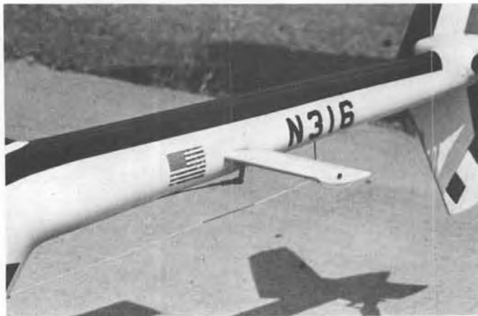
Ernie Huber's Kavan Jet Ranger with a Mike Bosch elevator rig for looping. It ties into "reverse" cyclic.
