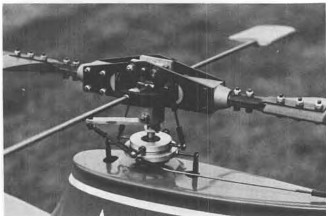
Here's John's Huey Cobra with the Schluter "Expert" collective pitch head. Described in text.
