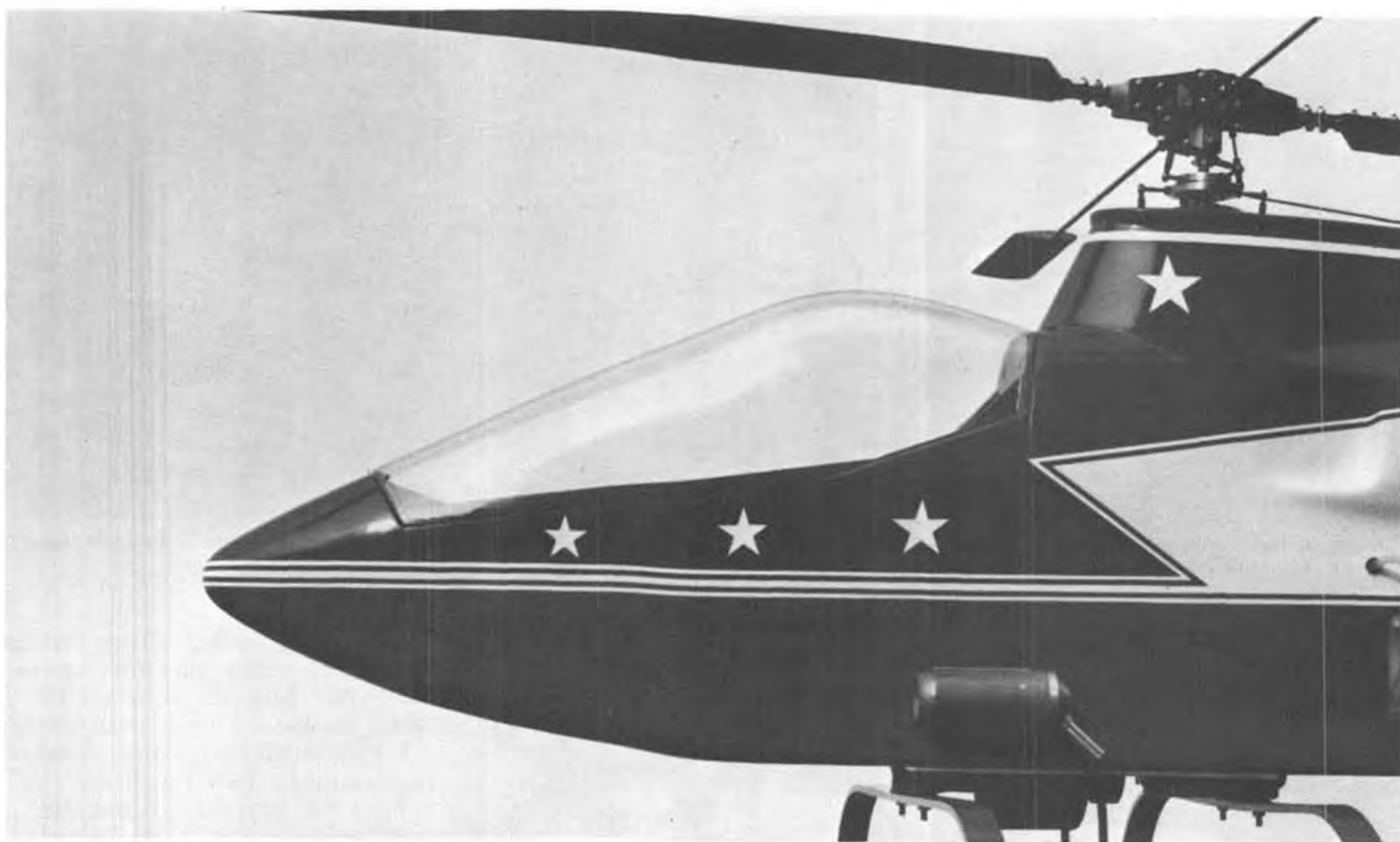
The "New Look" on John Tucker's latest Heli Bell Huey Cobra was obtained by turning the stock canopy around! Not a bad looking arrangement. Modification required a triangular gusset to fill in a gap at the aft end.
