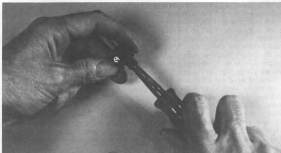
Use a tapered reamer to reduce losses and increase pressure at the crankshaft inlet port.
