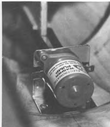
Reversible electric windshield washer pump operates bow thrusters.
