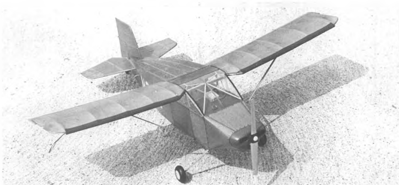
Tom Stark's Tailwind rubber powered model won first in outdoor scale at the 1974 Nationals. Only deviations from true scale are slightly increased dihedral and stabilizer area. The flight times averaged over a minute for four flights.
