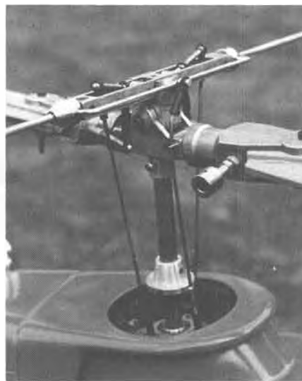
"Third arm" conversion for Kavan Jet Ranger, as explained in text.
