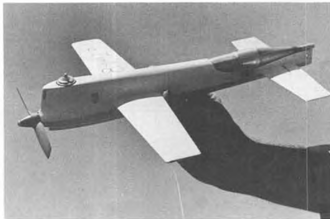
Record holder all buttoned up and ready to go. Note left-hand prop and Mono-Line lead-out, also, last-minute AMA numbers!
