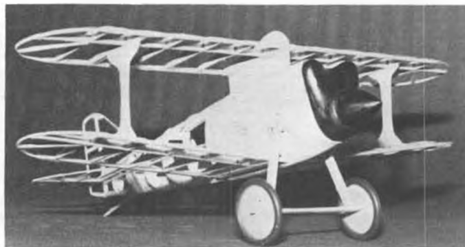
Joe Bickinella's 9-1/2" span (1/2" scale) 1922 Curtiss R-6 Pulitzer Trophy Race winner. Surface outlines are 1/20 bamboo.
