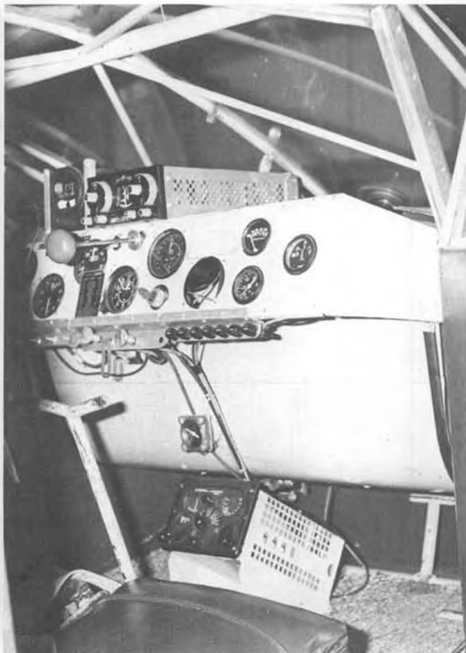
Instrument panel is light gray. The stick is centrally located and can be used from either seat.
