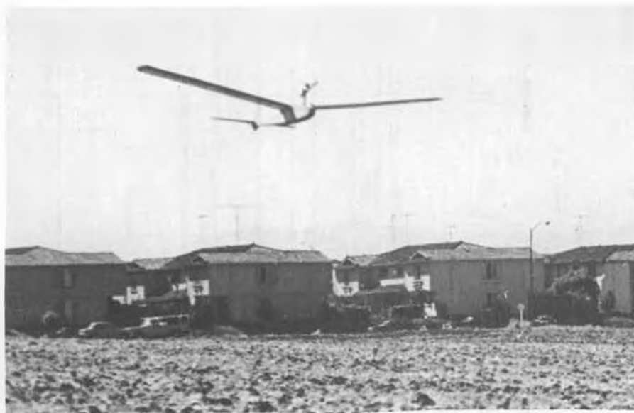
Coming in after another powered, but silent, flight. For powerless thermal or slope soaring, the power pod/hatch is replaced by a plain, flat panel. Extra ballast will then be needed.
