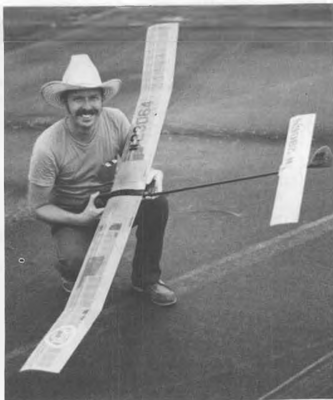
Mike Ransom, Dallas, with his Texas-style Nordic. Monokoted wing, sheet T.E., British style fin, glasrod boom. Linstrum photo, '74 Nats.
