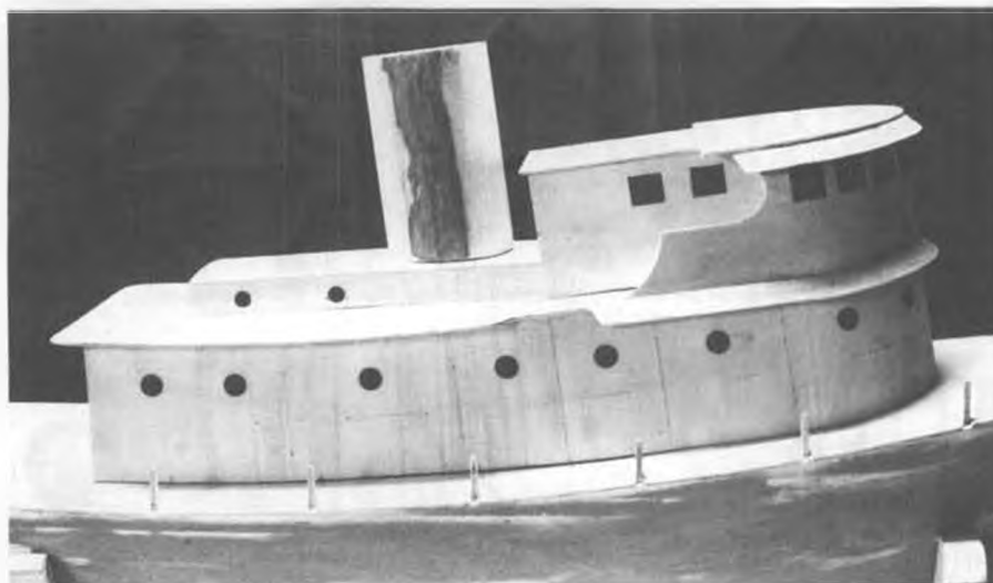
Completed cabin structure, resting on deck. It fits over deck opening rim, and serves as a quick-opening lid to the radio and running gear in the hull.
