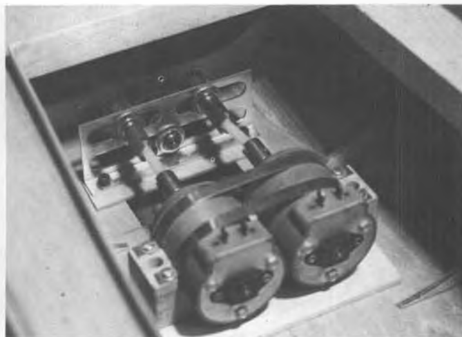
Another drive system consisting of two Dumas motors with a Dumas 3-1/2 to 1 gear reduction. Note universal couplings.
