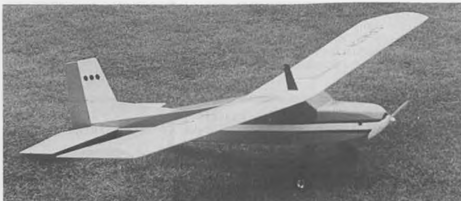
The Camion, an all-purpose model designed and built by Thomas Lewin. Uses a Keller 50/24 motor with 21 1.2 ah cells. Drops candy bon bons, also used for glider towing.
