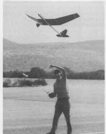
Going up on the line. Light weight and large wing area make for high launches.
