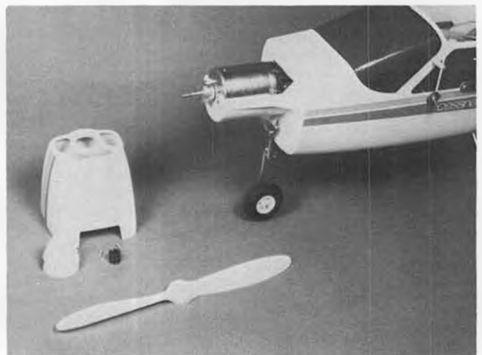
Motor is fastened to a plastic mount that also holds the nose gear. Two screws hold plastic cowl in place. Top Flite BX4 prop.
