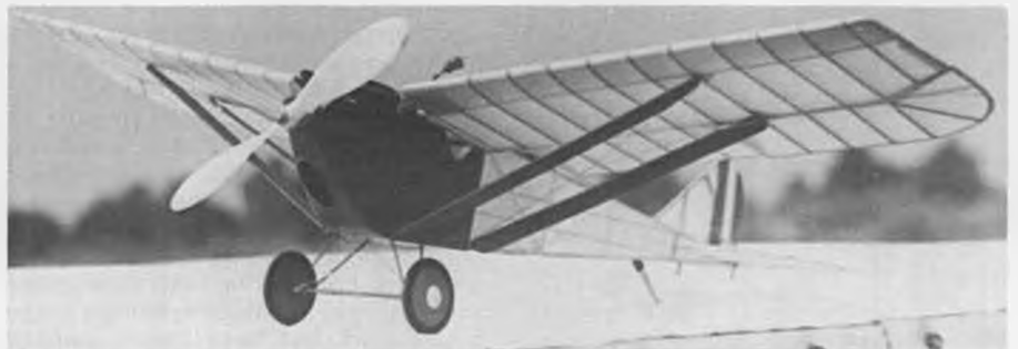
Nick's Loening has all the right proportions for a scale F/F model. Dihedral has obviously been increased over that of the full-size aircraft. Note separate ailerons for flight trim.
