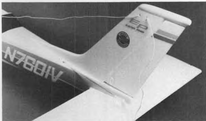
Fin extension over rudder is prone to breaking, text tells how to cure this. Stab is held in place by friction and a plastic screw.
