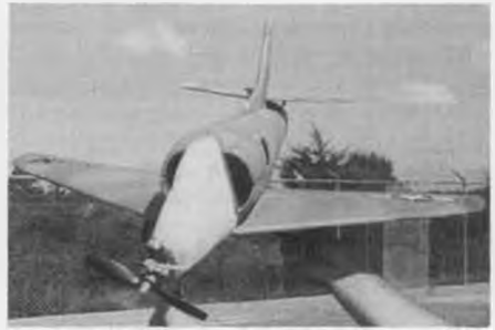
FIG. 22. The A4D fitted with a nose-mounted TD .049 prop engine.
