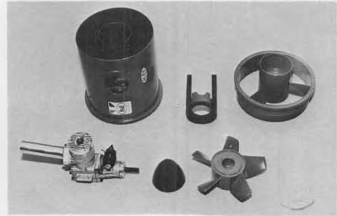
FIGS. 23 (left) and 24. Before and after assembly photos of the RK-20 fan unit designed for .20 size engines. Midwest Products has the unit on the market now, called the RK-20B.
