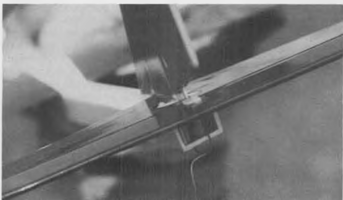
Ken has all the horns and linkages mounted internally to cut down on drag, yet are easily accessible for adjustments.
