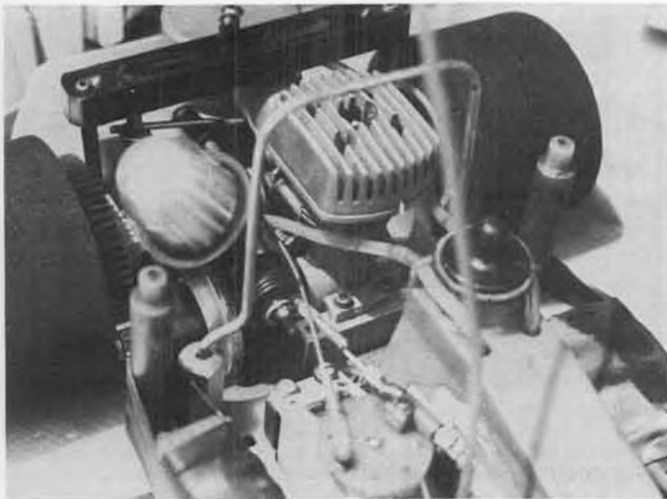
OPS engine and new slide valve carb on Bervoets' car, with wet-weather air cleaner and Delta type fuel tank filler.
