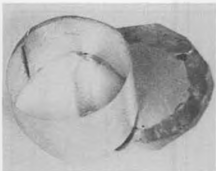
Fuel tank space is limited, so a special tank is needed. This one is reminiscent of the old deBolt "clank" tank. The fuel pickup tube is weighted (see middle photo) and can swivel a full 360°, ensuring good fuel draw regardless of the model's attitude.
