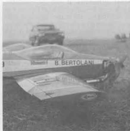
Clever and very precise trimmable aileron tip used by Benito Bertolani on his Komet.
