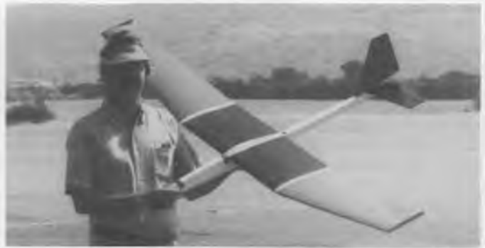
Ken's bird uses a flat center section wing and 8% thick airfoil. Fuselage is open on top and bottom, covered with Monokote.
