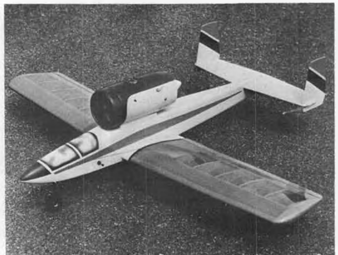
The Jetster 20 by Midwest Products, specially designed for the Axiflo RK-20B fan unit.
