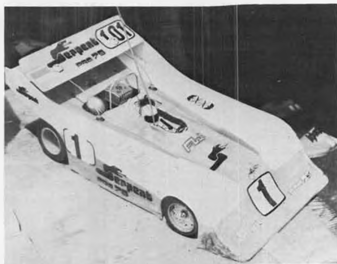
Pieter Bervoets' Serpent car. Wing is mounted farther forward than on most cars, is supposed to help car handling.
