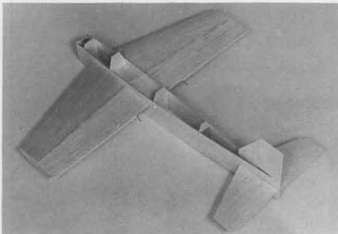
The assembled basic framework. Note that the wing i.e. inside the fuselage is cut away to make room for the R/C gear.
