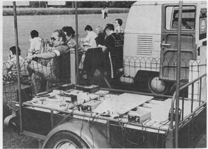
Charging station at Benelux meet uses 1800 ah truck batteries and Graupner chargers, can charge up to 18 volts from a 12-volt battery.
