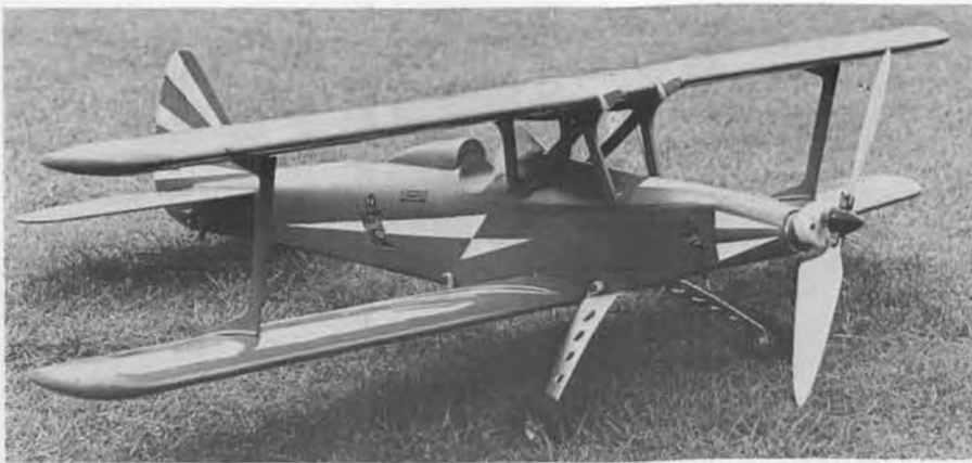
Fritz Geist, maker of the excellent Geist motors, built this Wayfarer a Don Dewey/RCM design). Uses a Geist type 126 motor, geared to a folding prop.
