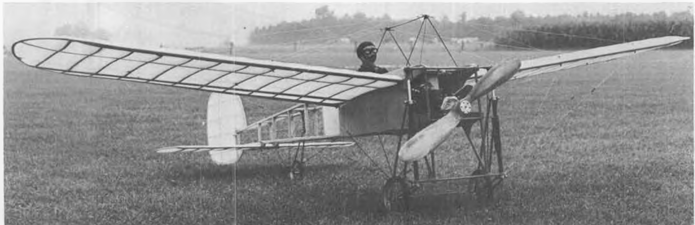
Realistic looking Bleriot by R. Diederich was flown at Benelux Electro Meeting. Spans 67 inches, weighs 102 oz., uses a Carrera motor. Flight performance is only so-so, as there's too much drag with all those wires.
