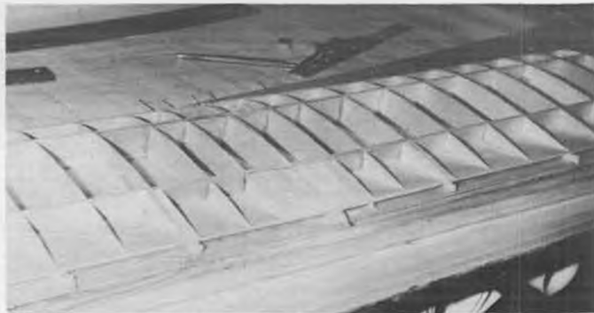
Spars and ribs are notched egg-crate fashion for easy, strong assembly. Finished framework is sheeted with 1/16 balsa.
