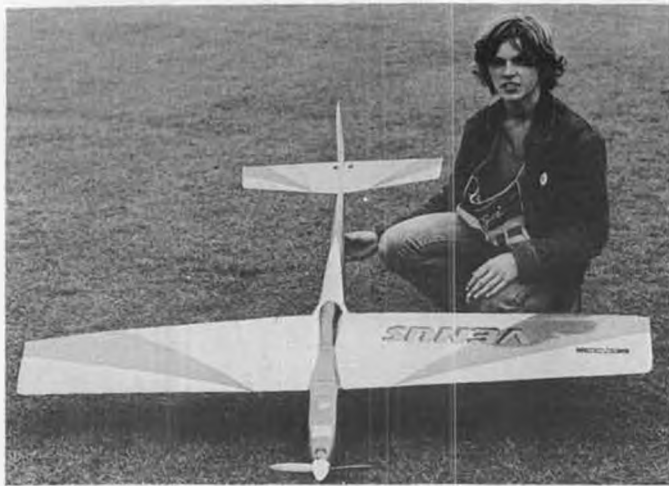
Dennis Kuhn, 17, Pattern winner at Benelux Electro Meeting. Model weighs 7-1/2 lbs., uses Keller 50/24 motor and 24 1.2 ah cells.
