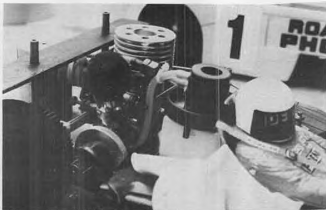
Engine, carb, and fuel tank set-up on the Phoenix car. Note small metal carb (like Veco .19).
