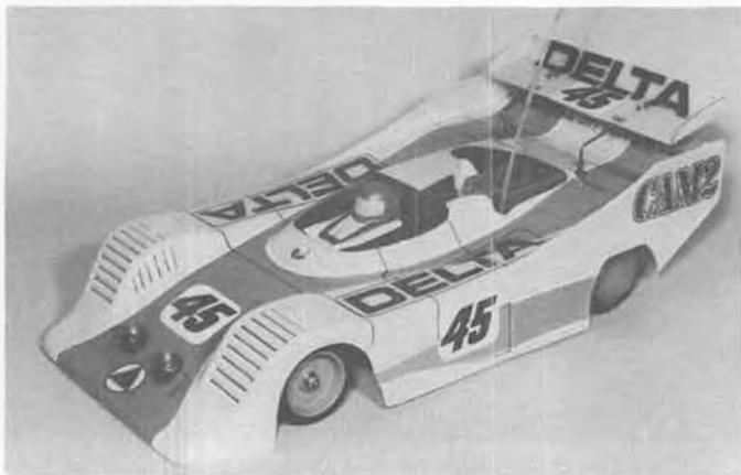
The Delta Super J chassis wrapped in MRP's TOJ-BMW Can-Am body. Standard Dirty racing colors, orange and yellow.
