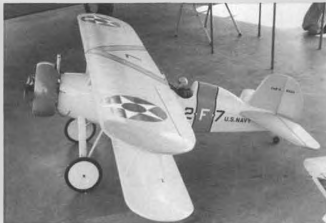
In contrast to the big F4B3 is Nate Rambo's 1/4-scale F4B4. Basically the same airplane but with bigger fin, other minor details.
