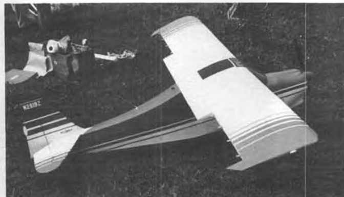
. . . aileron flutter did this. Luckily, both ailerons came off clean and Cliff made an uneventful landing with just rudder control.
