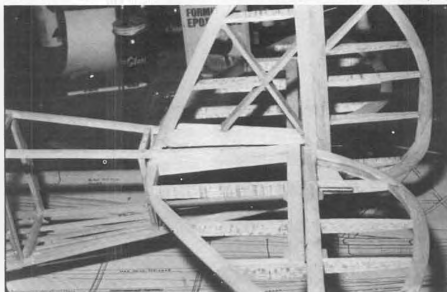
Tail surfaces are built from 3/8 balsa, sanded to a streamlined cross-section. Outlines could also be laminated out of 1/16 thick strips for higher strength at no increase in weight.
