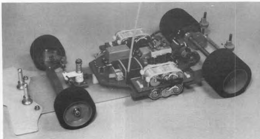
Electric cars in 1/8 scale are available, even though not widely publicized. This 12-cell model is from Delta, is basically a converted Super J with Astro 15 motor. Very smooth running.
