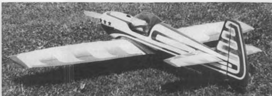
The Higgins Aero Composites CAP 20L, built entirely of epoxyglass shells with urethane foam cores. At a weight of less than 20 lbs., it's agile with a Quadra. Three flew in the meet.
