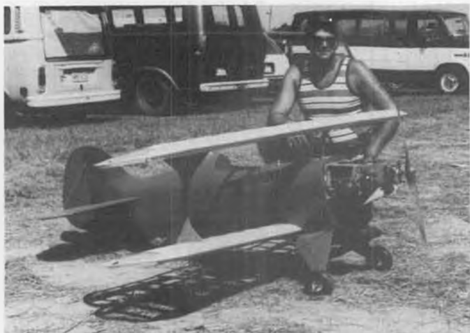
Two scratch-built Pitts by Dave Landvater, Elizabethtown, Pa. The S-1 on left has 2 Quadras in tandem and Eastcraft starter, weighs 30 lbs. The one at right is single Quadra powered. Both seen at DC/RC Scale Meet & Air Show, Flying Circus Aerodrome, Bealeton, Va. Droegge photos.
