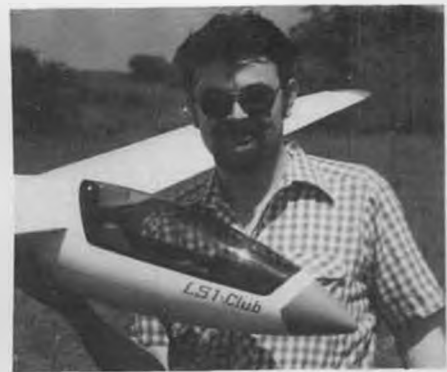
Here's Herb Wanitschek himself, holding one of his larger scale sailplanes, the LS-1 Club (147-1/2 inch span). Note the UHF antenna dangling from the fuselage.
