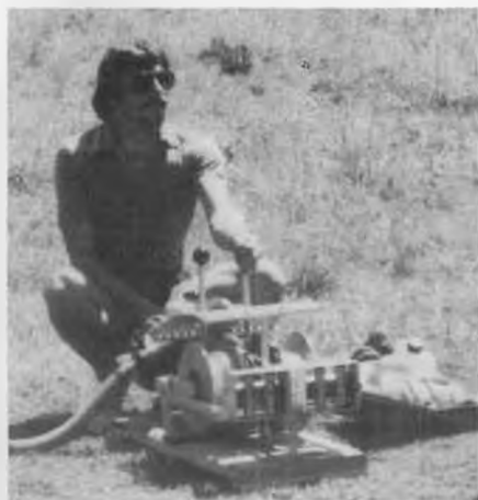
Our roving columnist spotted this gasoline-driven winch at a contest in Switzerland. It's equipped with a line return reel that brings the parachute back to the winch after release from the model.
