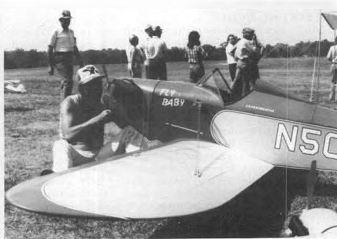
The spread between aircraft and model narrows. Gary Ingraham, Roanoke, Va., powers his Mitchell Wing B-10 with a 12 HP McCulloch engine. On the right, Walt Moucha, New York, services the 3 cu. in. Roper in his 1/2-scale Fly Baby. Both seen at Bealeton, Va. Photos by Bob Droege.
