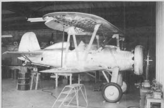
Indicative of the projects you'll find in Santa Paula's hangars is this incredible scratch-built Boeing F4B3, being constructed by Jim Dewey. Should be flying within a year.
