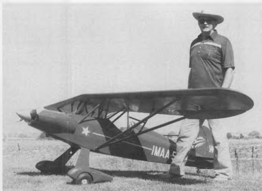
Wally Rinker doesn't quite manage to dwarf his 1/2-scale Stolp Starlet, said to be a magnificent flier with its 6 cu. in. Husqvarna (motorcycle?) engine. Spans 13 feet, weighs 57 lbs.
