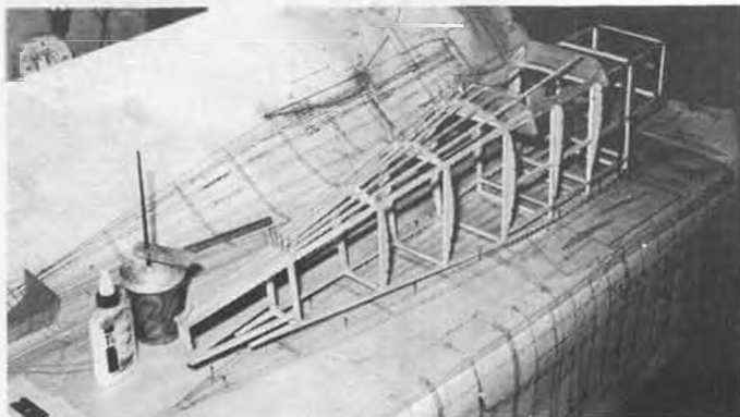
Basic fuselage structure is a simple 3/16 sq. box, with formers and mucho stringers to give the nicely rounded cross-section.
