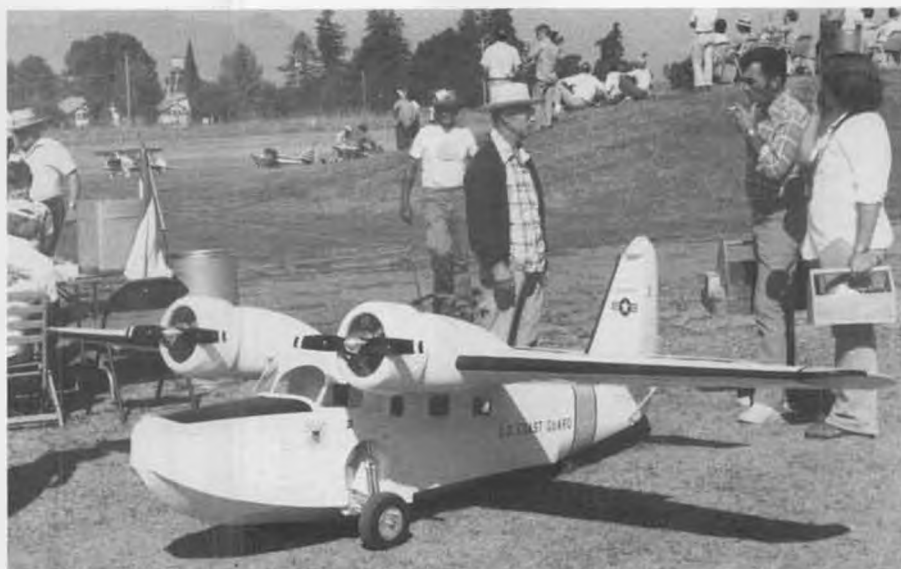
Dick Hershey, in straw hat, discusses his almost-finished Grumman Goose project with spectators. This monster spans 13-1/2 feet, weighs over 120 lbs., and is fitted with two Roper 3.7's.
