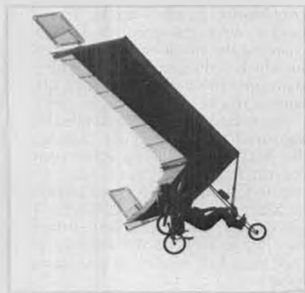
Powered hang gliders were given their chance to perform also. This particular one is a Pterodactyl Fledgling, powered by a 440cc Xenoah snowmobile engine.
