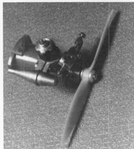
G-Mark's .03 is the smallest available powerplant equipped with a working carburetor throttle. Cannon Electronics imports them.
