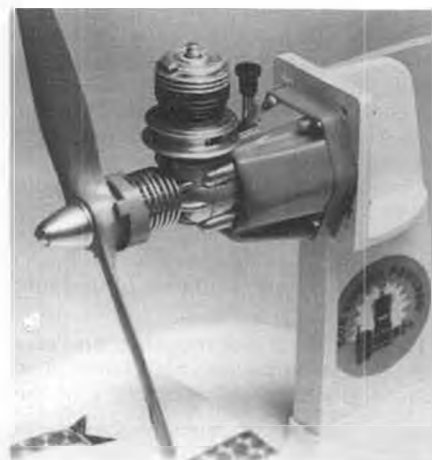
The Cox R/C Bee features an extra large capacity tank, new spring starter design, throttle, and muffler. Runs great, and the mounting holes are identical to other Cox engines.
