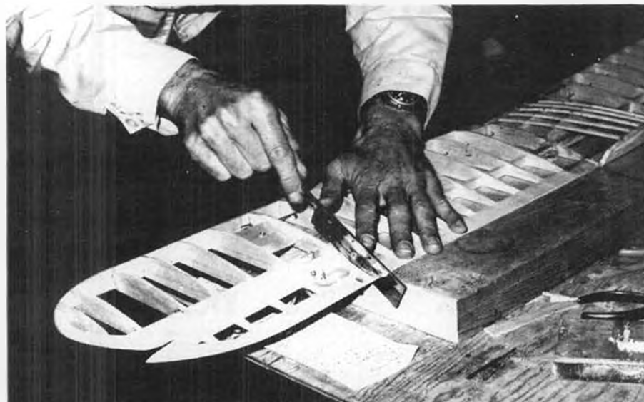
Ailerons are built as part of the wing structure, then carefully cut loose after the pushrods, bellcranks, horns, etc. have been installed. The last step before preparing the wing for covering.
