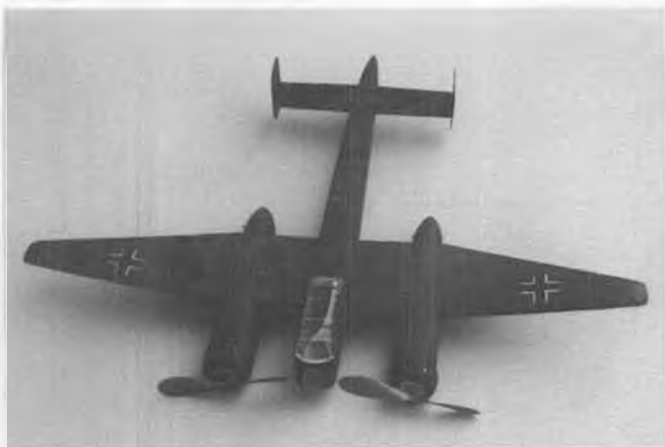
Another off-the-beaten-track model is this Arado 240-A light German bomber by Fernando Ramos. Rubber motors are enclosed in the 12-inch nacelles. Best flight time to date: 26 secs. Fernando plans to build another, lighter version in the near future.
