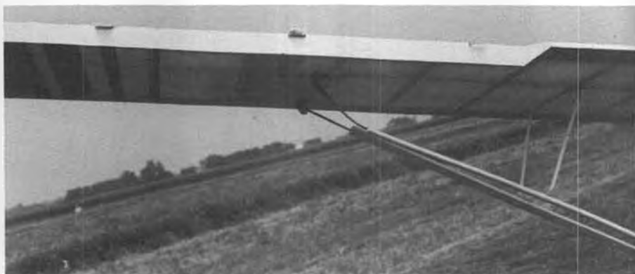
Here's what the aileron flutter did to the wing struts on Tacie's high-powered Citabria. Hinges had been pinned with straight pins, but they pulled right out.
