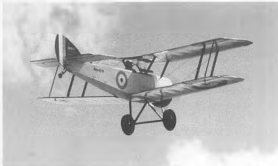
With all that wing, Ken's Pup is a real floater even at an all-up weight of 32 lbs. Prop blades barely stick out beyond the 13-1/2 inch diameter cowl.
