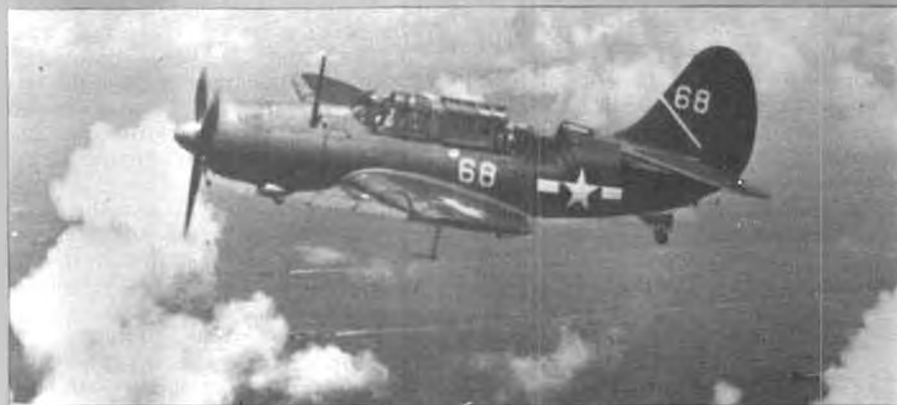
Final version of the famous Helldiver was the SB2C, direct descendant of the old F12C-1. A total of 7,535, including 900 A-25A's, were built in WW-II. Photo courtesy Ed Young.
