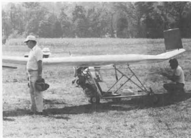
The spread between aircraft and model narrows. Gary Ingraham, Roanoke, Va., powers his Mitchell Wing B-10 with a 12 HP McCulloch engine. On the right, Walt Moucha, New York, services the 3 cu. in. Roper in his 1/2-scale Fly Baby. Both seen at Bealeton, Va. Photos by Bob Droege.
