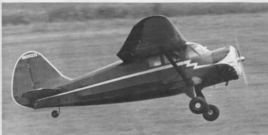
Corky Heitman's big Stinson SR-9 lifts off. Kioritz engine turned this putt-putter into a performer. Built from Barron plans, it spans 10-1/2 feet and weighs 37 lbs.
