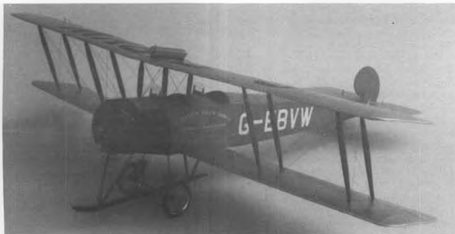
Here's the troublesome AVRO 504 that gave our columnist fits just before the F.A.C. Nats... see text for sad tale of woe. Span 36 inches, power is a D.C. Dart .035 diesel.
