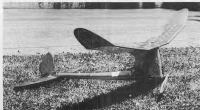
Photo No. 13. Another of Bob Knutson's experiments back in the old days was this Zomby-like design, featuring a Snuffy VI wing and tail on a dural fuselage. Bantam .19, later had folding prop!
