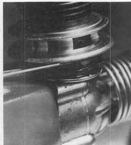
Hook-up and adjustment of the throttle are probably the easiest of any engine. A rubber muffler slips over the outside of the throttle sleeve. Idle is low and quite reliable.
