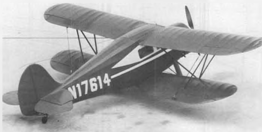
Cabin Wacos had distinctive lines when viewed from any angle. Realistic finish is good ol' silk and dope, finished with Aerogloss paints. YKS-6's were powered by 225-hp Jacobs engines.
