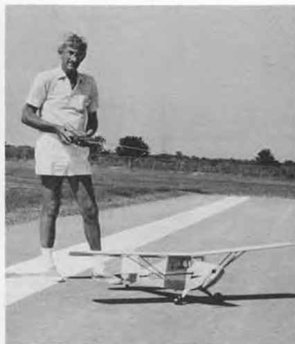
Don Siegle of Houston Sparks with his Astro Porterfield with Astro 40 cobalt motor, 20 Sanyo 800 batteries and Emco throttle.
