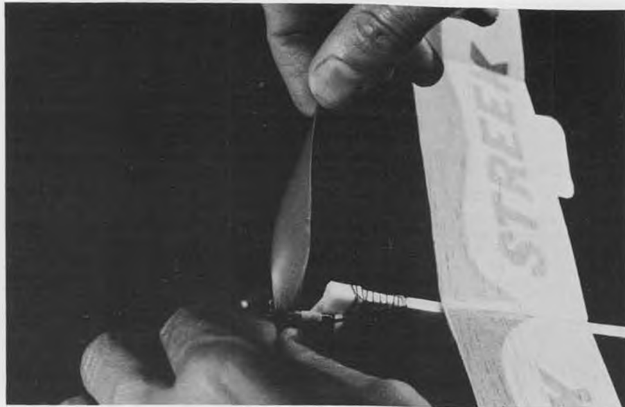
Twisting prop blades into lower pitch gives more power, but runs out the winds sooner.
