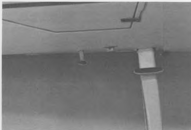
Can you find the switch? Surprise, it's the small step just below the door on this Citabria. A simple push-pull arm does the job. It's connected to an internally mounted switch.
