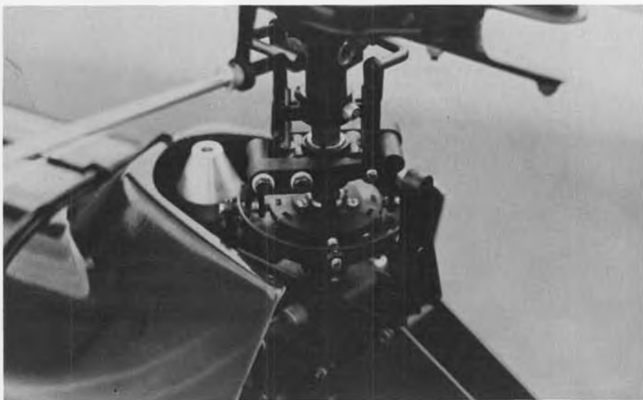
Note washout at 45-degree angle to flybar.
