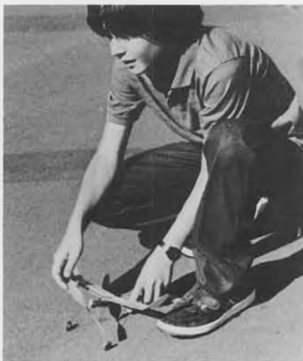
Here Kris Samonas demonstrates the proper way to launch an ROG. Aim a little to the right, facing the wind, let prop start turning, then release your plane.
