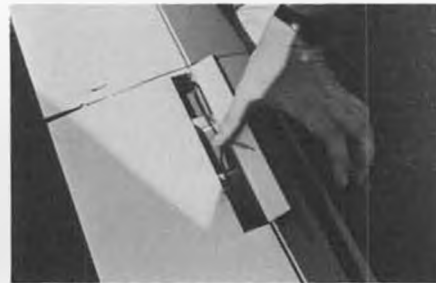
Open Spoiler bay gives access to the Image's aileron servo connector and extension cord.
