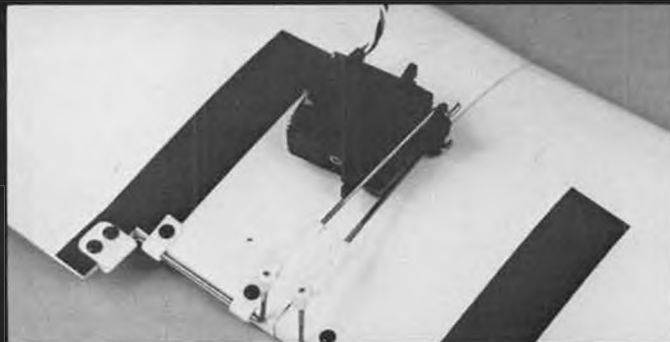
Aileron servo installation is like that on larger planes. A piece of plywood is epoxied to balsa wing covering with servo attached.
