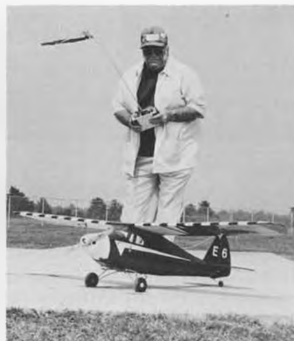
Dr. Jean Duke of Houston Sparks with Astro Porterfield powered by an Astro 40 cobalt and 18 Sanyo batteries, and Geist throttle.
