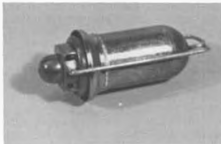
Jet-X, rocket-type jet motor of the 50s and 60s is back. Made in England by Powermax and sold by Peck-Polymers in the USA.
