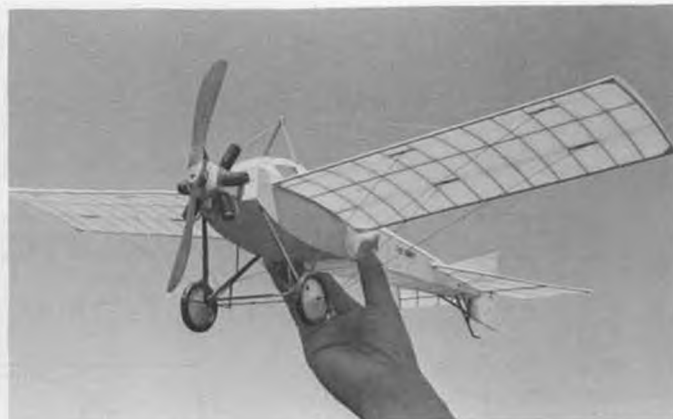
Cessna Comet by Larry Kruse was the winner of the '87 Nats Scale Gas class. Powered by a Telco CO 2 engine, the 22-inch span model weighs in at a trifling 59 grams.
