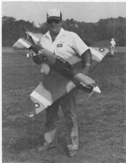
Dick Watz got to show off the new Hurricane MK 11C from Aerodrome Models at the Four-Stroke Rally. A nice performer, not too big at 62 inches, it flew up a storm on its Saito .80 four-stroke engine.
