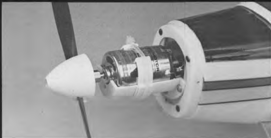
A LeMans AP-29 handles things in the power department, and is furnished complete with a 6-volt 450 mil Ni-Cd battery and a 12-volt input timer-operated fast charger.
