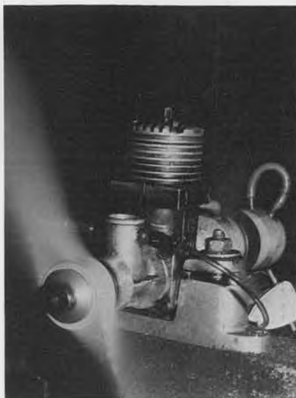
Engine was running in 15 seconds on the test stand. Raising/lowering the fuel tank made no rpm difference.
