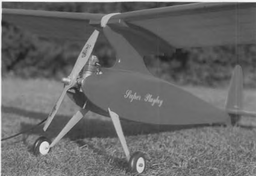
With a wingspan of more than nine feet, the nine-pound weight of the Super Playboy was relatively inconsequential. With care, it can be built much lighter without sacrificing strength.
