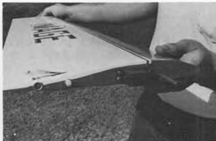
Aileron servo for the Image mounts to the root rib of the tip panel.
