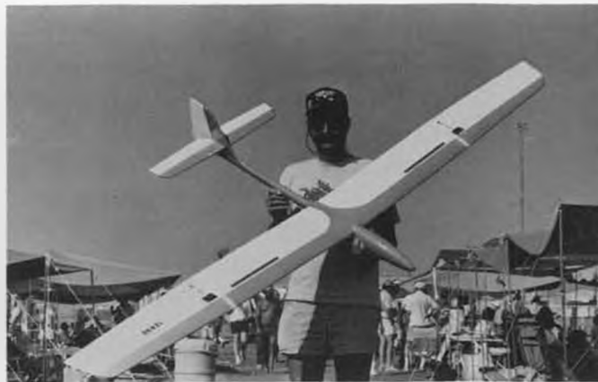
Mike Walter and his modified Cumic. Had trouble with servo tape letting go inside wingtips. Note square holes.
