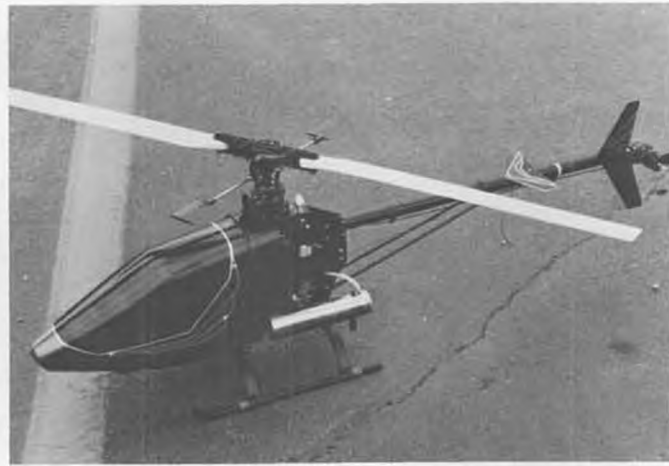
Schluter Junior 50. Note difference in tank location and start shaft.
