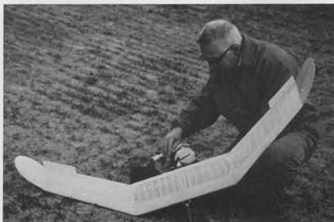
Bill Darkow readies an unusual Nostalgia Ship, the Wing Ding by Hank Cole, from an issue of Flying Models. Ship is powered by a Cox Baby Bee. Bill claims ship flies better with balsa ailerons. Photo: Stalick.
