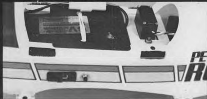
The removable canopy gives access to the flight battery for charging. Elevator servo also shown. Pushbutton switch starts the motor independent of the radio.
