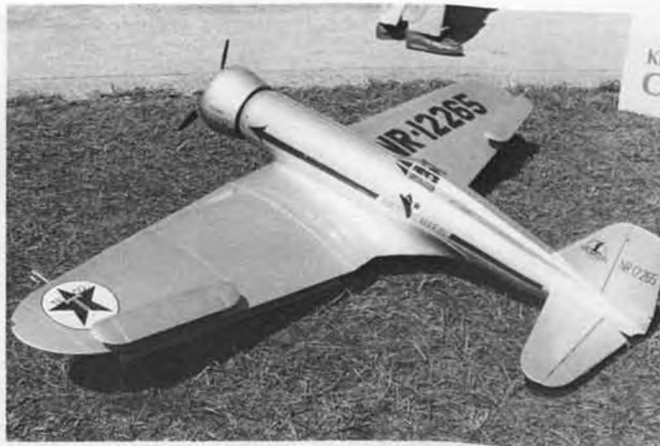
Northrop Gamma by Jack Cole and Pat Corderman from Colorado Springs. An all-fiberglass model, it weighs 18 pounds with an O.S. 108 engine. This plane will soon be kitted by Jack.
