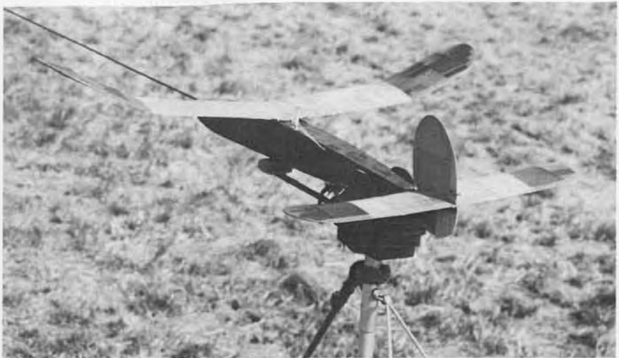
John Lenderman's original Gollywock in the winding stooge. Note the differences between this ship and Marlin's, above. Elliptical stab tips and subfin are giveaways.
