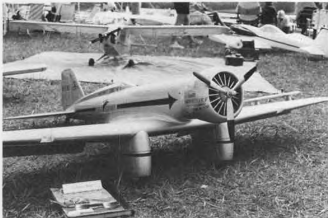
Northrop Gamma by Jack Cole and Pat Corderman from Colorado Springs. An all-fiberglass model, it weighs 18 pounds with an O.S. 108 engine. This plane will soon be kitted by Jack.
