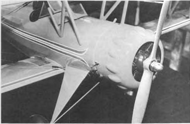
Cowl in place showing engine control; lower wire at rear is the needle valve, other is choke control.
