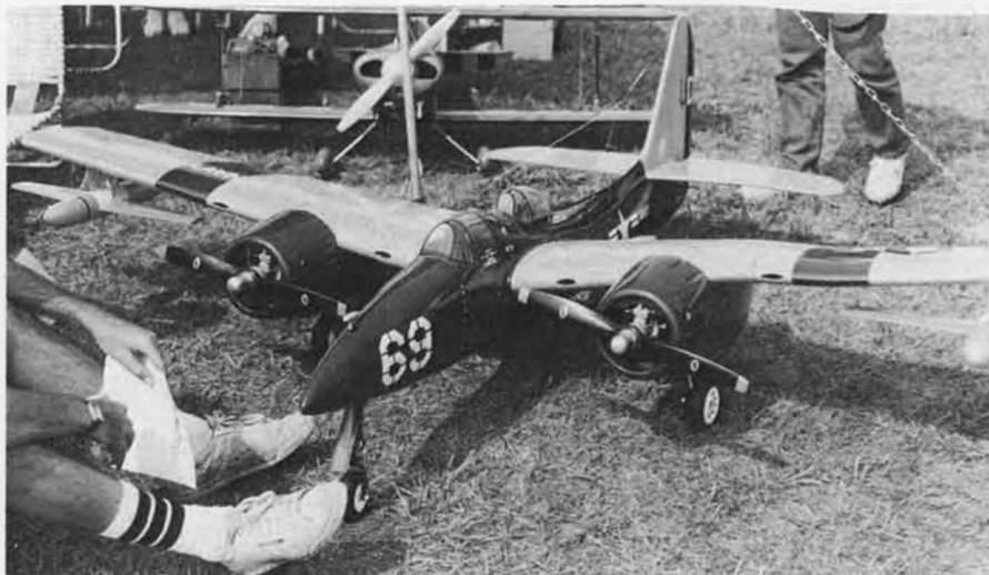
This F7F-3 Tigercat by Ed Sheldon and Bob Antonelle of CBA models is to be a kit soon. Powered by two S.T. 2500s, the 'cat's span is 97 inches.
