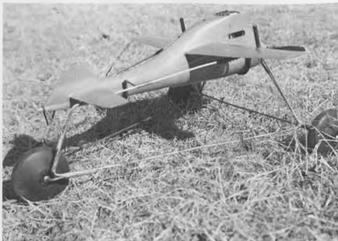
A McCoy .60 ignition engine converted to glow to power this speed ship. Best recorded speed was 129.03 mph.
