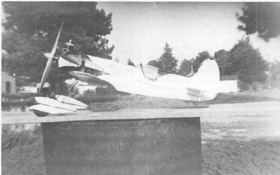
Lee Hoffman's first gas model, circa 1937, a Stenzel Tiger Shark, powered by an Ohlsson .19.
