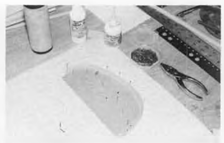
Forming a wingtip bow using cardboard form.
