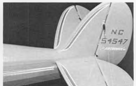
Tail from above showing faired fabric fillet covering as described in text.
