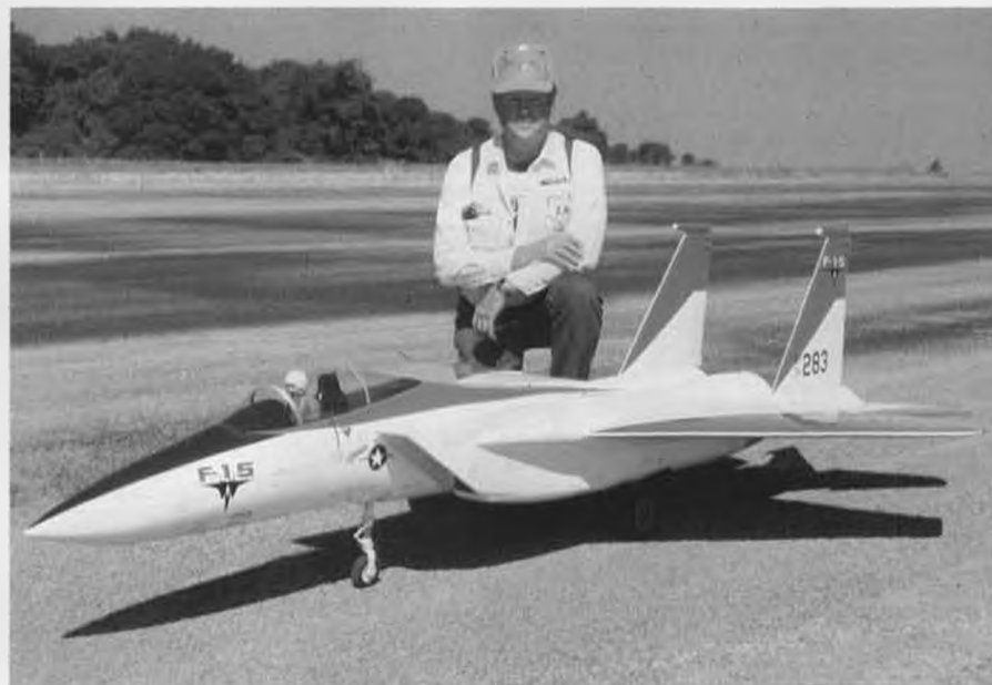
Ron Ables with his Byron Originals F-15 Eagle. Probably the largest model at the Fan Fly, it was most frequently flown twin-powered by two O.S. 77s, with Byrofans.
