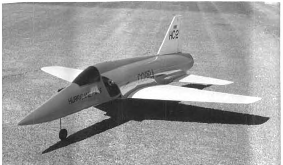
Steve Korney's Cobra powered by his original Hurricane fan with a Rossi .90.
