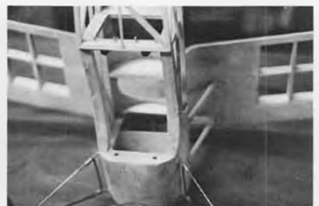
Lower wing saddle and landing gear in place.
