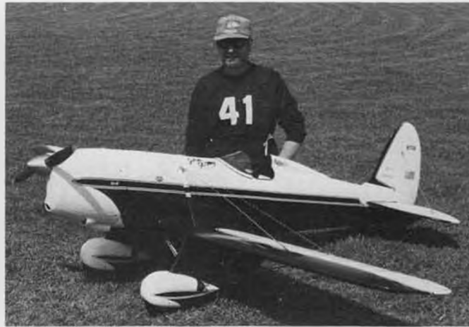
A 90 cc chainsaw engine pulls this 47-pound Ryan STA through the air with Mark Collins at the controls. Span is 118 inches.
