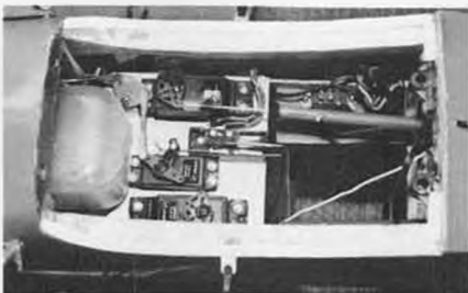
Note 90-degree reversing bellcrank for reliable link to throttle. Glow heater switch box seen here in center.
