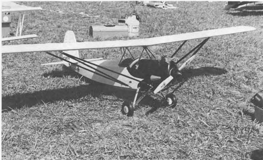
Jack More's Heath Parasol was powered by his own homemade .90 4-stroke engine.
