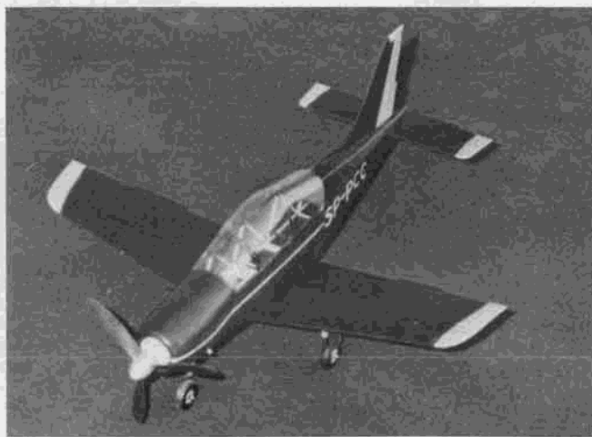
Canopy can be stretched or vacuum-formed. Walt scavenged a canopy from Golden Age Repro's P-51 kit.
