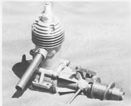
An Atom Minor Mk III, machined up from castings by Bruce Abell. Turns 5,000 rpm with 14x5 prop.
