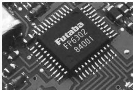
An inside look at the R129DP shows the exclusive Futaba PCM 1024 microprocessor and surface mount construction (SMT).
