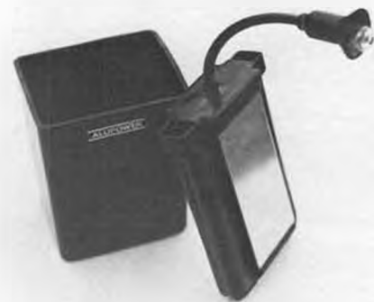
The unusual aluminum/air battery. See text.
