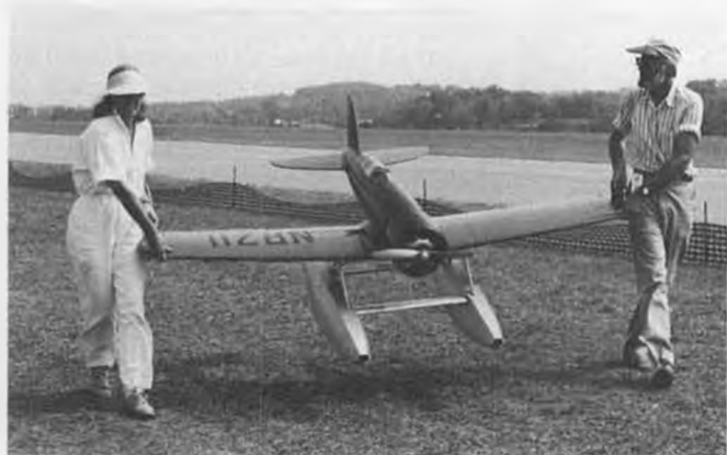
Wendell Hostetler's Lockheed Sirius on floats. It had vintage wheels hidden in floats which allowed takeoffs from runway. Good flyer.
