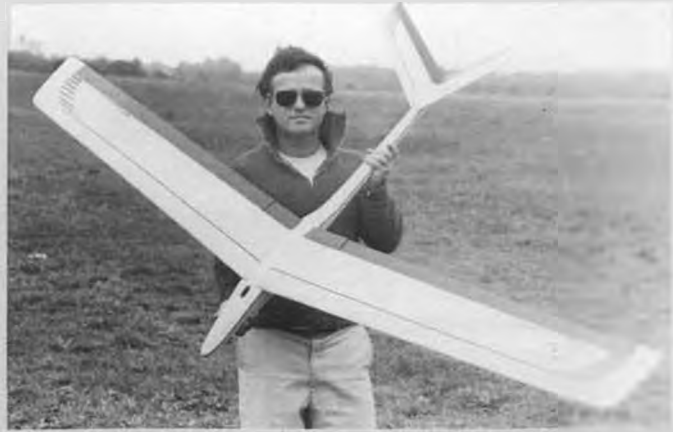
A little more serious Walter and his two-meter Alcedo original design. V-tail has elevator only, wing has ailerons only.
