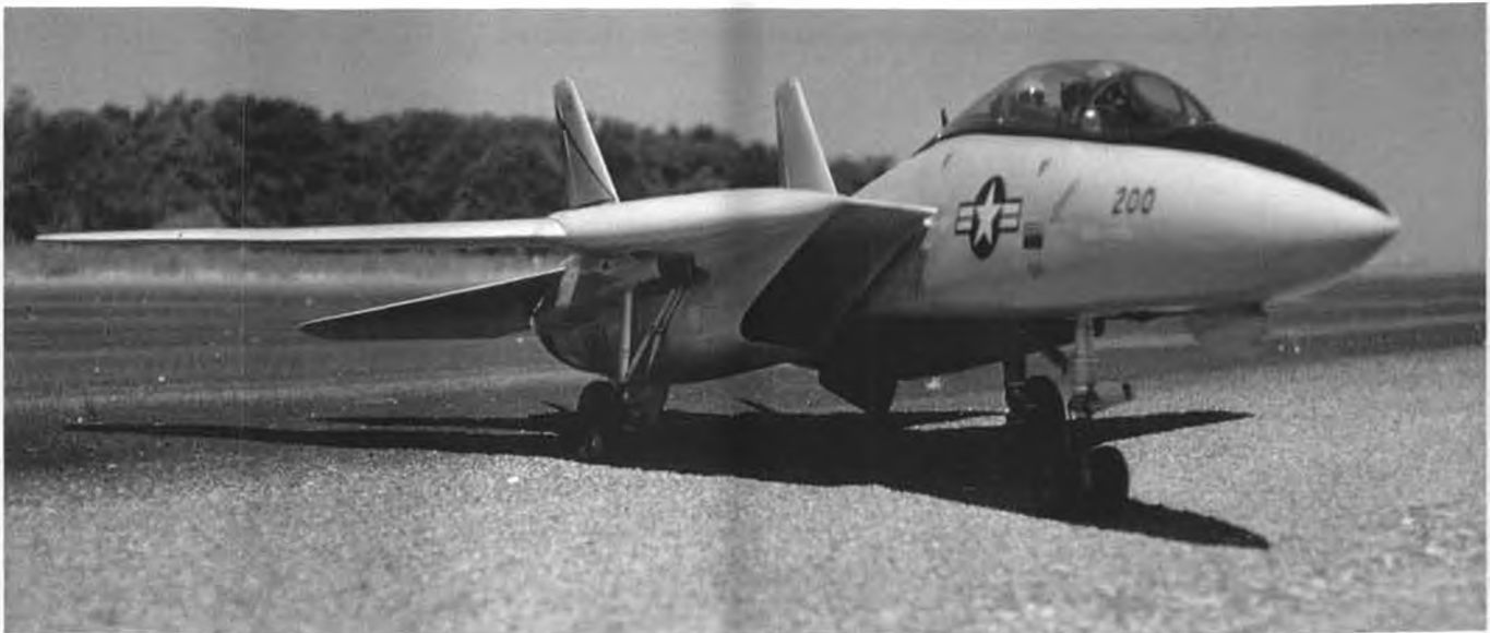
The 1/9th scale Grumman F-14 Tomcat soon to be marketed by Yellow Aircraft. It is powered by twin Dynamax fans with O.S. 77 engines.
