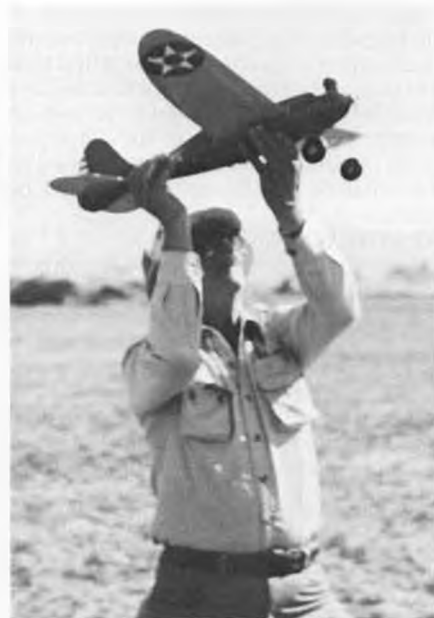
Clarence Bull's A.J. Walker Fireball done up as a free flyer, powered by an O&R .23. Fireball is a steady, fast flyer.
