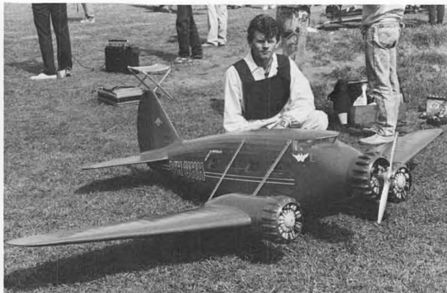
Ian Forrester's 108-inch span Stinson R. Powered by an S. T. 2500 and an 18x10 prop. This big quarter-scale craft tips the scales at 23 pounds.
