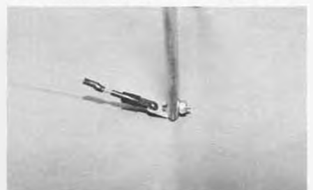
Flying wire attachment at interplane strut. Aluminum tab is free floating.
