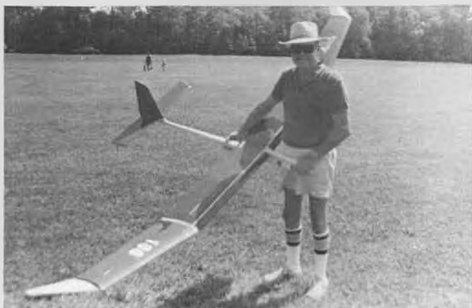
Stretched Gemini built by Bob Champine and flown by Fred Gregg. Has Selig S4233 airfoil and 1140 sq. in. wing area.
