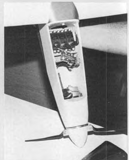
Inside the fuselage of the Project Fred. Lots of room for servos or speed controllers. Astro Challenger 05 direct drive motor and Airtronics radio gear shown.
