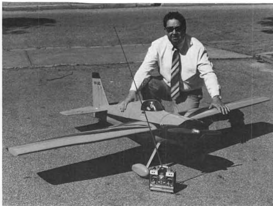
Leo O'Reilly with his quarter-scale Laser 200 with an Enya VT 240, and an 18x10 propeller. Weight is 19 pounds. Seen at the Bicentennial Model Aircraft Pageant in Australia.
