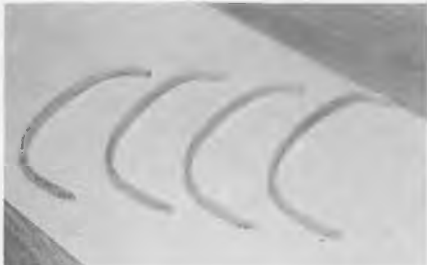
Wingtip bows ready for cleaning and trimming to finished length.
