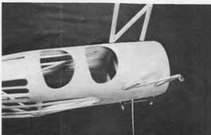
Cockpit cutouts with cabanes in place. Note filler blocks between stringers.
