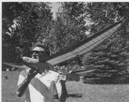
Bruce Augustus and his Thermic 72, with tissue on the wing and stab, silk on fuselage.
