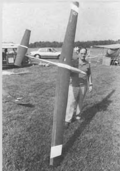
Don Goughnor and his Swag 134-inch Unlimited ship. Has 1120 sq. in., Eppler 214 wing, NACA 0009 stab, weighs 70 oz.
