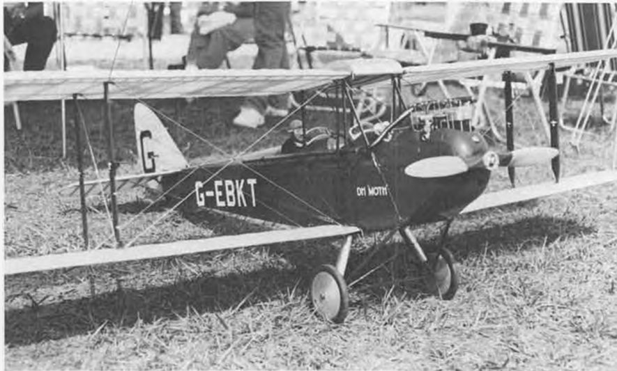
Seen at the IMAA Giant Festival: a beautiful Gypsy Moth by Merrit Aimmerman, complete to the last detail. Flies with his own Cirrus 4-cylinder 4-stroke engine.
