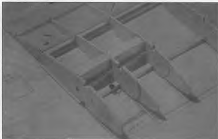
The two-piece wing is joined by a length of music wire inserted into a brass tube in each wing half. Note plywood wing rib doublers and the 1/2" thick tube support blocks.
