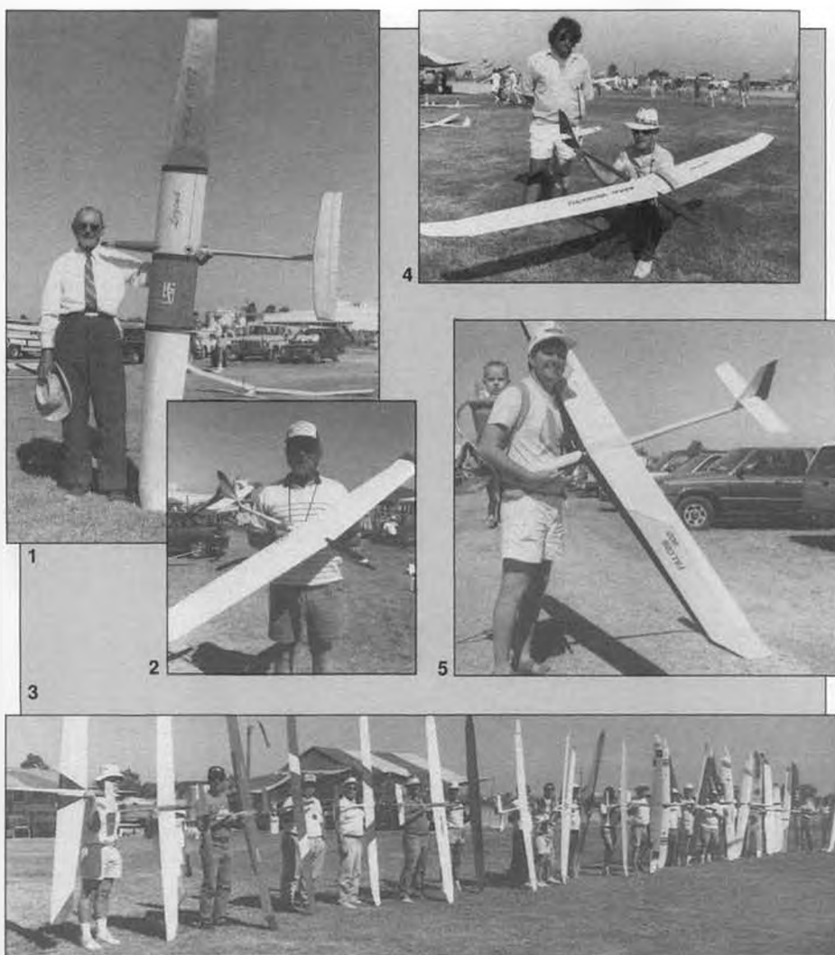
(1) The fourth Legend flown was Col. Bob Thacker's early prototype, which had flaperons on its center panels and aileron-less polyhedral tip panels. Not as maneuverable as later aileron versions. (2) Brad Clasen finished in 1st place at this year's Fall Soaring Festival flying a Falcon 880. Here he holds a two-meter version called a Falcon 600, a new design from Flite Lite Composites. (3) Count 'em, 27 Falcon 880s and 800s! And at least three had already been put away when this shot was taken after the close of the meet. In two years this design has caught on like no other since the Sagitta 900.
