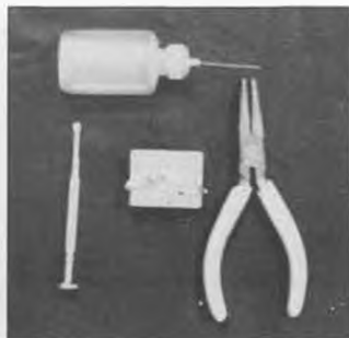
(Left) Some examples of clockwork engine timers. At left is the latest model available from Tatone and KSB; early style Tatone at middle top; Tatone 1/2A Tickoff at middle bottom; and the Tatone Flood-off timer at right. All of these can be cleaned and repaired, as described in text. (Middle) To properly clean and repair timers, you'll need a jeweler's screwdriver, smooth-jaw needlenose pliers, and a pin-point oiler filled with light oil. Also needed is a small ultrasonic cleaner or a small container with a tight fitting cap, for cleaning parts in solvent. (Right) This is what the timer works look like with the faceplate and back cover removed. Stalick photos.
