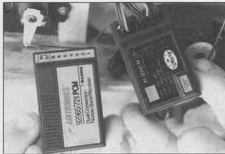
Stu chose the Airtronics-compatible RCD FM receiver as the heart of an extra airborne RC system working from his same Vanguard PCM transmitter . . . he now flies two different models from a single transmitter by switching from PCM to PPM as needed. Very cost-effective.
