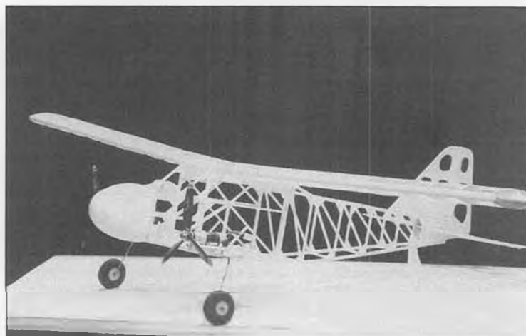
The completed, uncovered structure as seen here, but sans motors, should weigh in at about 2-1/4 pounds. Finished model comes in at 6 pounds.
