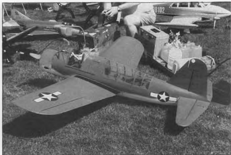
OS2U "Kingfisher" by Dave Gaur, Hanover Park, Illinois. Weight 23 lbs., span 84 inches, all balsa covered with glass cloth and epoxy resin, 3.2 Sachs Dolmer, 1/5-scale.
