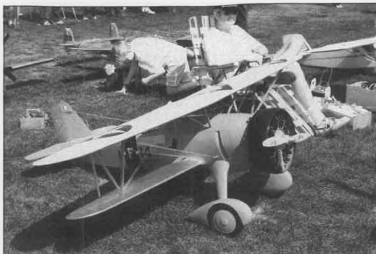
Curtiss F11C-2 "Goshawk" in quarter scale, is latest plan offering by Don Nell, Lincoln, Nebraska. Span eight feet, 30 pounds, 3.2 Sachs Dolmer.
