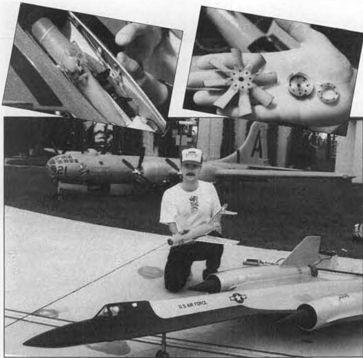
Bob Hahn, Costa Mesa, California, poses with his mini-ducted fan Mig-15. Byron's SR-71 in foreground and B-29 in background. (Insert, left) Close up of Bob Hahn's Mig-15 interior. (Insert, right) Bob Hahn's Mig-15 eight-blade fan is fashioned from cut-down wood propellers.
