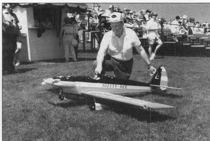
Ed Izzo, Orlando, Florida, and his Bizzee-Bee. Powered by a Sachs Dolmer 3.7 engine, Ed's converted Bridl Big-B includes his own smoke system with outlets on both wingtips and fuselage.
