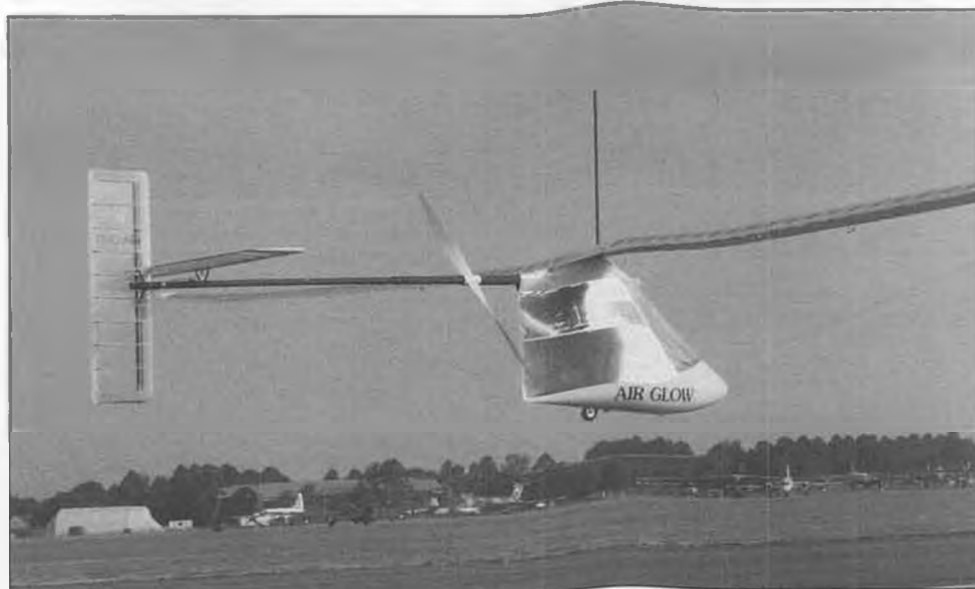
The British "Air Glow" human powered aircraft, built by a group of modelers and being flown here by 18-year-old Nick Weston. Configuration appears to be quite similar to the U.S.-built Daedalus MPA. Whether the Air Glow will go after a performance record for MPAs, is unknown. Photo by Ron Moulton.
