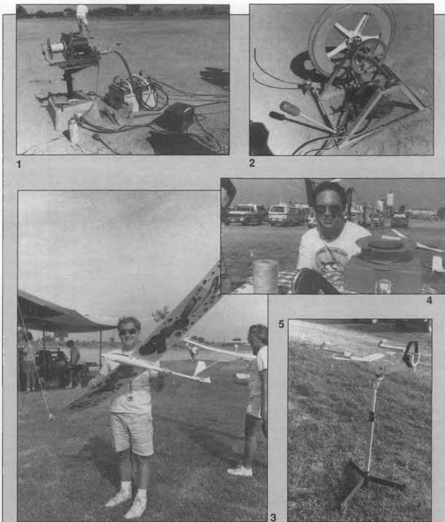
(1) Visalia's Central Valley RC fliers go all-out to provide the best anti-backlash 12-volt winches. Permanent winch pylons with AC outlets for the chargers keep the two batteries up to nearly full charge all day long. (2) Winch line retrievers allow launch-a-minute pace. They are a modified Davey Systems type with a starter motor that hangs by gravity on a pivot plate to maintain belt tension. Tension release handle at lower left. (3) Ken Adcock had fun with anyone who admired his skill with an air brush . . . make that a Pep Boys automotive decal set! Model is a Buzzard glass fuselage with Olympic II wings and stabs. (4) Norm Tibbs Engineering (1672 Los Osos Valley Rd., Los Osos, CA 93402) sells winch and glider accessories, including the nicest ball bearing turnaround our columnist says he's ever seen. AMA safety rule switch (right) and H.D. solenoid (left) are "must have" items. (5) Dean Aldinger's adjustable tripod Falco stand, which he engineered and made himself out of aluminum and foam rubber. Makes for much easier model setup.
