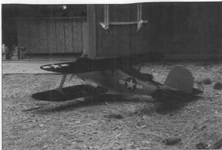
The author's Byron Beech Staggering in Navy service colors. Weighs 20 pounds, powered by ST 3000 turning 18-8 prop. Airtronics Vision radio; flaps, retracts, acrylic lacquer over fiberglass.
