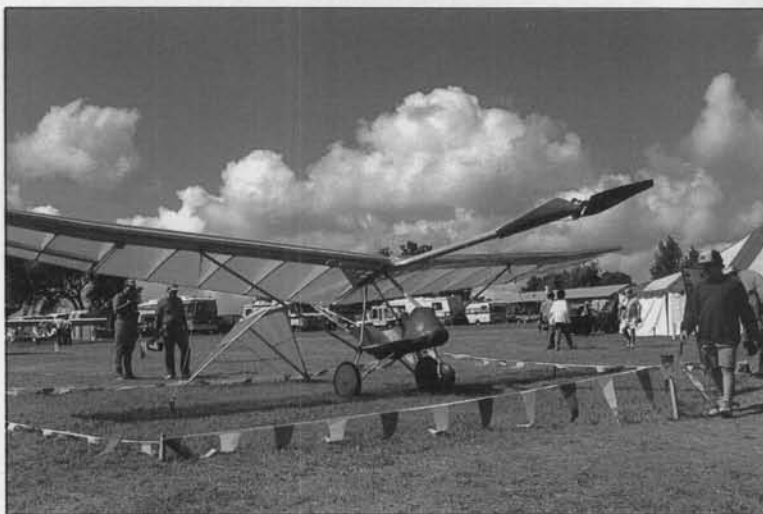
Believe it or not, this is a man-carrying rubber-powered aircraft! See details in text. Photo by Frank Scott.
