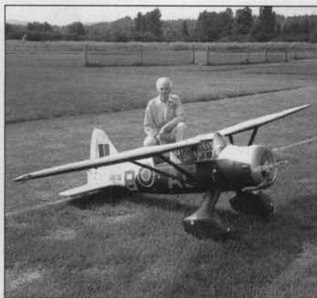
Edward Hess did a great job of scratch-building this 12-ft. Lysander. It weighs 32 pounds, is powered by a Quadra 52, and is guided by a Futaba 1024 PCM.
