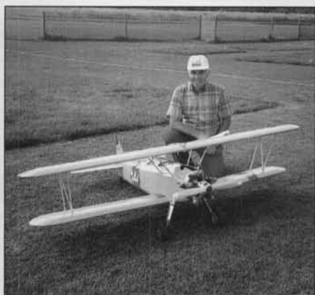
An O.S. FR 500 powers Ward Emigh's scratch-built Ziroll N2S-5 Stearman; 28 pounds, Futaba radio. Robart landing gear is fully functional.
