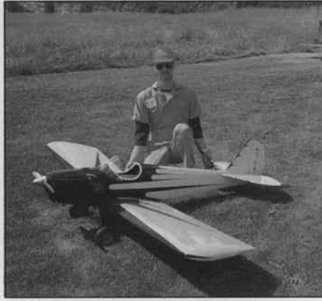
Troy Klein builds like a pro. His Sig Spacewalker weighs 20 pounds, has a 104-inch wingspan, and a Futaba five-channel radio. The Spacewalker is powered by a 2.5 cu.in. Remington.
