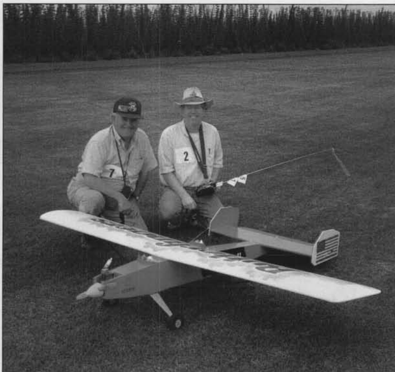
Jay Hopkins, left, built this candy bomber; Dave Denison does the flying. Dave says the "Butterfingers" uses stealth smoke. Big Bird has a 96-inch wingspan, uses O.S. 91 F/S and Futaba radio.
