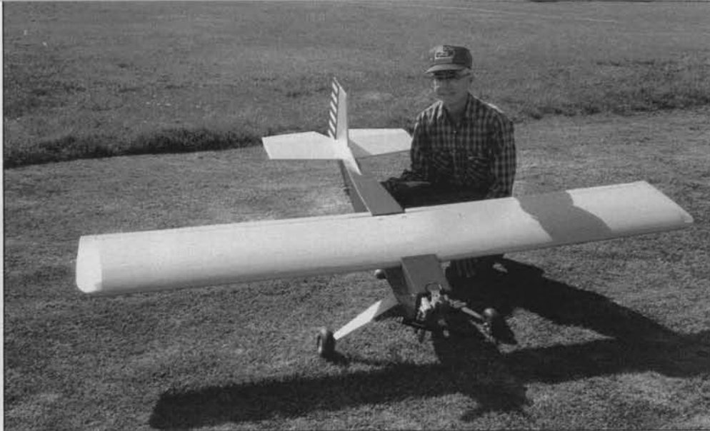
This Roadrunner has a 96-inch wingspan and weighs 14 pounds. It is powered by a Zenoh G-23, guided by an Airtronics PCM. Bill Maloney really enjoys his plane.
