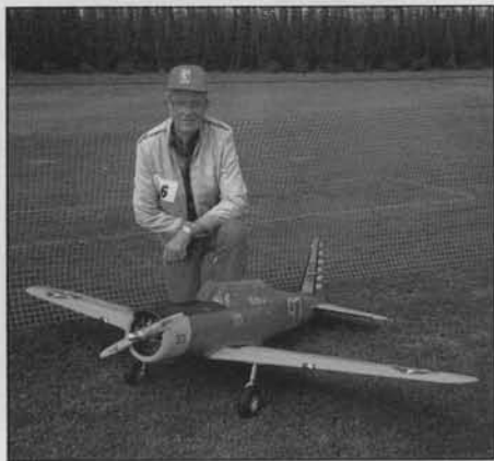
Bert Baker, at 6 ft. 9 in. tall, dwarfs his BT-13 Vultee Valiant, better known as the Vultee Vibrator. This Big Bird has a 92-inch wingspan, weighs 21 pounds, and is powered by an ST3000. Radio is a JR PCM 9. New kit is available from Bert.
