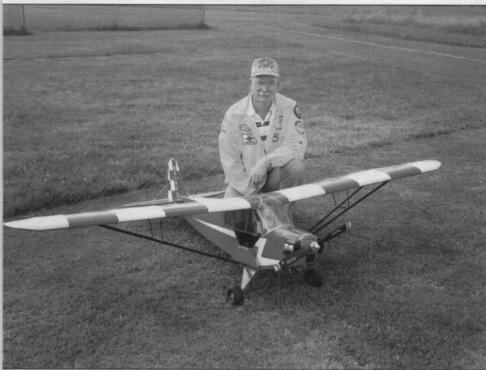
An O.S. FR 500 powers Ward Emigh's scratch-built Ziroll N2S-5 Stearman; 28 pounds, Futaba radio. Robart landing gear is fully functional.
