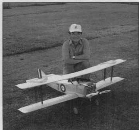
A Sopwith Pup built by Sveng Lee has a 66-inch wingspan. Sveng uses a JRx347 radio and an O.S. 1.20 F/S for power.
