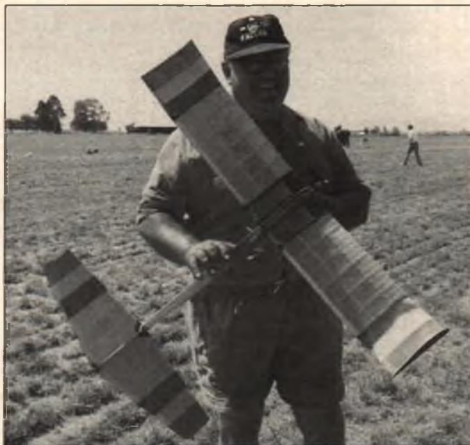
John Crossetto always comes to the N.W. Free Flight Champs with a passel of 1/2A models. This is the classic RamRod 250 by Ron St. Jean, which John flew to 3rd place in Nostalgia. Power is a Cox reed valve .049.
