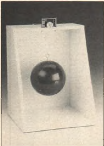
The JR MES-4721 servo lifts a 16-pound bowling ball. One powerful servo! See text for our columnist's comments.
