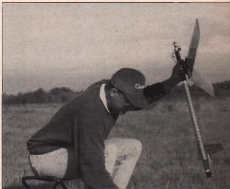
Mike Slessor produced this F1J model, which has some characteristics of the 1/2A Vee published as a three-view in a recent issue of Model Builder . Mike found he had to increase the dihedral to 11 degrees in order to get consistent flight patterns. Impressive performer with a Tee Dee .049. Photo by Bob Stalick.
