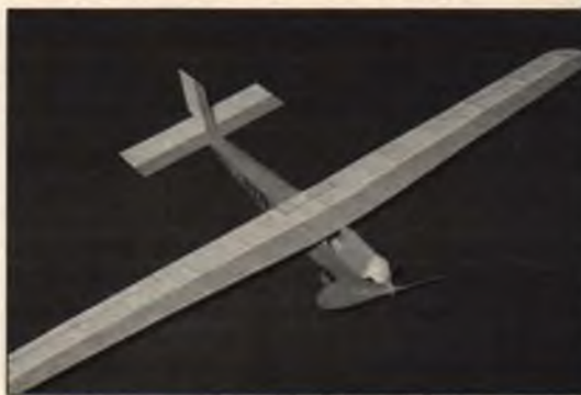
Top & Above: The author's replica with and without its clothes on. The long, high aspect ratio wing gave the full-size aircraft outstanding performance on only 32 horsepower—the model is likewise an excellent flier. It's designed to take full advantage of the 9-inch fuselage rule, hence the greater-than-normal (for a Peanut) wingspan of 17-3/8 inches.
