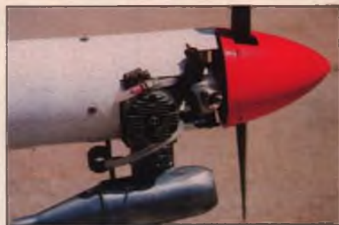
A Webra Speed .40 serves as the motive power in the author's test model. Nose gear is factory installed, and the spinner is furnished in the kit.
