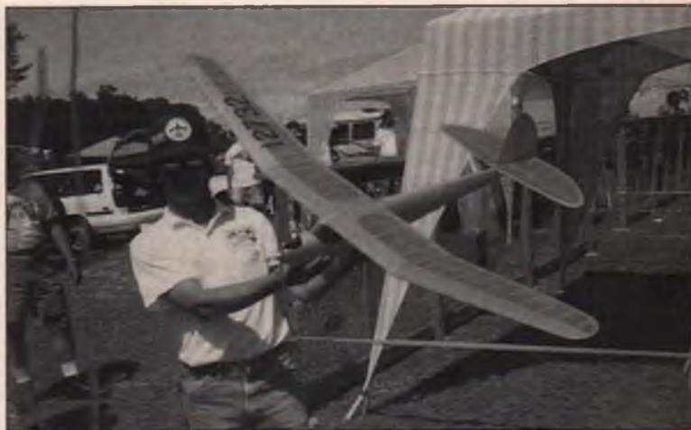
Photo No. 3. Bruce Gornig, of SAM 75, holds Walt Geary's 400 square inch version of the Megow Chief, a potent competitor in Class A RC events. Power is an ElfIn diesel.
