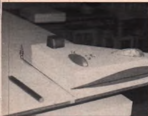
The setup for cutting the Delta Vee wing cores via the "pivot point" method. It's a one-man operation and requires only one airfoil template. This technique was explained in detail in a past "Model Design and Technical Stuff" column by Francis Reynolds—see text for reference.
