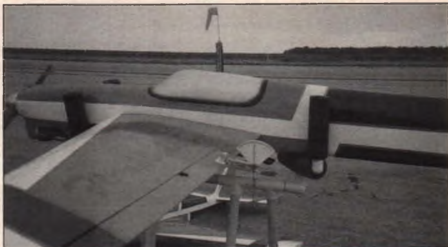
The Breene Aircraft Throw Meter, a handy setup and trimming tool, shown clipped to the aileron of Dennis Breene's Flashback II. The Flashback is Dennis' own design for 1.20 engines.
