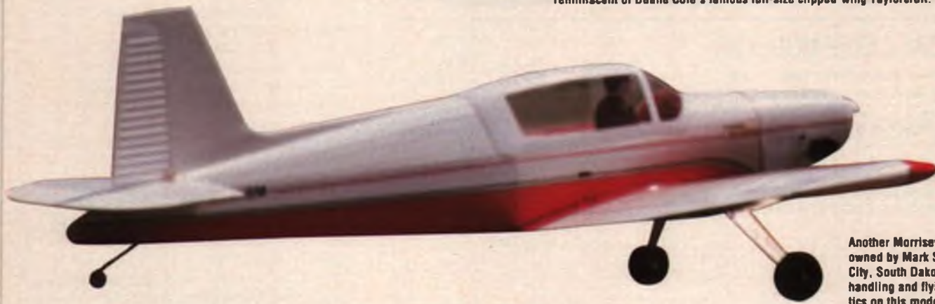
Orv Shields' Sig Cadet Senior is powered by a K&B .65 Sportster. Orv customized the plane by making it a taildragger and adding ailerons, giving it an appearance reminiscent of Duane Cole's famous full-size clipped-wing Taylorcraft.
