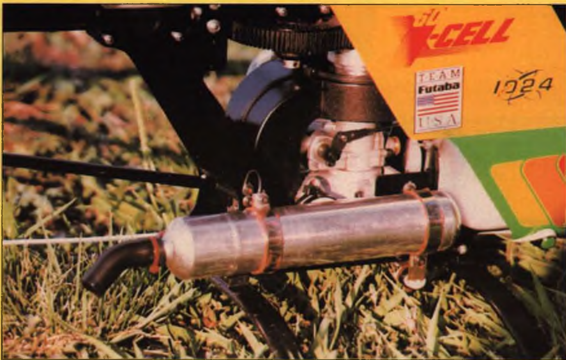
The YS .61FSH inside our author's X-Cell 60. The engine cylinder faces toward the rear of the helicopter. Note the 1/2-inch diameter knob on the bottom of the crankcase opposite the carburetor; it is the idle adjustment knob. Text gives hints on how to set up a YS carburetor. The Hatori 666 muffler is very quiet and causes minimal power loss—an excellent combination. This motor loves 38% nitro fuel and hot plugs, like the Enya 3 or Fox.
