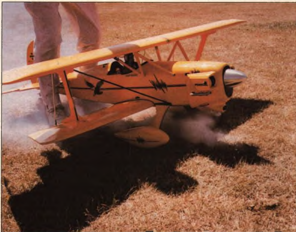
Above: Walt Wyrick's smoke system puts out a good deal of the white stuff. An S.T. 3000 powers his Der Jaeger biplane, and a Perry pump moves the smoke oil. Below: Lloyd Marohl's Grizzly Bear looks great in the air because he set up his muffler to blow smoke over and under his wing. Power is a Zenoh G-62.
