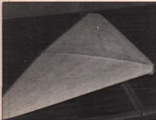
Bottom view. The protruding plywood spine serves as both a skid and launch handle. They don't show up here, but the spine has three narrow slots flush with the bottom of the cores, through which fiberglass strapping tape is passed and stuck to the cores to serve as a wing spar.
