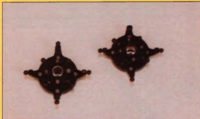
This is our columnist's favorite new item for the month, an all-metal swashplate for the Hirobo Shuttle from Century Imports. There is no discernable slop between the rotating and nonrotating pieces; an excellent piece of work.
