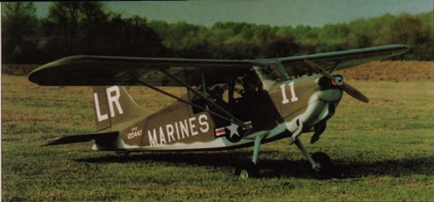
Vally Aviation now has plans for this Stinson L-5E Sentinel. Model has a 102-inch wingspan, weighs 14-18 pounds and uses engines such as a Zenoah G-38 or Quadra 35. Details in text.
