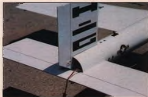
View of the tail shows the tight, clean mating of all parts. On/off switch is in front of the rudder, and the battery charging connector conveniently hangs out the tail opening.
