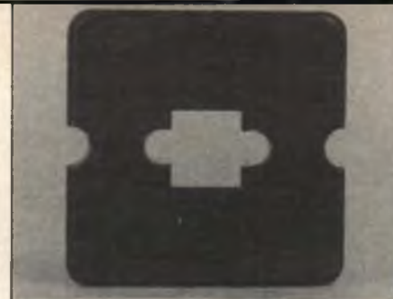
Here are the half-round cutouts that must be made in the pushbutton mounting plate to mount the D&R stick assembly. The outer half-holes mate with similar cutouts in the transmitter case to complete the mounting holes for the base of the stick assembly.
