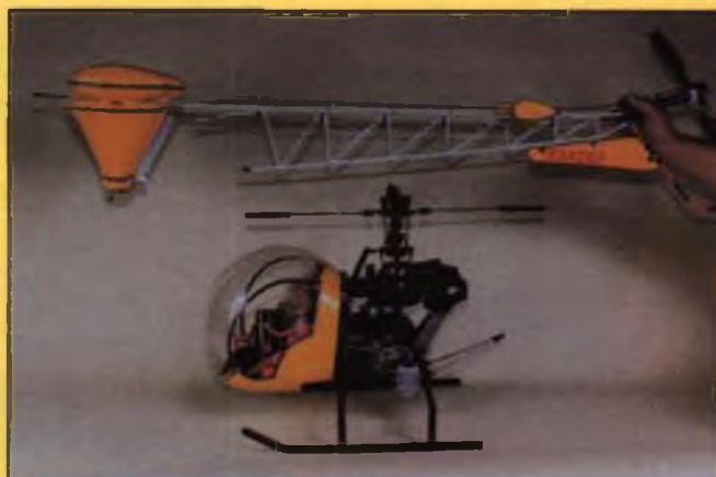
James flies an X-Cell 60 with the new Robinson R-22 scale conversion kit from Century Imports. Because it is not a full-fuselage scale ship, it is fairly easy to add to a stock X-Cell 60. Due to its clean lines, the model is relatively fast and does nice autorotations.
