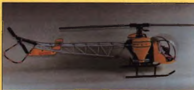
Century Imports recently introduced this Bell 47G scale conversion kit for the Miniature Aircraft X-Cell 60. The scale-looking aluminum truss tailboom is welded by the factory and is finished with white powder-coat paint. Also included is a welded metal landing gear, anodized black. The main cabin and dummy fuel tanks are fiberglass. For information on this or any of the other Century Imports items pictured on these pages, give them a call at (408) 942-9521.
