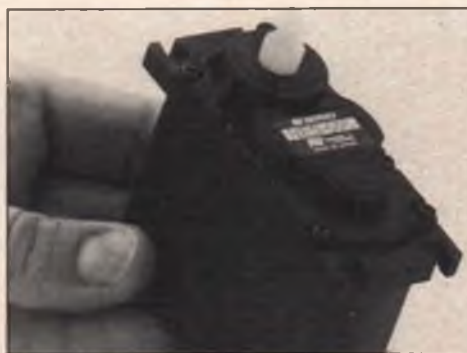
The new JR NES-605 servo is a big one. Intended for quarter-scale and larger airplanes and cars. Its modern design includes all features required for this exacting application.
