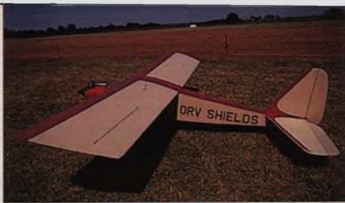
Orv Shields' Sig Cadet Senior is powered by a K&B .65 Sportster. Orv customized the plane by making it a taildragger and adding ailerons, giving it an appearance reminiscent of Duane Cole's famous full-size clipped-wing Taylorcraft.
