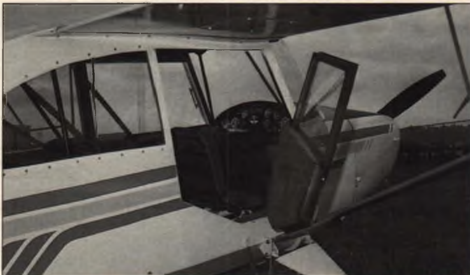
The interior of Bo Moore's 1/3-scale Aeronca Champ is nearly perfect and uses material from a full-scale aircraft supplier. The 42-pound model is powered by a Zenoah G-62.
