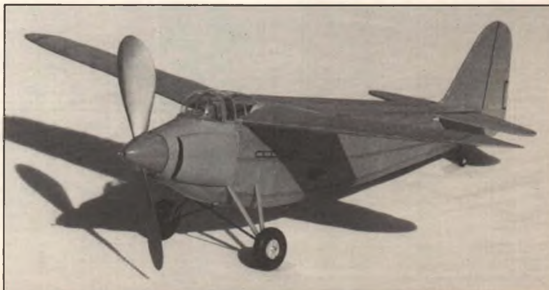
Peanut Scale Koelliker F.K. 55 is one of Michael Morrow's projects. This particular model has turned in a high time of 61 seconds with a plastic prop. Plans are available - see text.
