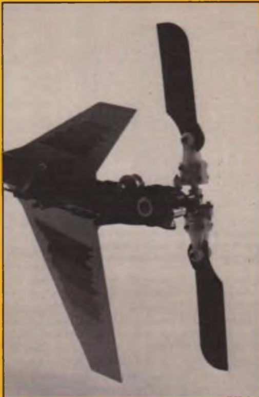
The Ninja Pro Master's new glass-filled nylon tail rotor blades have swept tips and an efficient reflexed airfoil.
