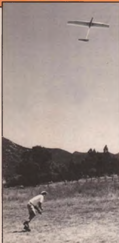
Art Markiewicz is a real hand-launch fanatic. He's long been his own aircraft designer, but he's now also a regular contest winner. His airfoil of choice is the RG15, a fast, low-drag section which he can modify into a good thermal section using camber changing—note the curve under each wing. Construction is molded glass fuselage, glass sheeted foam wings . . . no wood anywhere.
