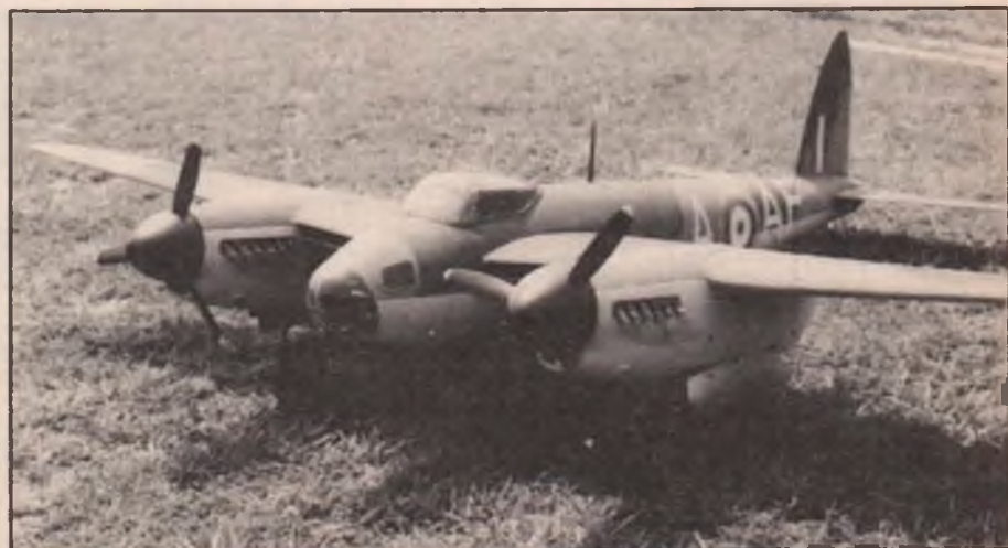
Beautiful building job on Dave Grilo's 81-inch span DeHavilland Mosquito, powered by two geared Astro 40s turning three-blade 12.6x3 props. Thirty-six 1700 3CRC cells provide 5-1/2 to 6 minutes of realistic flight time.
