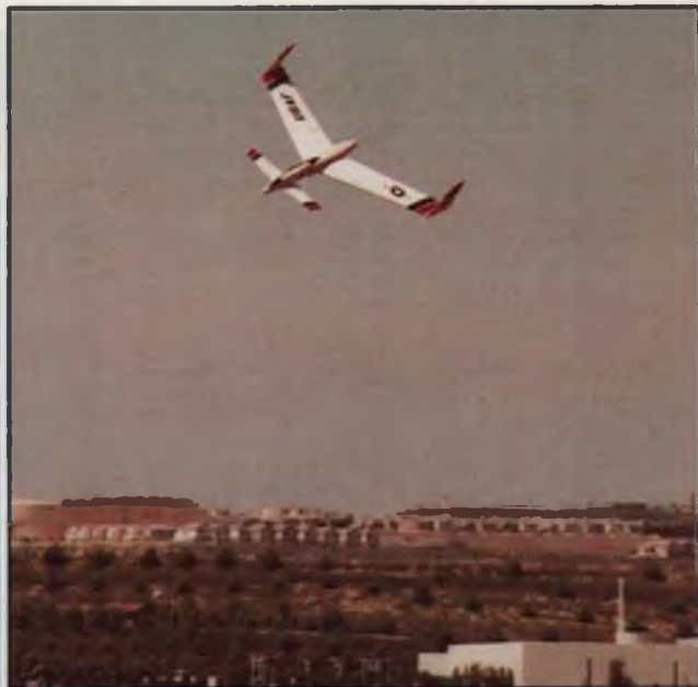
In the air the Tri-Star presents a striking profile from any angle. Dave found the CG and aileron reflex settings to be quite critical to achieving the very best performance, so don't be afraid to try different combinations while getting the model sorted out.
