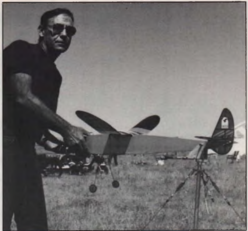
Frank Roberge flew a George Reich design, the Double Feature, in Small Cabin Rubber. While winding for his first contest flight, the hook pulled out of the winder and totaled the first two bays of the nose. Fortunately Frank had some balsa sticks on hand and rebuilt the front end right on the field; to re-cover the nose he stripped off part of the Mylar covering from one of his other models and soon had the model back in the air. Didn't win or place, but he sure came away with a fun story to tell!
