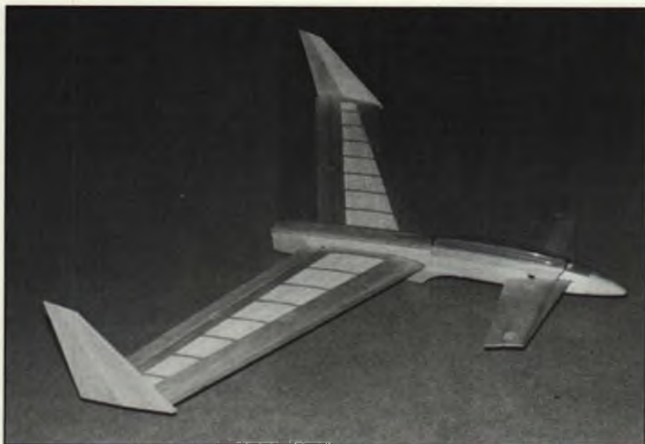
All framed up and ready for covering. Model features a partially sheeted foam core wing, conventional sheet balsa fuselage and canard. Belly pan is molded ABS plastic and is rugged enough to stand up to some pretty rough landing abuse.
