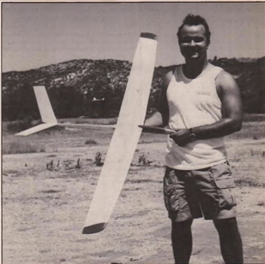
UCSD student Aaron Valdes, fresh from his Soar Mats victory, almost pulled off another win at the Fall Classic. He dropped to 2nd place after a tough flyoff round. He flew an Art Markiewicz design based on a Climmax fuselage and Art's hot-wire cut, fiberglass sheeted RG15 wings and symmetrical stab. Pre-preg carbon fiber spars are just under the 1.5-ounce glass cloth. Model takes four Futaba S133 servos to operate the flaperons and mixed V-tail.
