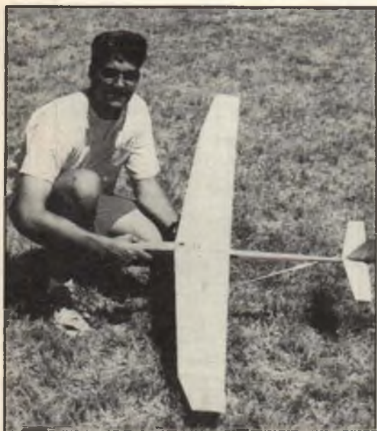
Brian Allan drove 500 miles to attend the SD meet. His HLG, which he calls the "Wisp," is a fine example of cutting-edge original design. Glass fuselage was laid up in a friend's mold, wings are Brian's own. He first tried the E387 airfoil, which he said did not perform as well as his current S4083 wings, which he likes. He says he's going to try the S7837 next.
