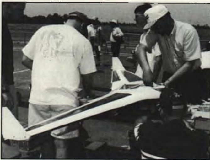
■ ABOVE: Note the interesting aft fuselage construction on Grove City College's (Grove City, Pennsylvania) design; three carbon fiber tubes between the cargo compartment and the tail assembly—most likely done to reduce the fuselage's projected surface area.
