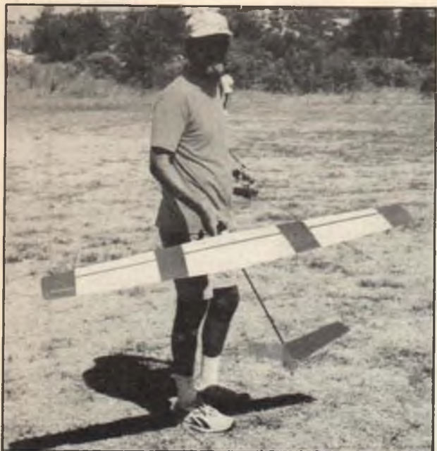
Mark Gumprecht used to fly curved and bent-wing HLGs; now he's into ailerons! The wings are unshoed pink foam covered with EsonaKote. The spar is a 1/32 vertical grain shear web with I-beam style top and bottom caps of carbon tow. It bends tremendously (with no wrinkles in the covering), but doesn't break. Airfoil is the S7837 thinned at the tip. Wing area is 340 square. Flying weight is 11.5 ounces. Ailerons are built up and were very prone to warping in the sun until he buried a 3/32 aluminum tube in the L.E. as a stiffener, now it's trouble-free—tweak it, it stays put!
