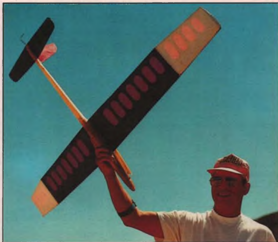
The winner! George Joy went from 4th to 1st place in the flyoff round, flying a not-quite-stock Climmax. George decided to thin out his factory pre-shooted wings for better penetration; he V-bagged the 57037 wing to 18 inches of mercury, which compressed the foam and reduced the thickness of the wing by about 2 percent of chord! Then he routed out holes in the wing to make it lighter. It now has incredible penetration with no apparent loss of climb, and little loss of strength.
