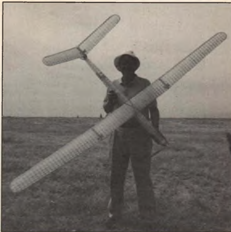
Bruce Kramer of Pacific Palisades, California designed and built this huge 8-foot span, 600 square inch rubber-powered model. The ship features a V-tail and a geared motor, and is covered with Polyspan. Photographer Sal Frucianno says it's a great performer.
