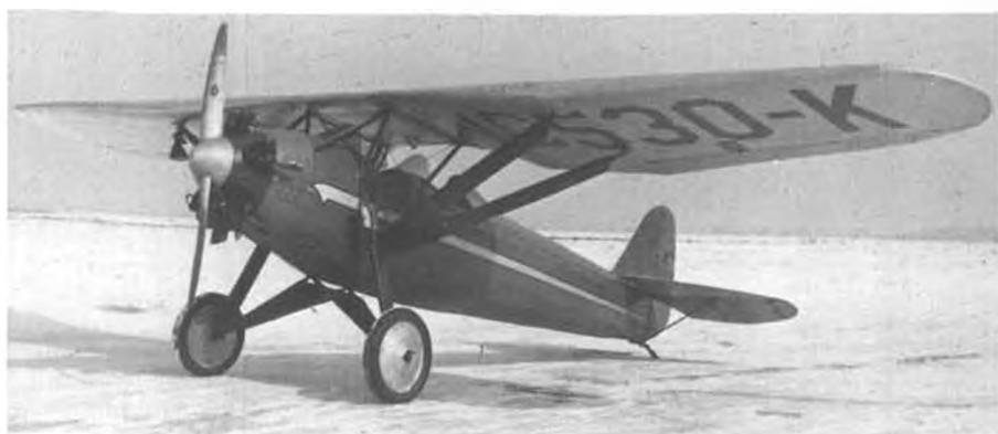
A classic of its time, the Davis V-3 was both an aerobatic plane with quick responses, and also stable and docile for the average pilot. Top speed of this LeBlond powered model was 95 mph.
