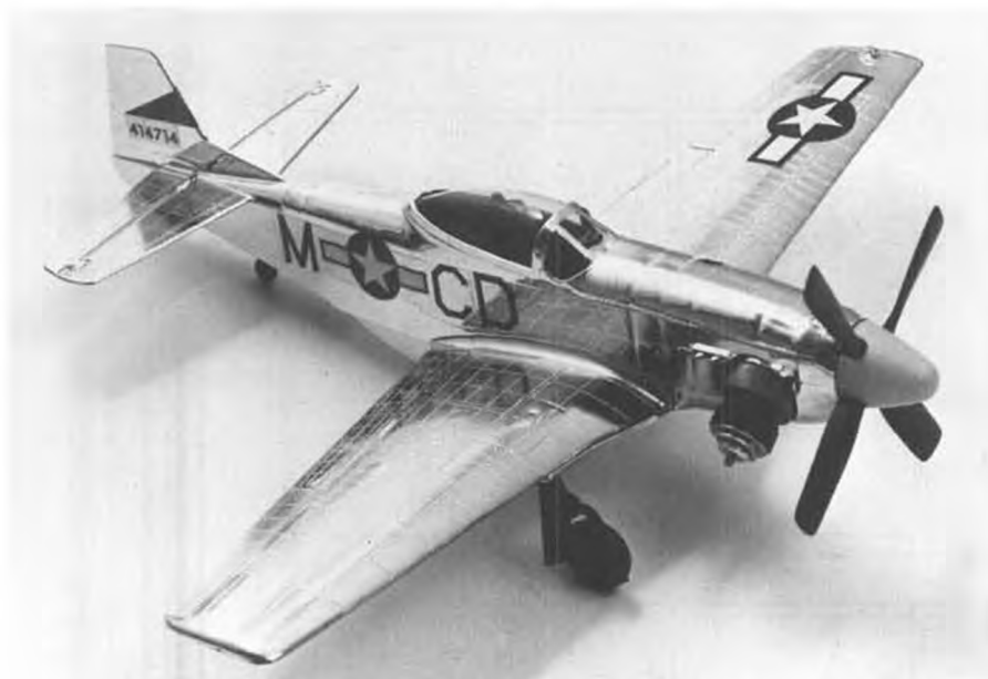
Testor's ready-to-fly planes are realistic looking, have muffled engines, and with the low pitch prop, fly slow enough to be easy to handle for the beginner. This little P-51 is typical.
