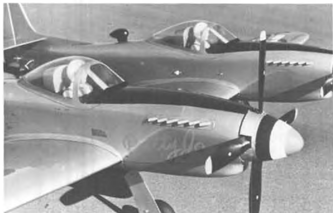
Complete airplane is built up. No fiberglass; no foam. Bob worked from only rough outline drawings, using Willis Nye 3-views in MAN.
