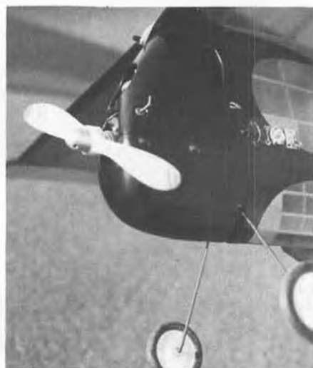
The well known stubby Pacer nose. Cowling carved from balsa block. How unique!
