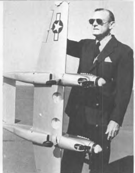
Dapper Bob shows Goldberg retracts, operated by variable travel World Engines servo.
