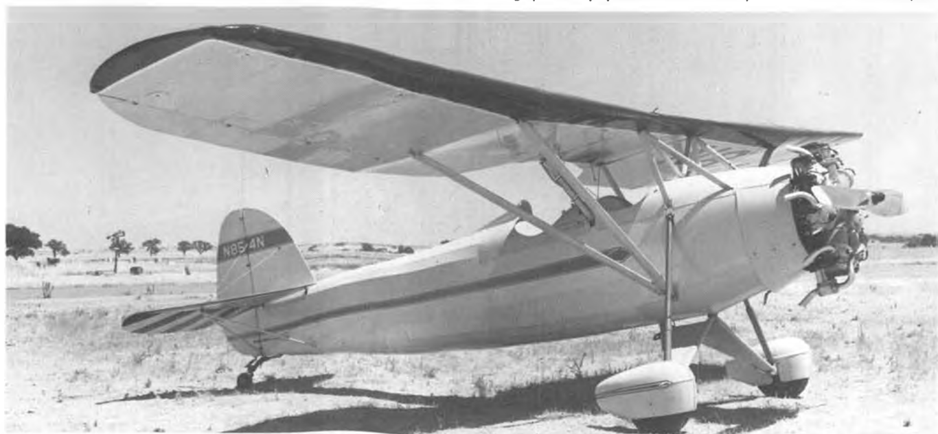
N-854N, a Davis D-1W, was rebuilt in 1965 by Joe Pfeifer of Columbia, California, with a 145 hp Warner and wheel pants from another plane. This and above photo from Pete Bowers.
