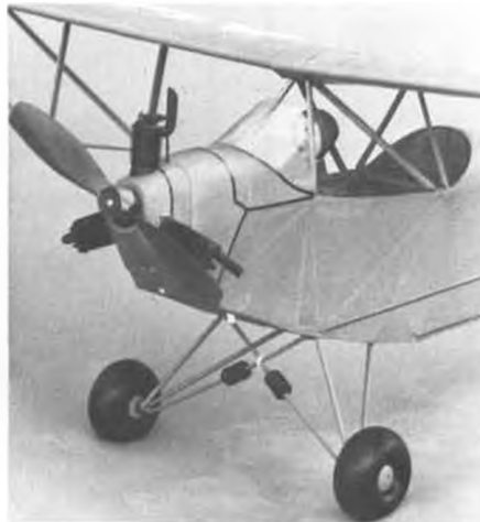
Wing is joined at cabane struts. Cover plate hides joint. VL prop painted brown grained.
