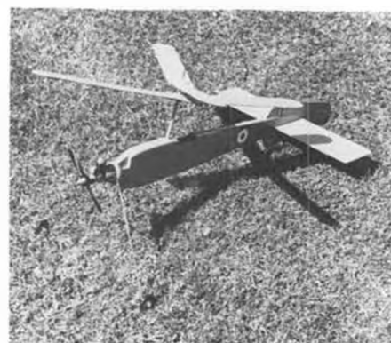
Cox powered free flight contrarotating rotor autogiro, by Bob Brown, England.
