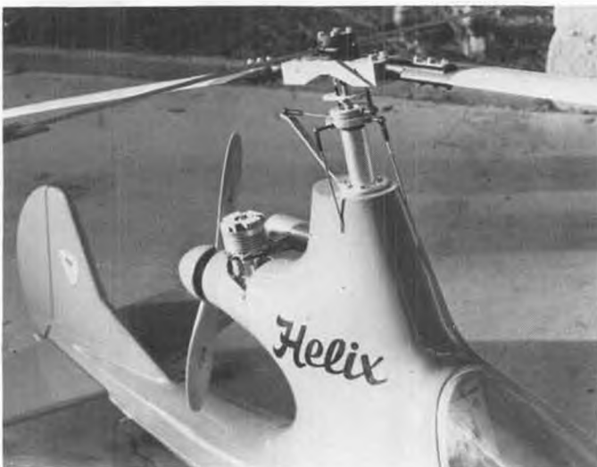
Control links to main rotor swash plate. Front rod is for up/down pitch control, side rod for L/R banking.
