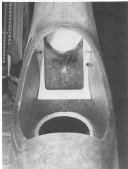
Engine and fuel tank bulkheads above, oval ring bulkhead to tail boom below.
