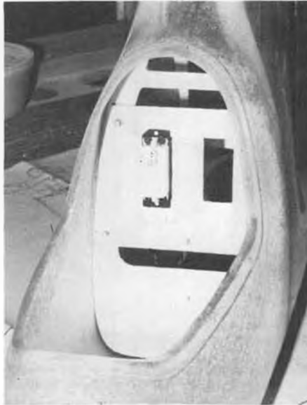
Removable servo mount in place on main bulkhead. Buckets of room!
