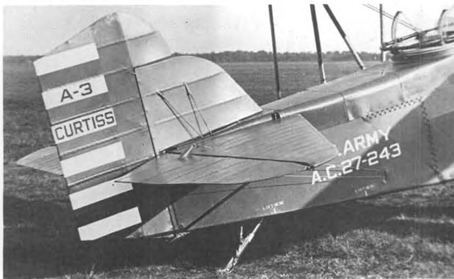
Classic Falcon tail, remembered by anyone who ever saw the airplane. Tail surfaces were dural sheet and tubing, riveted together and covered with Grade A cotton fabric.
