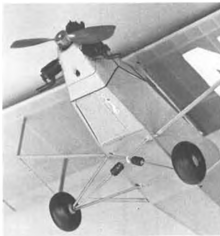
Underside of nose reveals VL switch and charging socket. Trexler wheels.
