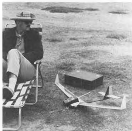
Dave Jones and his original design for Formula 72 contests. Weighs 21 oz. with Cannon Mini.
