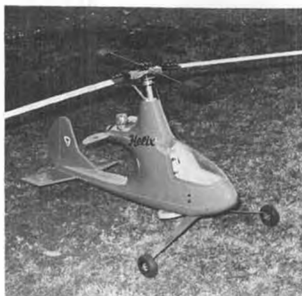
Note blade droop in at rest position. Blades "flap" upward during rotation and lift.
