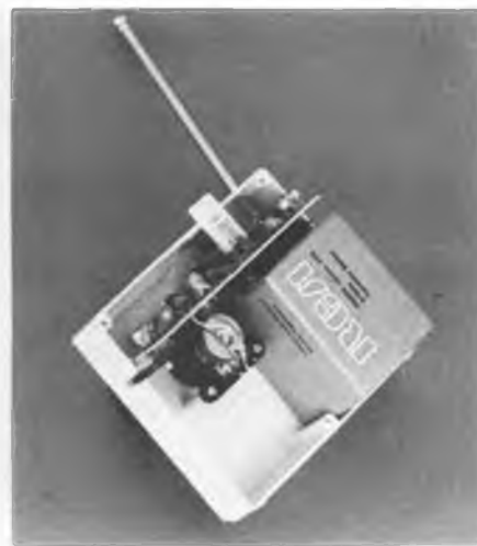
Transmitter with back removed. Note dry cell power and plug-in changeable frequency xtal.
