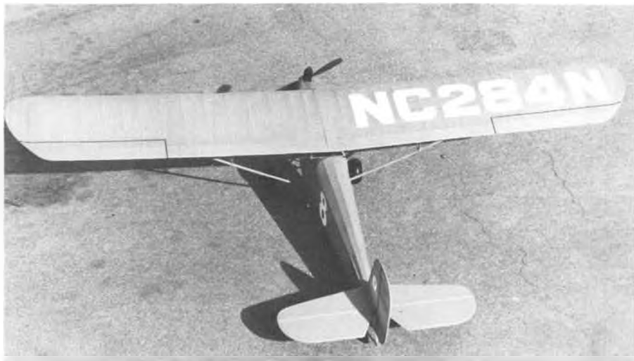
Plan view photo shows the fine aerodynamic layout for free flight afforded by the parasol design. Only changes from scale include a smidge of dihedral and slightly enlarged stab.
