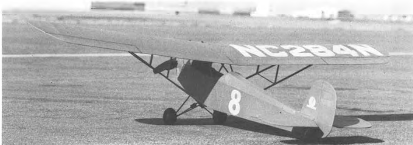
Three-quarter rear view accents long tail moment which provides excellent stability. Tail surface outlines are made from four laminations of 1/32 by 1/8 basswood strips. Photo taken at Orange County Airport, home of TallMantz Air Museum.
