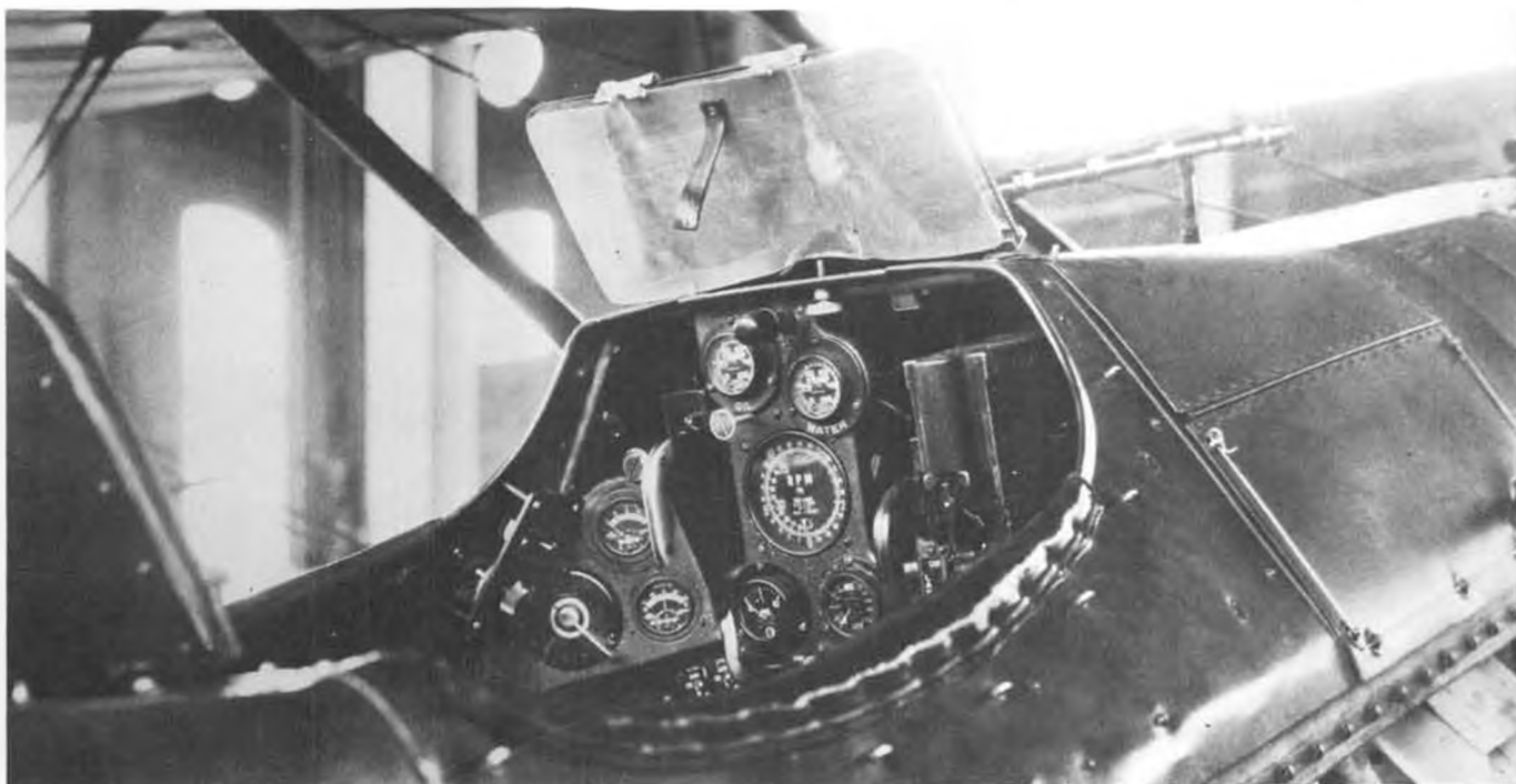
Front cockpit of an A-3B shows instruments grouped around left-hand .30 caliber Browning and right-hand .50 caliber gun. This airplane was equipped for blind flying instruction, with cover over windshield and hood fasteners.
