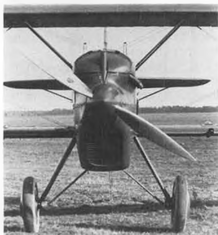
Front view of characteristic tunnel radiator. Prop forged and twisted from aluminum slab.
