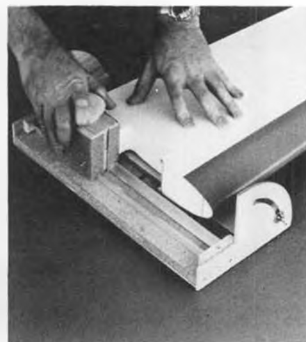
Miter Sander in use with a sheet plastic covered foam R/C wing. Tight, strong joint results.
