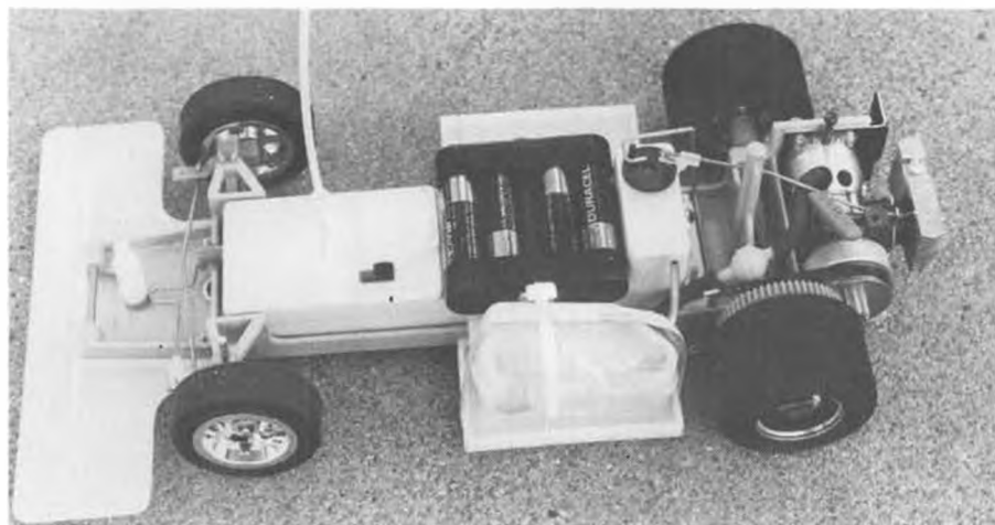
All the works are exposed with body removed. Radio batteries sit on top of receiver/servo case. Side-mounted fuel bottle feeds engine thru filter. Pull-starter just above flywheel.
