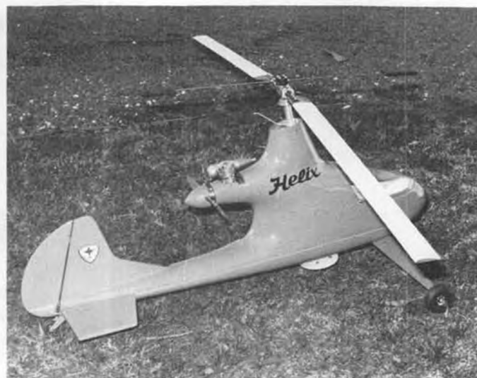
And the "after" shot, the completed Helix autogyro, before trim paint was added. Disc underneath starts rotor at takeoff.
