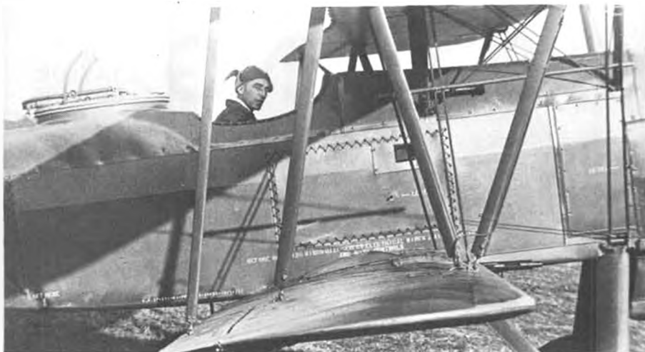
Plenty of detail visible in this A-3 photo. Browning .30 wing guns could be rigged down four degrees. Pilot had two .30's in fuselage.
