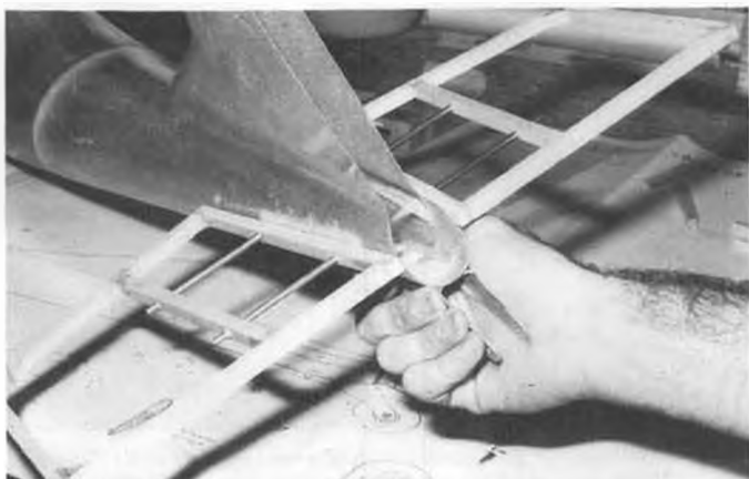
Stab is mounted plug-in style, similar to sailplane wing attachment. Tailwheel bracket bolts directly to fuselage.
