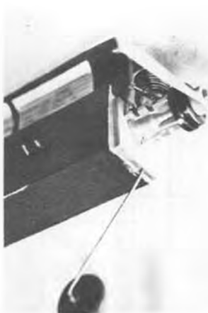
Landing gear sandwiched between 3 pieces of 1/16 sheet metal. Wire bent to match cut-out in center piece. All epoxied and bolted tight.
