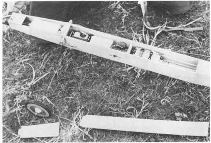
Kraft 3-channel-with-brick installation in Brian McCleave's ship. Dig the "open top" fuselage! Easy to fiddle with radio, if necessary.
