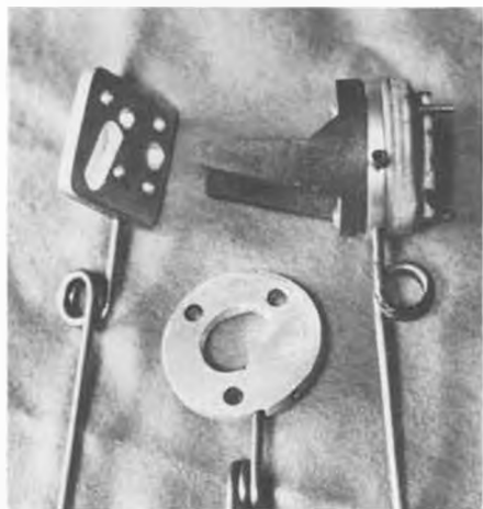
Three skids shown in different mounting rings. Note set screw in ring behind Kraft mount.
