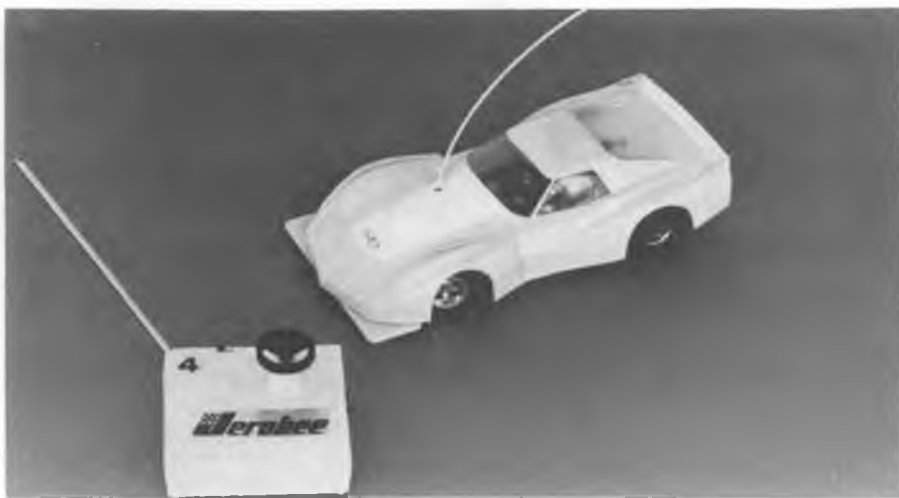
The ready-to-run Jerobee Comando 1/12 scale car with "Vette" body, and the two-channel radio transmitter (steering and throttle/brake).
