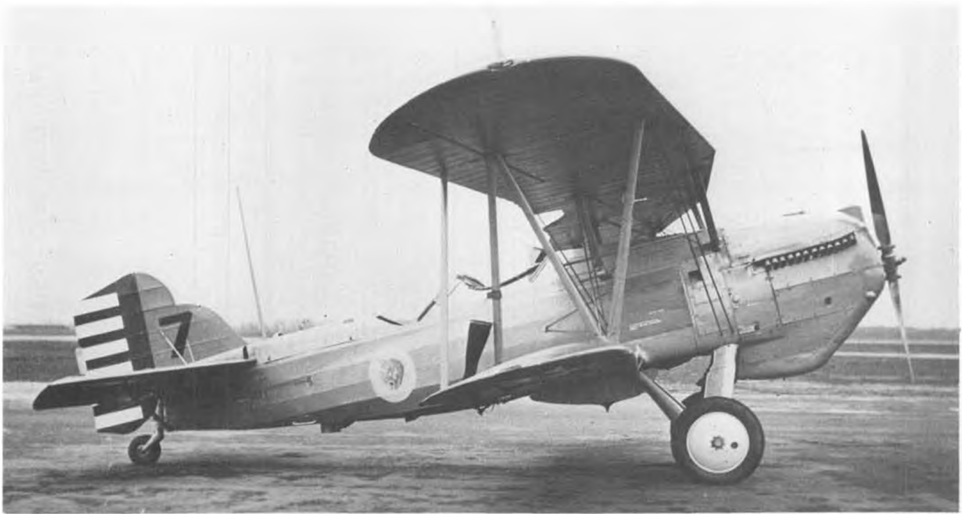
The O-1G was a greatly improved Falcon, with a tailwheel, better faired fuselage, wing cut-out, and many changes in engine cowling, landing gear, and rear cockpit. This late O-1G is also equipped with radio.
