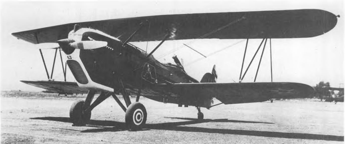
Airplane No. 63 of the 13th Attack Squadron, Fort Crockett, Texas. This A-3B had a white flash on the cowling when flown by the 13th. Rear gun is a single Browning on a Scarff ring.
