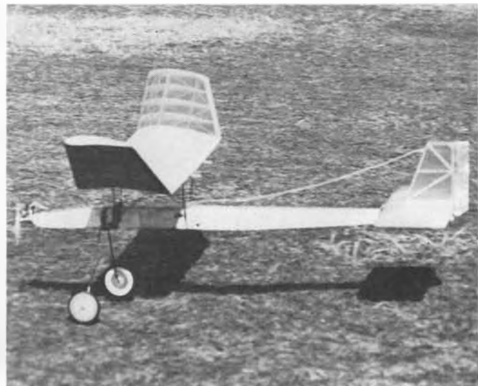
Even old timers would be jealous of that prop ground clearance! With those large, skinny wheels, you can take off from most any surface.
