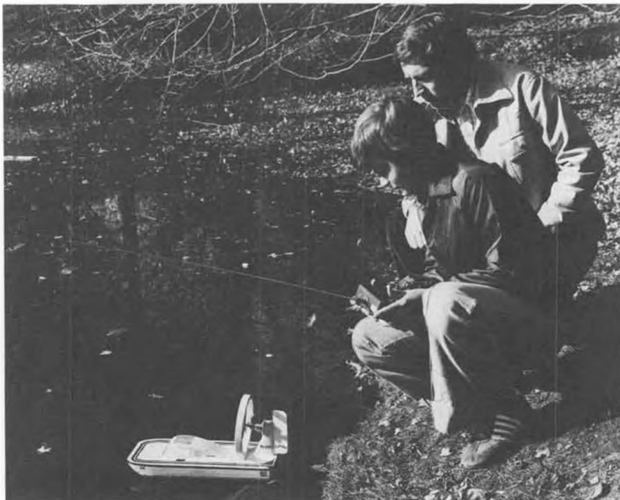
Sterling Models' latest is this molded plastic "Puddle Jumper" for water or land operation. For 2-channel radio, the .049 powered amphibian can be run in ponds or on parking lots.
