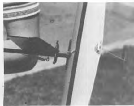
Auto-rudder and DT stab rigging. Both are very simple and fool-proof.
