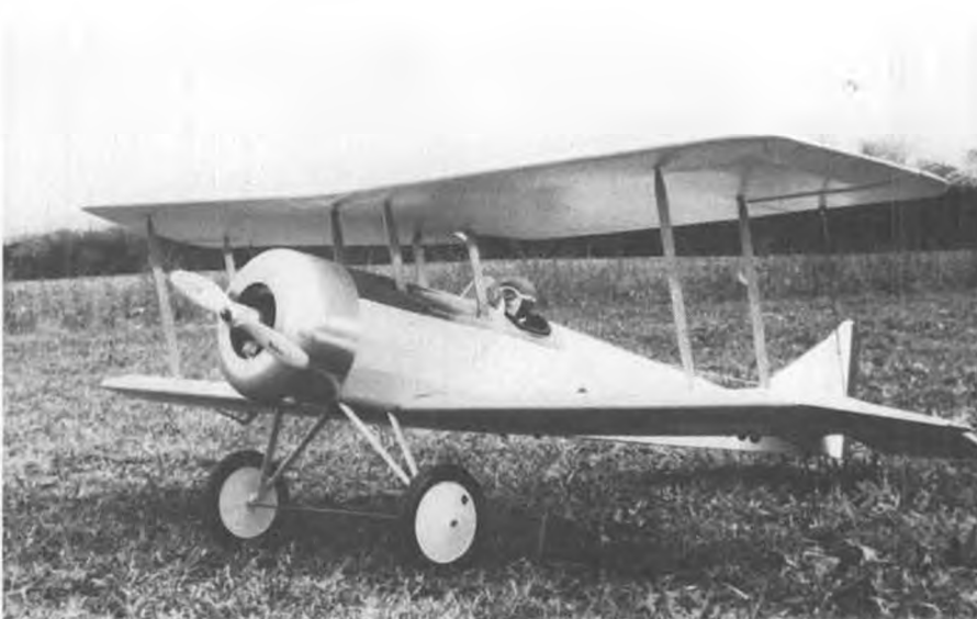
George Dickenson's Bristol Scout from another angle. The Supertigre 60 powered model is controlled by a Kraft KP7CS radio. George is now building an AMA scale version.
