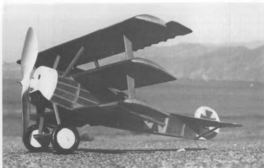
Tom Moore also built this Fokker DR-1 from Joe Wherry plans in 1946 M.A.N. Span is 19 inches, weight 2.5 ounces, and power is 8 strands of 1/8 rubber.
