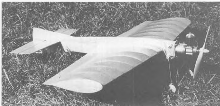
This stunt design by Boyd is an unnamed original. Span 21.5 inches, area 130 sq. in., weight is 6 ounces. Ship is fast and a bit combat-like.
