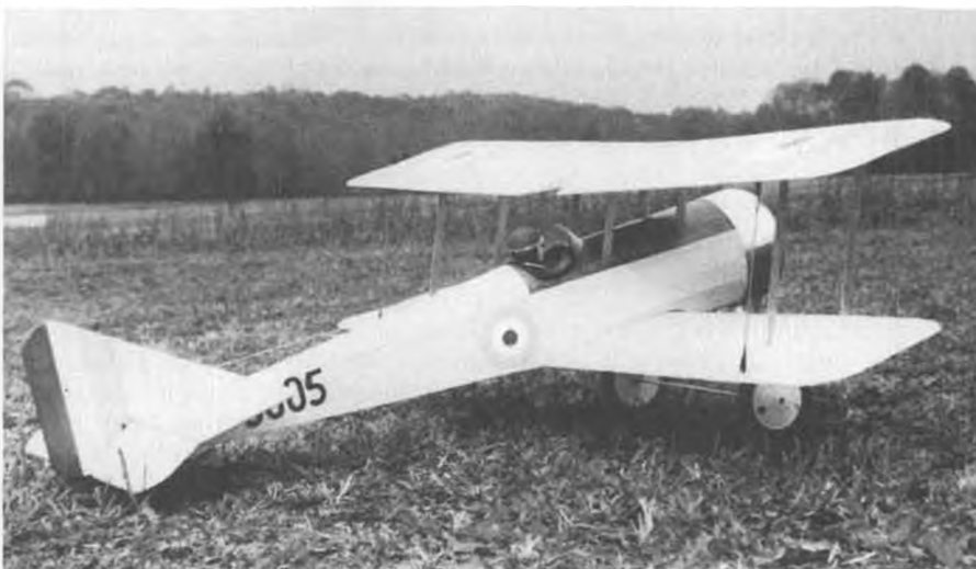
George Dickenson, Somerville, N.J., built this sport-scale 1916 Bristol Scout (Bullet) from a Strato kit. Covered with Super Coverite, it is Sig doped in Diana Cream.
