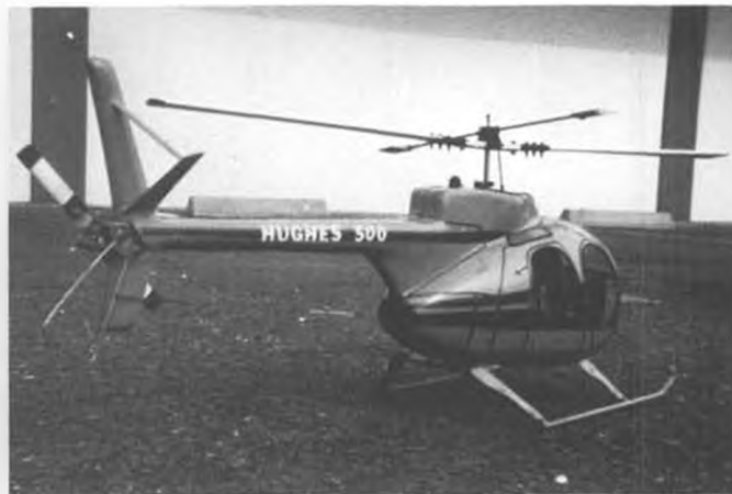
The Hughes 500 is more suited to the Heli-Baby mechanics, Scale landing gear was later substituted by skid risers.
