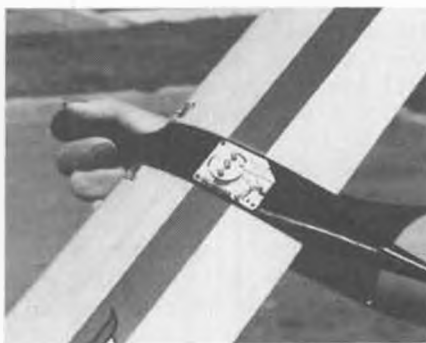
Cigar tube nose holds ballast, 1/4 inch ply core in fuselage carries all loads. 'Glass tail-boom.
