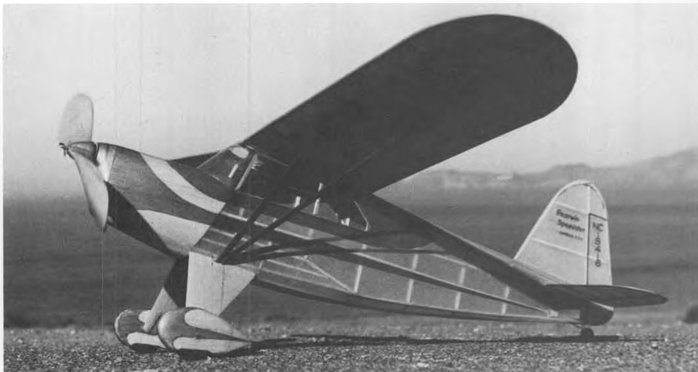
Tom Moore, whose prop building technique is described in the text, constructed this Rearwin Speedster from famous scale designer Earl Stahl's plans. Weight 2 ounces, and power is 10 to 12 strands of 1/8 rubber. Flyline Models is now kitting this and other famous Stahl designs.
