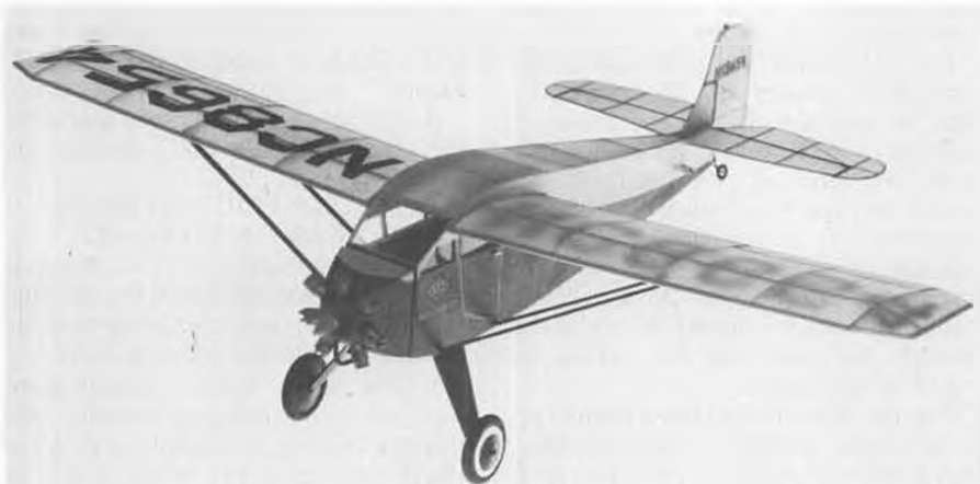
General Aristocrat Peanut, weighs 3/10 of an ounce. Finished in black and orange colors of the General "Sky Fleet". Has made flights of up to 80 seconds. Model and photo by Bob Clemens.
