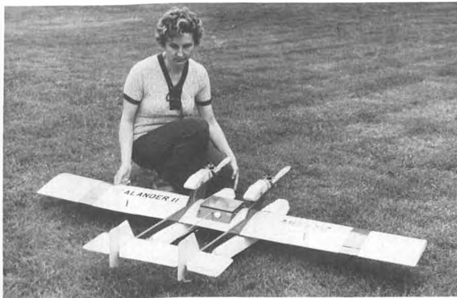
Sealand II and author's wife, Eleanor. Stretched wings, explained in text, are clearly visible. Original flights with 54 inch span, then 74, but 68 inch span is recommended. Again, see text.
