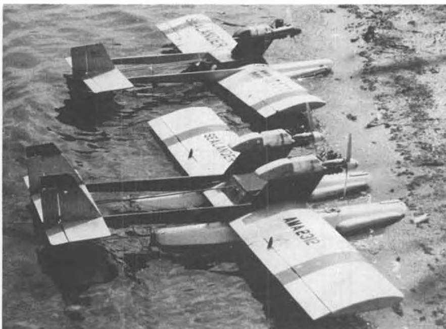
Sealanders I and II sitting at the water's edge. Note lead weights on front tips of Sealander II's floats. Like all models, Sealanders "groove" better with a forward C.G.
