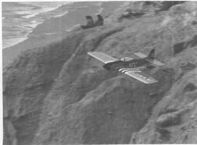
All-up weight of Mustang is 15 ounces. Span is three feet, and the model is very aerobatic. A great idea, huh, Ed Manulkin?
