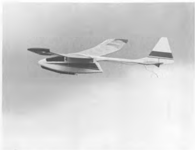
Hard to tell this is only a three-foot span model, except for the antenna wire size. It's Bob Simon again. Servos are in tandem.
