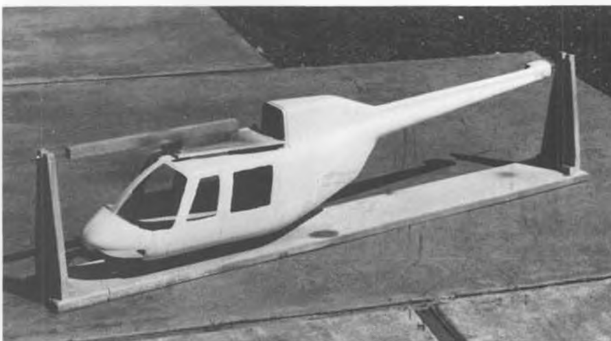
John Tucker's "fuselage holder", created for the purpose of handling a fiberglass fuselage while spray painting. Making one end support adjustable would make the jig more versatile.
