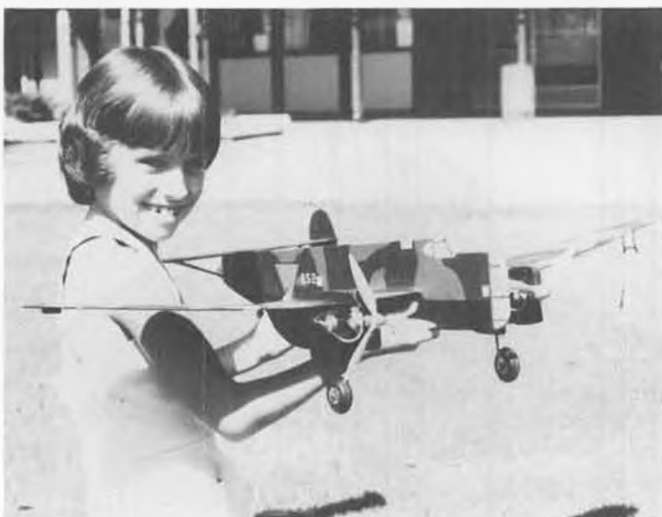
Mike's 8 year old daughter, Karen, holding the TV. Beam mounted engines offer simpler installation, TeeDee's are really too powerful.
