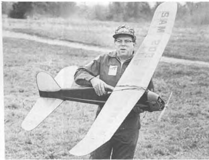
CD George Armstead and his Cyclone-powered Apache from 1941 Air Trails. Note New Ruler style fin of silk covered 1/4" al. tubing.
