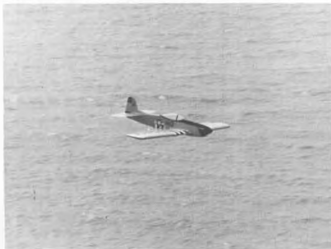
Bob Simon built this "Gliding Scale" P-51 from a Sterling control line kit. Flat pack is in the nose, receiver and servos in wing.
