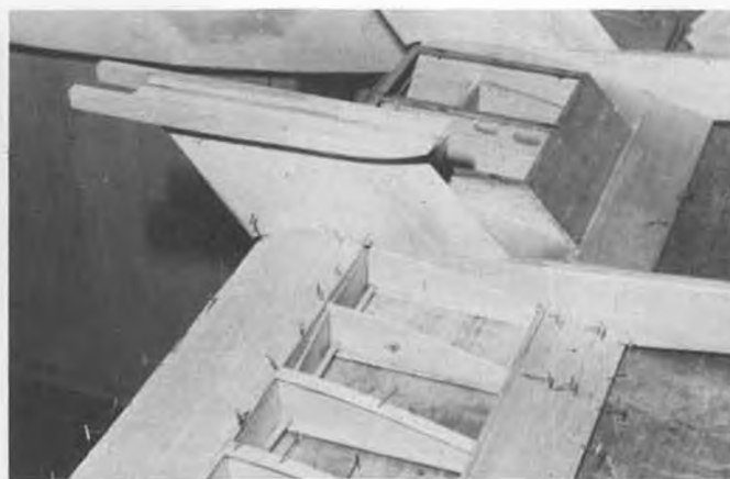
Sealander II center section during construction. Note aileron control tubing in place. Wing is semi-symmetrical but built on flat surface.
