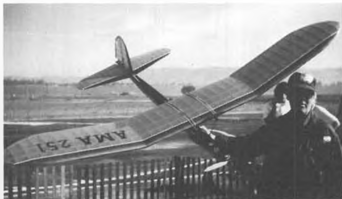
The purists can't complain about R/C in this 1937 Lanzo R/C Stick, with builder John "Daddy Warbucks" Pond. Merco 49 ignition.
