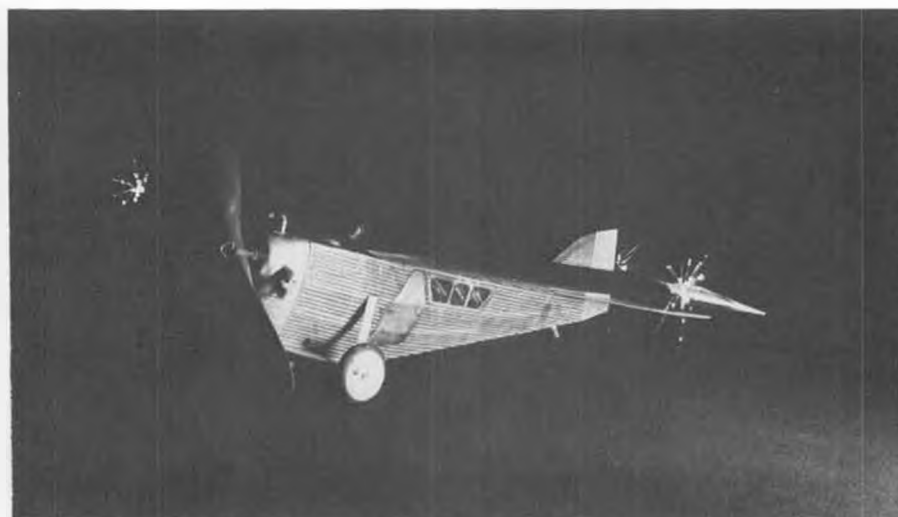
All ready for a night flight! This side lighted photo shows off the simulated corrugated metal skin of the ANT-2. Walt drew ball-point ink lines on covering tissue before applying.
