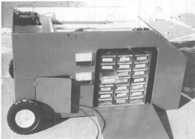
The author's portable pit box. Note the ammeters for two starting batteries. Two 6-volt packs in recessed top for electric starter.
