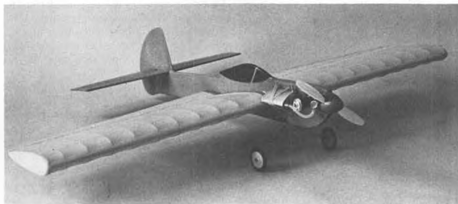
Boyd scaled down a Dick Mathis "Excaliber" to 32 inches for this one. Weight is 10.5 ounces. John is from Sioux Falls, South Dakota.
