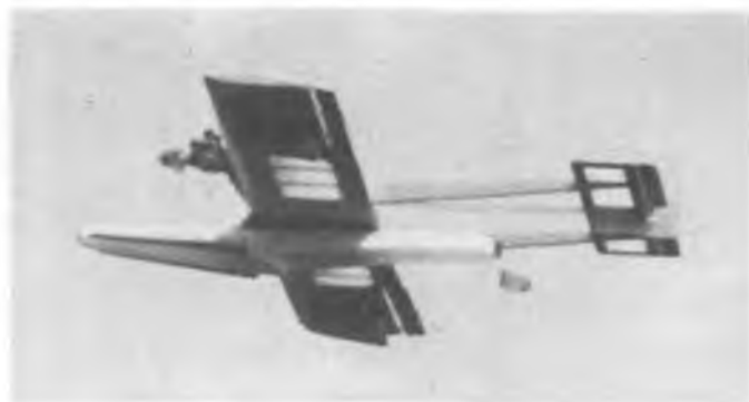
Telephoto shot of Sealander I in flight. Float is 33 inch Gee Bee molded from tough plastic.
