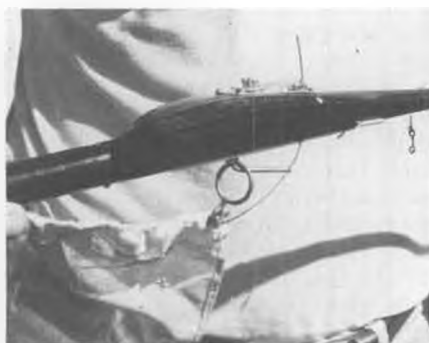
Wire from tow-line releases DT timer when glider is released. Auto-rudder link at right.
