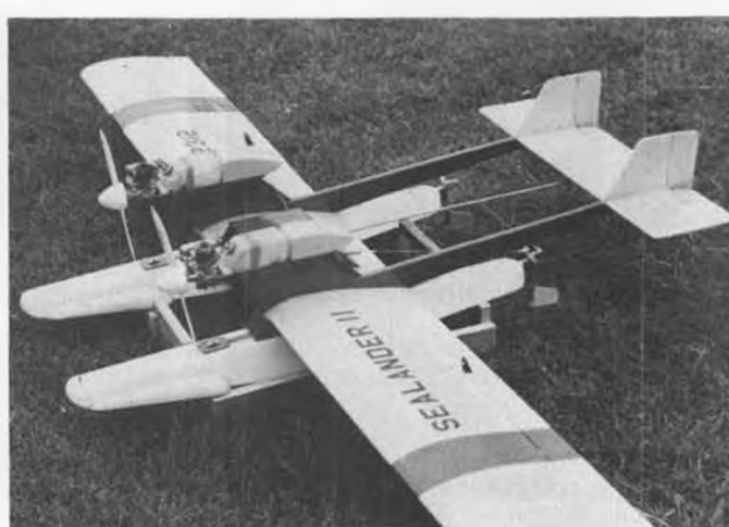
Both Sealanders have sponsons added to the floats. Lowers water-line and also deflects water spray away from props.
