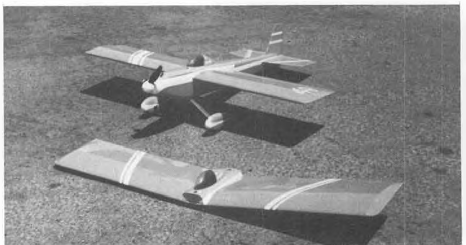
With two wings available, this little Half-A'er "doubles" as a competition (racer) and sport model. Sport wing has dihedral . . . no ailerons.
