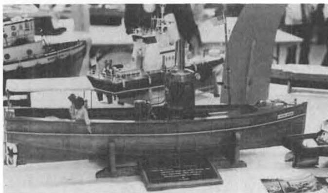
G. Miller scratch-built this African Queen from photographs. Steam engine machined from castings, other parts handmade. Radio control.
