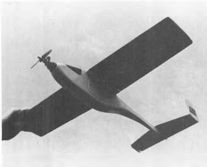
Bob Aberle has revised his Li'l Eaglet to use twin rudder set-up. He says this and the original inverted V-tail work about the same.
