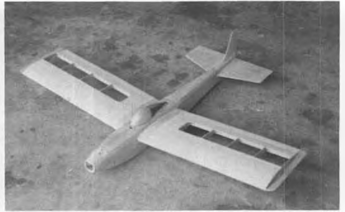
At the bare structure stage, we see the Dublr with both wings being fitted. You can build just one or the other, or set it up to make use of both.
