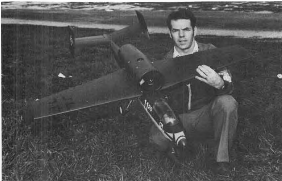
Nick Zirola, with his HE-162 Heinkel, kitted by Midwest Products. It uses the Midwest Axiflo RK-40 ducted fan kit for motivation.
