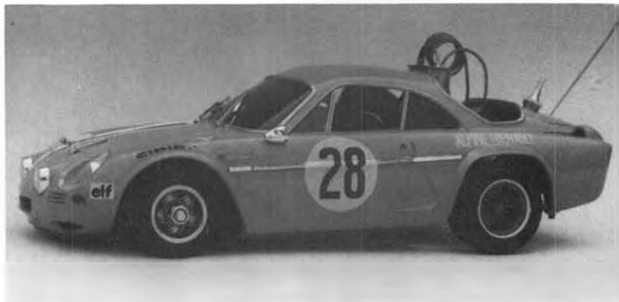
The CO 2 cylinders sticking out of Suzuki's little R/C Renault are reminiscent of World War II Europe, when many cars carried propane fuel tanks on their backs because of gas shortage.
