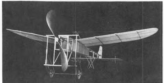
Sherman Gillespie constructed and photographed this classic Bleriot, from Ideal plans. Note the "motor stick", popular in early models.
