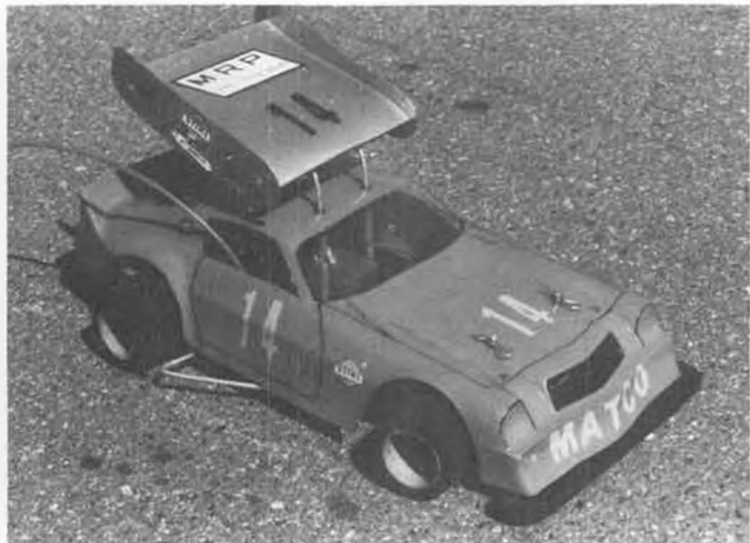
Matt Vuolo's 1/8 scale R/C version of a 1-1 scale modified (!) stock that he raced. Wing has inverted airfoil.
