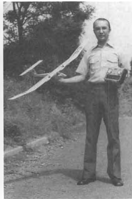
Here's Masayuki with his OS R/C guided CO 2 powered glider. Span is 1100 mm.
