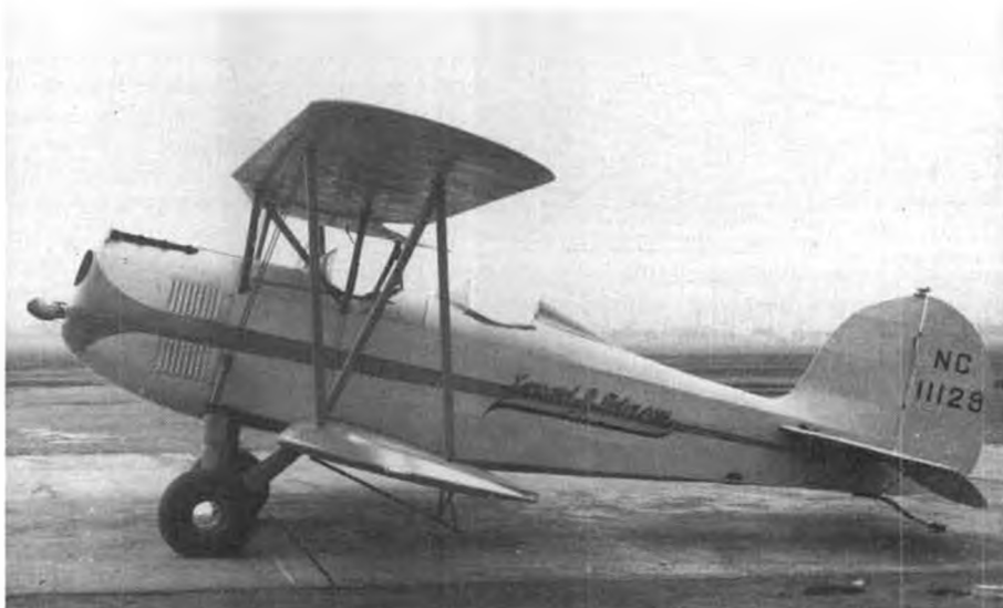
Just to confuse things, the 1931 GLT, with larger fin/rudder and rounded cowling, was still called the 2T-1A. Performance was not as good as earlier model. Note trainer wing skid.
