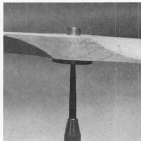
The "Biso Balancer", another device from Harry Higley. Hmmm . . . also balances props!
