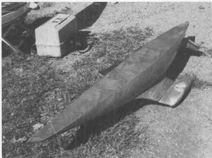
Former AMYA A-Class Sec., Ed Williams, built this A-boat. Note hard chine, diagonal planking. Lead shoe removable for transport.
