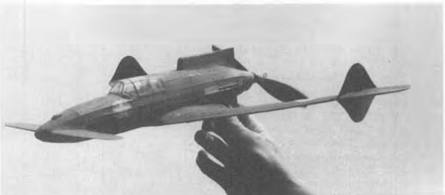
Some purists maintain that the XP-55 wasn't a true canard, but rather, a flying wing with a forward control surface. Picky, picky, picky . . .
