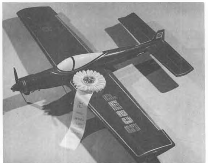
The author's Half-A stunter, which placed 3rd in that category at the 1977 MAC show. Note flaps, adjustable lead-out positioning.
