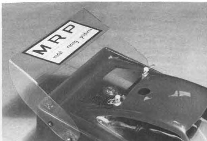
Wing is formed from .030 Lexan. Can be made adjustable by slotting rear hole on each side.
