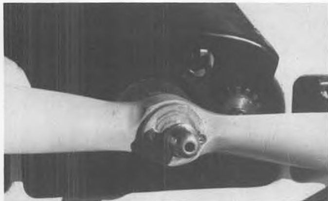
Two photos of Hanno Prettnner's power system. Geared prop (2 to 1) driven counterclockwise by two clockwise-running Webra 61's. Worked faultlessly for all practice and official flights. Further description in text. Interesting arrangement!
