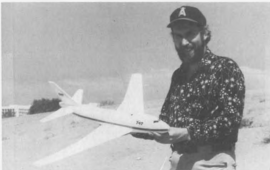
Talk about different! John Veale, of Manhattan Beach, California, converted this all-foam free flight 747 into an R/C slope glider. Uses Kraft radio with KPS-18 servos, weighs less than 10 oz.
