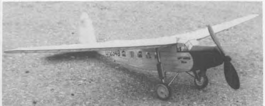
Bill Noonan's big rubber-powered Messerschmitt 20B spans 52 inches, is bigger than it looks in this photo. Bill hand carved all 10 of the model's occupants.
