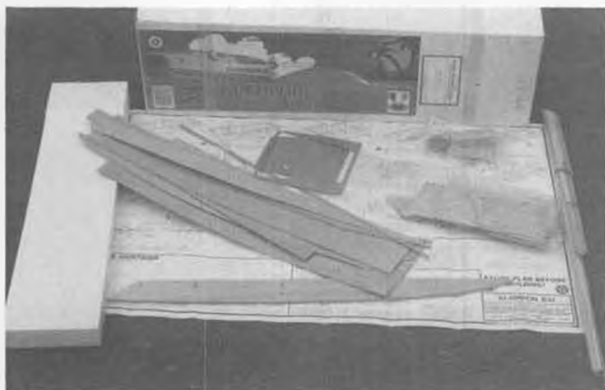
Kit contents. Foam building jig on the right is very helpful for maintaining alignment of the hull during construction.
