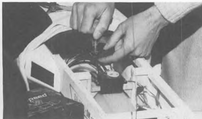
Hanno's only mechanical failure! Nut holding hatch hold-down bolt came loose. Re-epoxied after one flight with rubber band hood strap!
