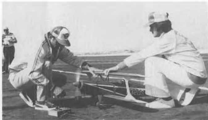
Norm Cassella fires up Webra .91 with O.S. .61 carb in his own kit Steen Skybolt. 15x5 prop, Kraft radio. Donohue holds.
