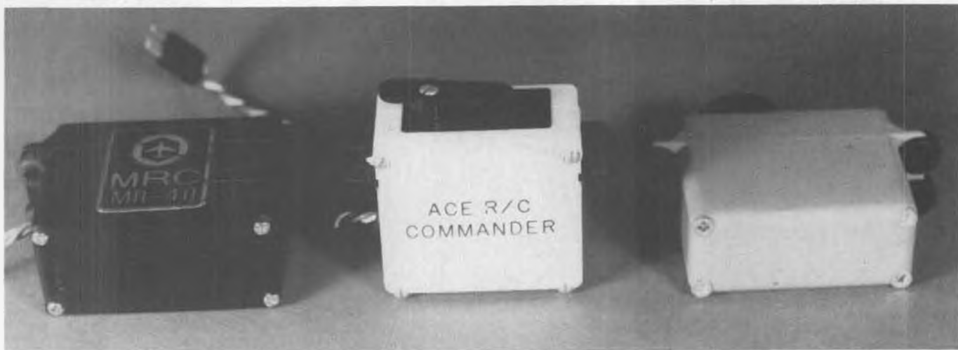
The first step (after reading the instructions through) in reversing servo rotation is to disassemble the case. Shown above are three miscellaneous servos showing the screws to remove. From left to right, MRC, Ace Bantam, and Kraft KPS-14.
