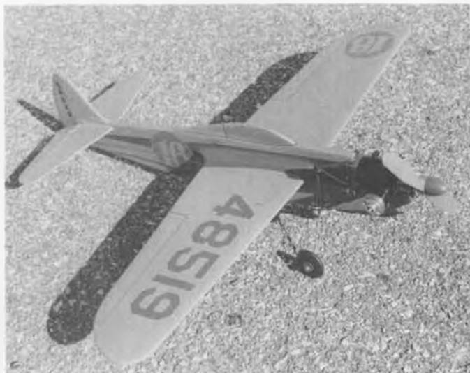
Dave's Shoestring with the flight landing gear installed. Note that the fuselage extension over the engine has broken off.
