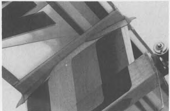
Closeup of Bob's Maverick, showing how he made the wing hold-downs. Fully described in text.
