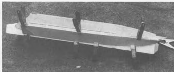
Clamps are used to hold the sponson sides to the basic framework, still on the foam jig.
