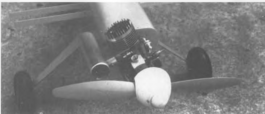
Prototype Gross Vogel uses an Enya .60, which is more than enough power. Engine is angled to one side to provide clearance for muffler.
