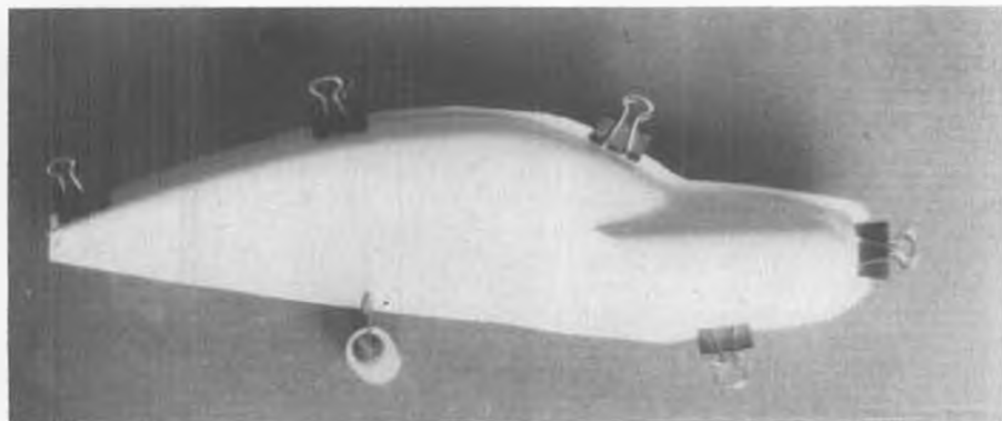
Gluing the plastic cowl halves together. Cutouts for wing and fuselage are made later. Use of spring clips from stationary store is a clever way to hold pieces while the glue dries.
