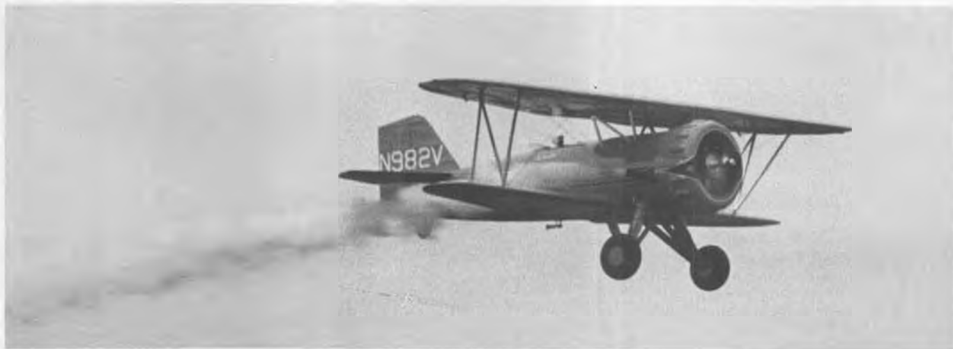
Beautiful action shot of Kirby Crawford's Curtiss Gulfhawk, recently flown at D.C. meet. Kirby did his own conversion on a Homelite chainsaw engine, does a good job of pulling the 27-pound model through a realistic aerobatic routine. Model is not quite 1/4 scale. Photo by John Preston.
