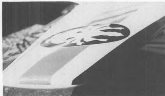
Sneaky stall strip blended into tip leading edge of CAP 20 L by Jeff Tracy, Australia. Maintained scale outline of aircraft, and legal.
