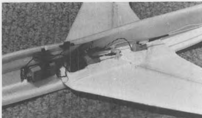
Closeup of the radio installation in John's 747. Ailerons are driven by torque rods set into the top surface of the wing.
