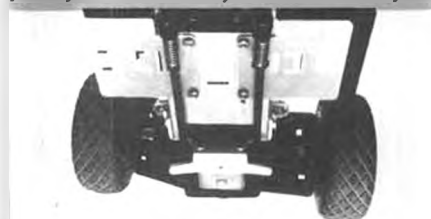
Actual torsion bar suspension system along with operating, independent wishbone suspension on each wheel help you run on uneven terrain
