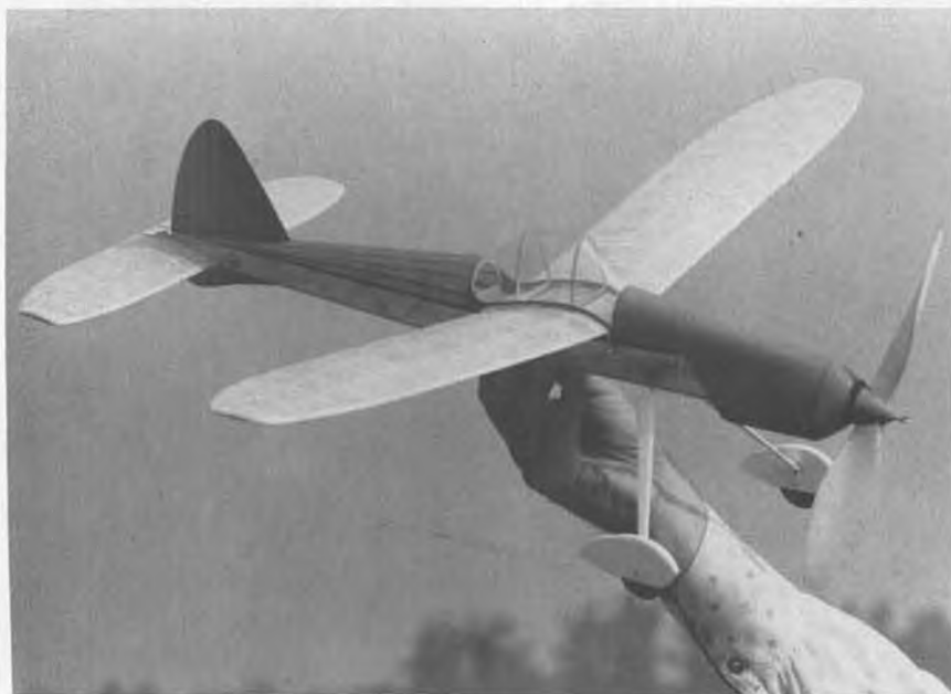
"Stormhawk" is one of the most realistic looking sport rubber models we've seen in quite a while. Wheel pants, unusual cowl, and eye-catching canopy are trademarks of the design.
