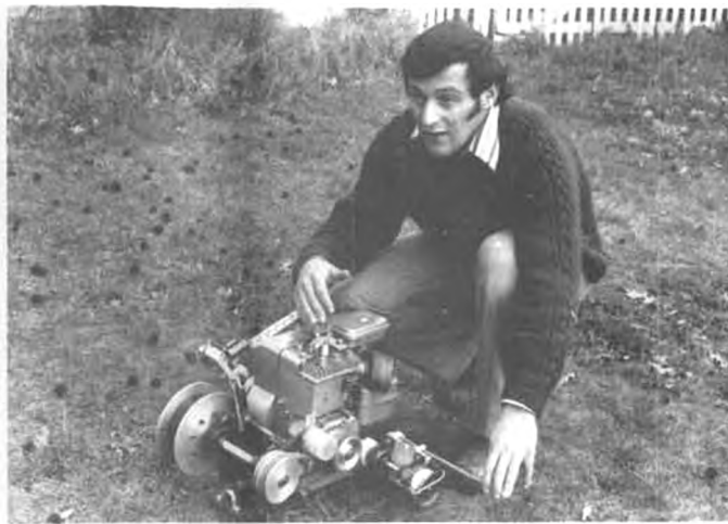
Ralph Learmont and his Launch Master winch. Also included is a line retrieval system that brings the towhook back to the winch.
