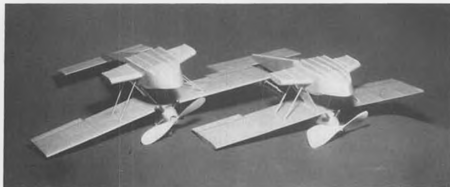
Hull and sponson strakes are added after the hull has been covered and doped. Celluloid air-flow straightener between front and 2nd cabane struts is just barely visible on model on right.
