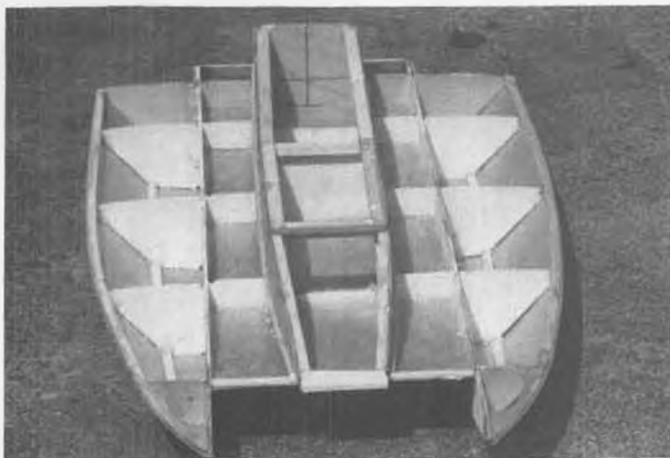
Front view of the deck, showing the cockpit and radio compartment.
