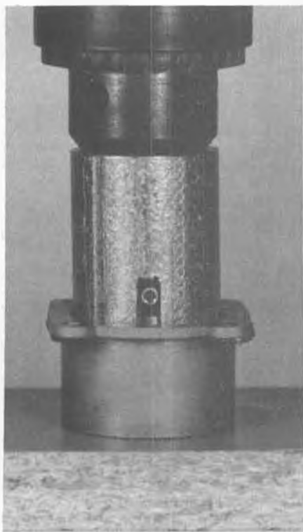
Pressing the pump-equipped backplate into the Webra backplate. Drill press is being used as a press. Note pressboard block between backplates and drill press table.
