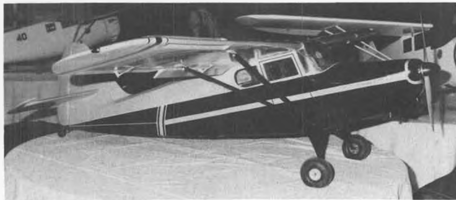
Stinson Voyager by Chris Evans, of Loomis, Ca., was flown at Las Vegas 1/4-scale Fun Fly. Built from Sid Morgan plans, 9' span, 20 lbs., Quadra engine. Low stall speed with flaps down.
