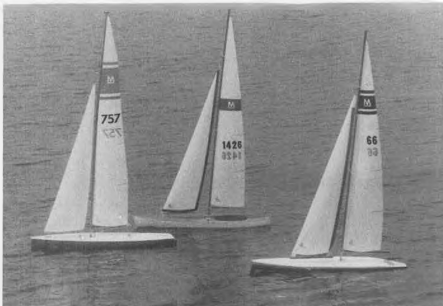
From left to right, the BINGO, EPIC, and new BONE design discussed in text. Note how the free foredeck area is increasing as the rig moves aft.
