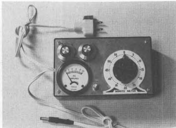
Portable charger from parts in photo at left. Uses regular 115 V plug, color coded with tape for positive and negative leads.
