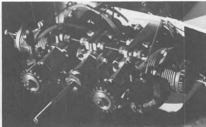
Two photos of Hanno Prettnner's power system. Geared prop (2 to 1) driven counterclockwise by two clockwise-running Webra 61's. Worked faultlessly for all practice and official flights. Further description in text. Interesting arrangement!
