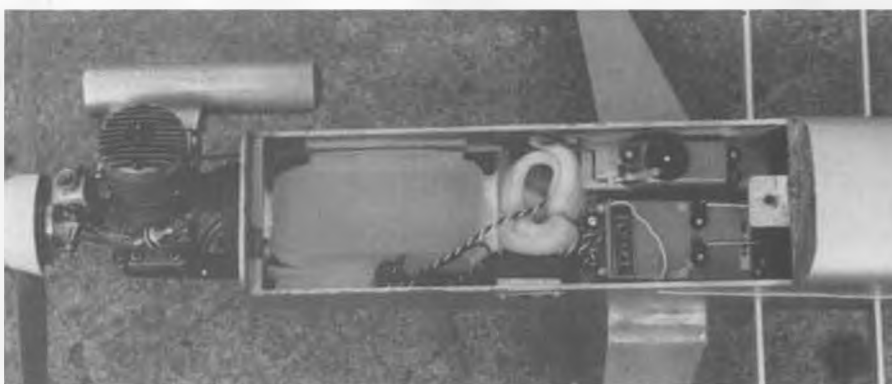
Good closeup shot of the engine and radio installation. Most of the top of the fuselage is removable for access to the tank, radio, and control linkages.
