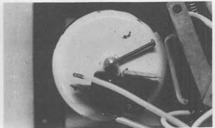
Closeup of back of timer in photo at bottom of p. 66. Note how long bolt in wheel collar on timer shaft will activate switch lever.
