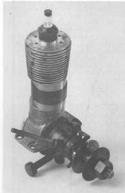
Otto Bernhardt's 3rd homebuilt engine, built about 1937. Inspired by the Baby Cyclone, it features a sand cast aluminum crankcase and bypass cover held in place with copper wire.
