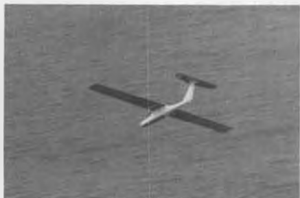
Sequence of photos of John Lupperger's Ridge Runt making a close pass at Torrey Pines. Model has a 49-inch wing with a 10% flat bottom airfoil. Really moves out at 9 oz./sq. ft.
