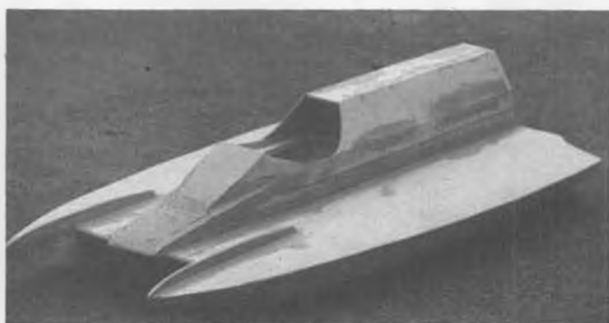
Basic hull with rear cowling in place and body putty in all joints and seams.
