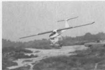
Sequence of photos of John Lupperger's Ridge Runt making a close pass at Torrey Pines. Model has a 49-inch wing with a 10% flat bottom airfoil. Really moves out at 9 oz./sq. ft.
