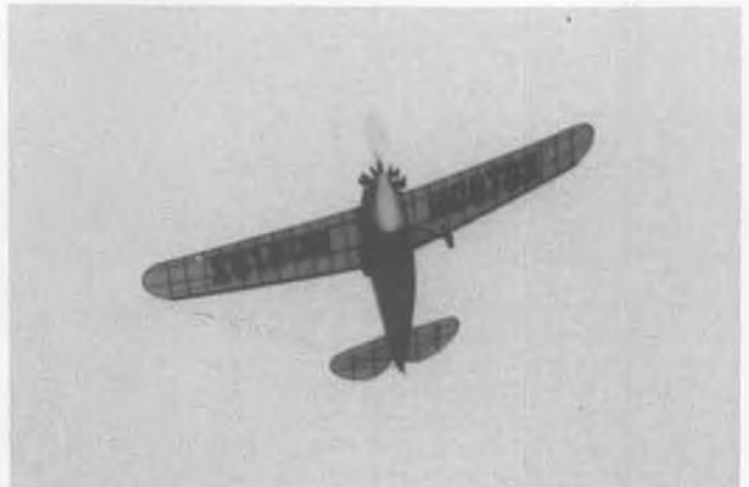
Cliff's Cessna AW in flight. Model was designed when the minimum span for Jumbo Scale was 48", since reduced to 36".
