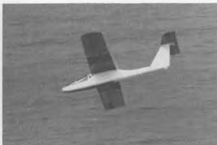
Sequence of photos of John Lupperger's Ridge Runt making a close pass at Torrey Pines. Model has a 49-inch wing with a 10% flat bottom airfoil. Really moves out at 9 oz./sq. ft.
