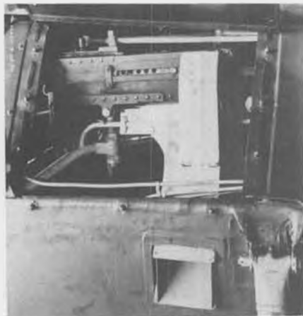
On military Fledglings, a single fixed .30 caliber Browning was installed on the right side ahead of pilot. A Lewis gun on a Scarff ring was also carried for gunnery training.
