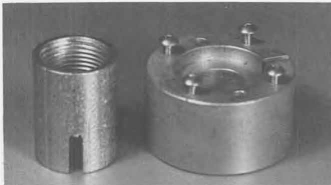
Jigs required. The piece on the left is a press-in adapter, the other is used to hold the Webra backplate during machining.
