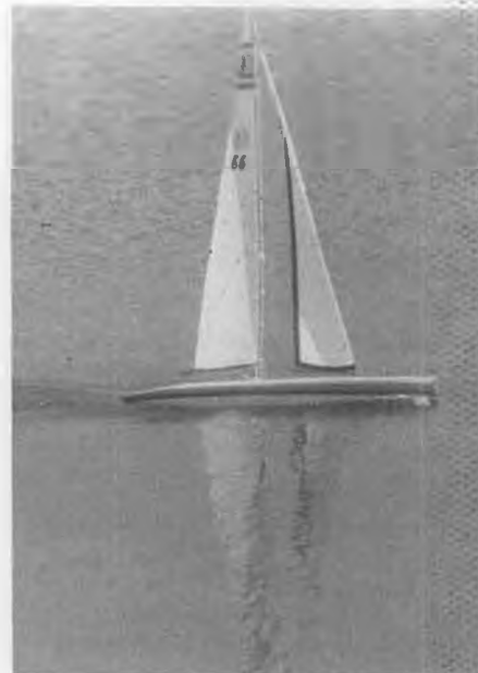
BONE on a reach. Note the excessive amount of twist in the jib.
