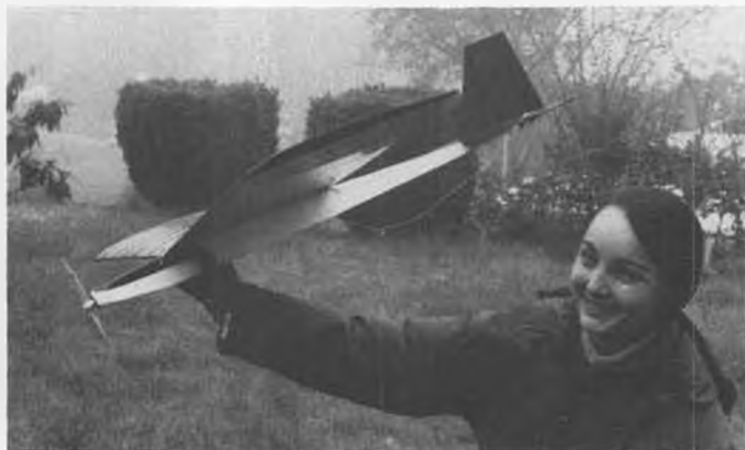
Two views of Mitch Poling's "Astro Dandy", designed and built especially for the Indoor R/C Record Trials to be held at the IMS Show. Sandra Smith Poling, M.D., is the better looking model in the photo. Astro Dandy has 4 sq. ft. wing area, weighs 16 oz. without motor on-off servo.
