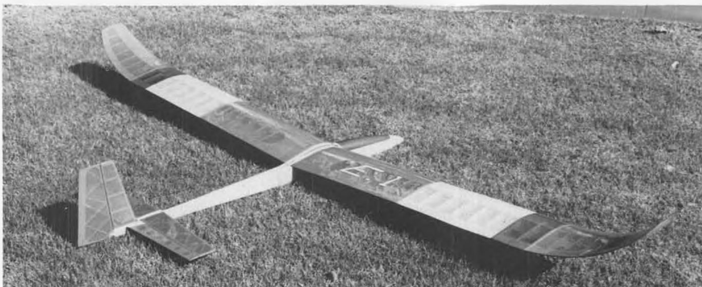
Herb Semmelmeier's beautiful "Elliptical" multi-task FAI design, featured as a 3-view on page 50. The model shown here was built by Harry Menke, of Santa Rosa, and was flown in the 1976 LSF Tournament held there. Model has a 117-inch span, 1046 sq. in. area.
