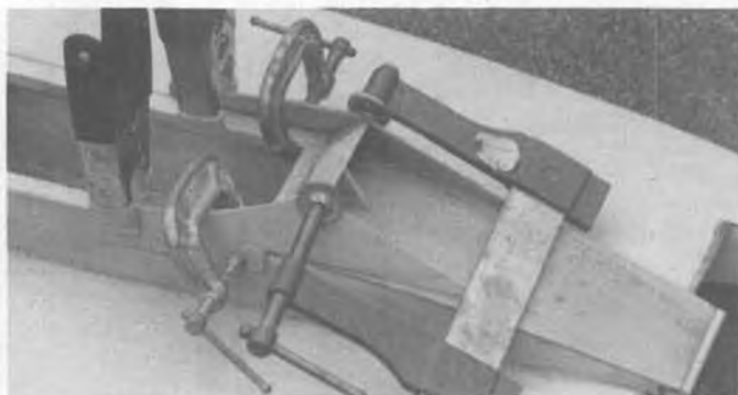
All kinds of clamps being used to hold the cockpit cowling in position. Remember, this is not the stock cowling.
