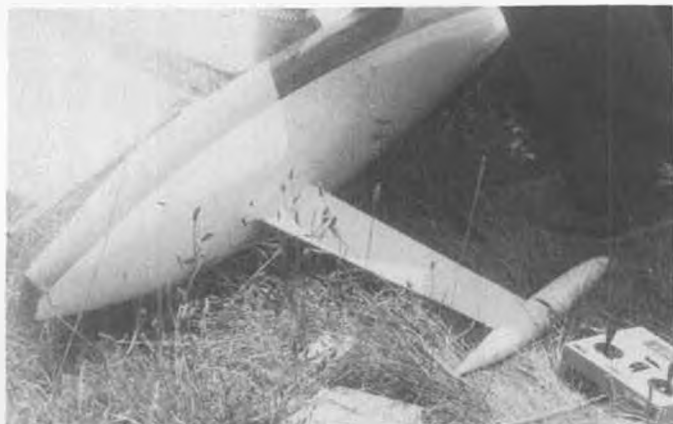
Transom of BONE is only 1-1/2" deep. Center of Gravity of the whole system is 6" below waterline. Hey! Where's the rudder?
