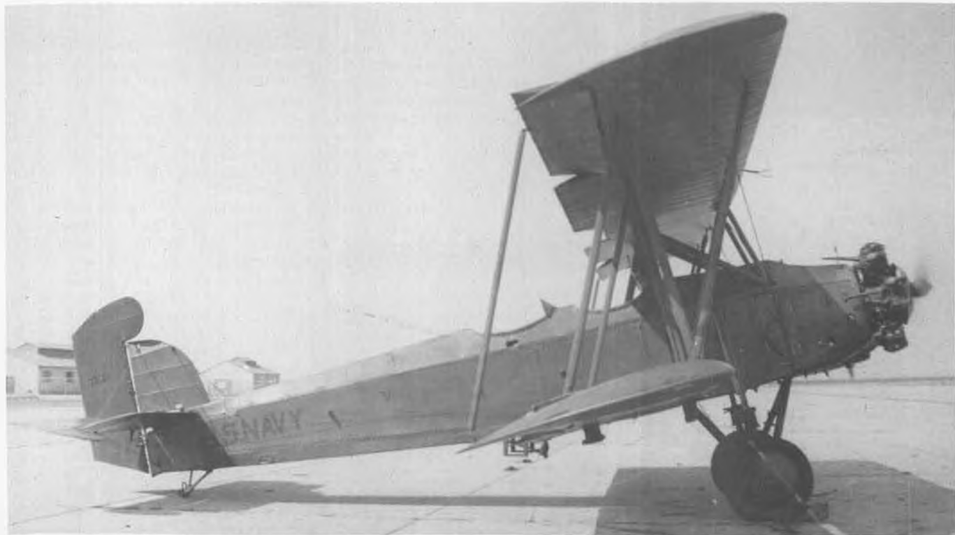
Both XN2C-1's and N2C-1's were powered by the 9-cylinder Wright Whirlwind J-5. Bomb sight and bomb rack fittings have been installed on the all-yellow trainer, but the tail stripes and serial number are missing. Pete Bowers photo.
