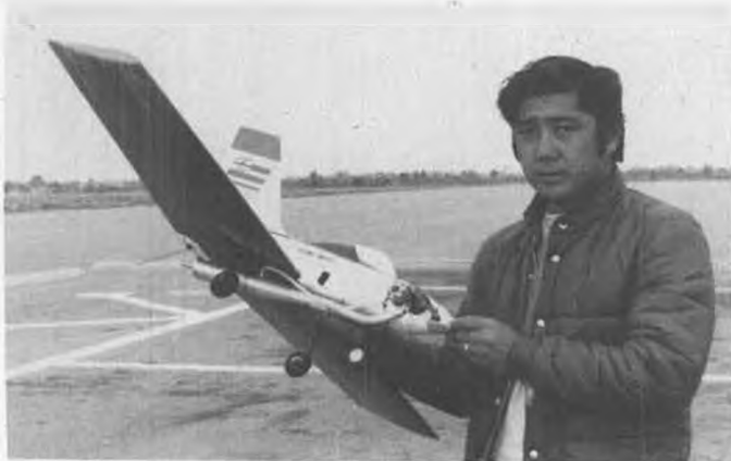
Wayne Sakamoto placed 2nd in R/C Power with his Evans "540" design. Uses .40 size engine with tuned pipe. Fast!
