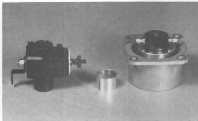
All the new components ready to be installed. Sleeve is required to install the .61 carb into the .91 case.
