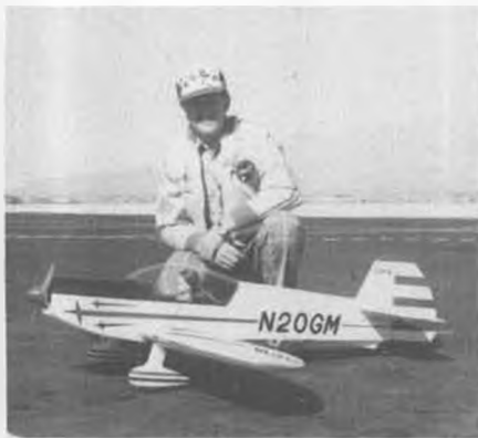
Ivan Kristensen, own CAP 10b, Webra .91, Perry Pump, MD 14x6, Solarfilm, Pro Line.
