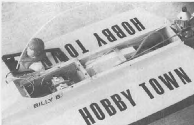
Radio, fuel tank, and engine installation in the Klampon Kai that the author built for Bill Brazzle.
