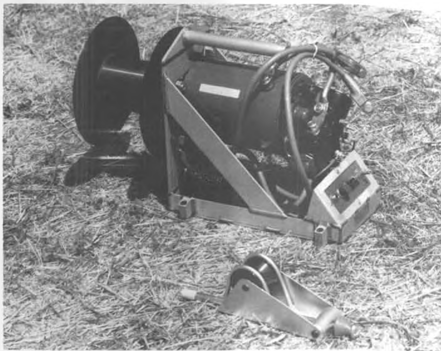
Sturdy, well-built electric winch by Bill Amour, of Torrance, California, will operate on either 6 or 12 volts. Cost is $185, excluding the battery and nylon towline.
