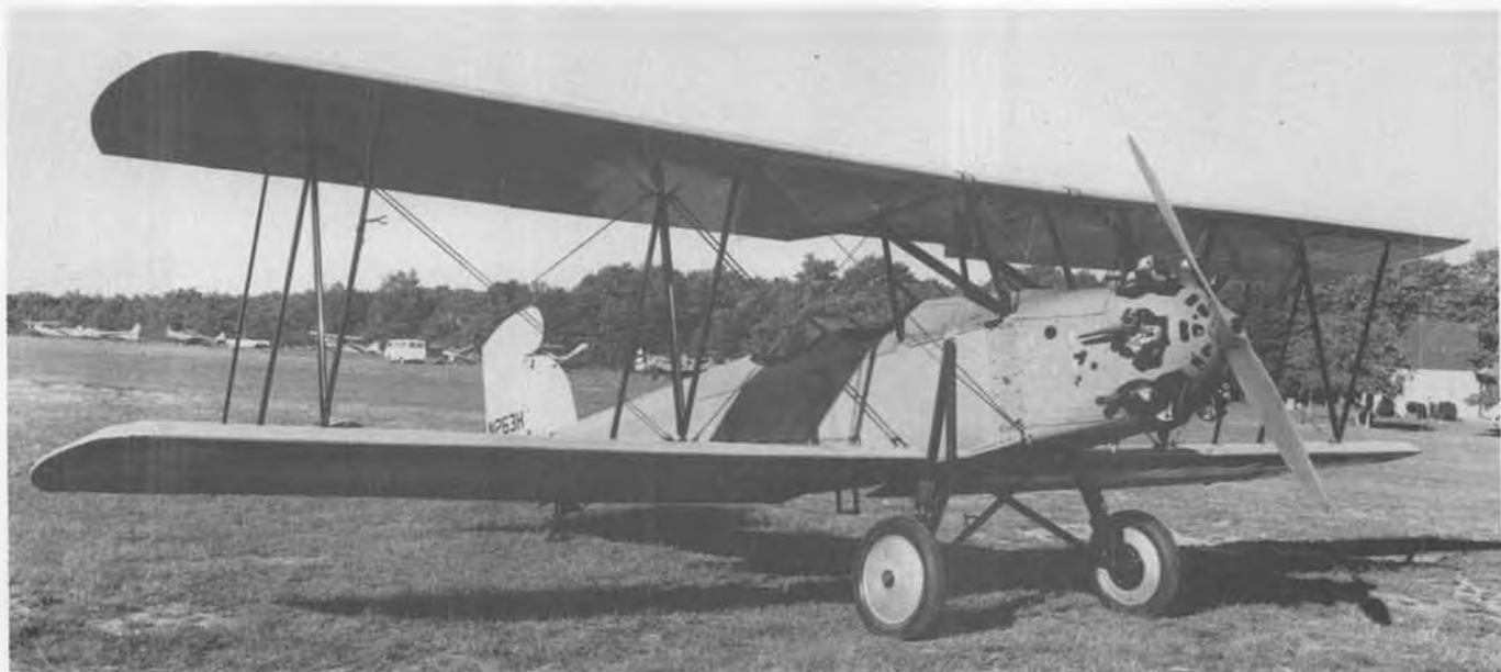
Antique Grand Champion of the 1966 Antique Aircraft Association fly-in was N263H, a Fledgling restored by Joe Erales. Restoration is authentic down to the Challenger engine and forged Curtiss-Reed prop. Airplane is now in a museum in Rio De Janiero. Warren Shipp photo.
