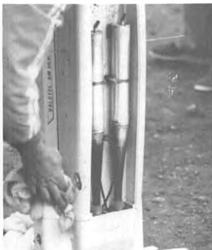
Twin tuned pipes in bottom of Prettner's Dalotel DM-165. Tubes lead to prop bearings.
