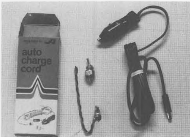
Astro Flight charge cord that connects in auto cigarette lighter. Doesn't have timer, so don't forget to unplug after 15 minutes!
