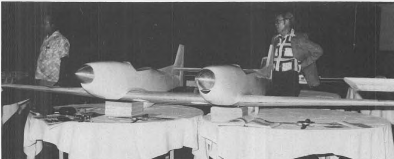
What not to build for 1/4-scale. This 12'10", 55-lb. F-82 Twin Mustang, being built by John Simone and Frank Johnson, is a good example of what the 1/4-scale movement could lead to unless some upper limits are placed on engine size, wing loading, and total weight.
