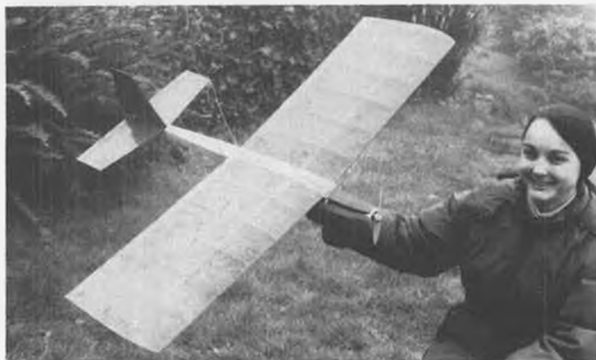
Two views of Mitch Poling's "Astro Dandy", designed and built especially for the Indoor R/C Record Trials to be held at the IMS Show. Sandra Smith Poling, M.D., is the better looking model in the photo. Astro Dandy has 4 sq. ft. wing area, weighs 16 oz. without motor on-off servo.
