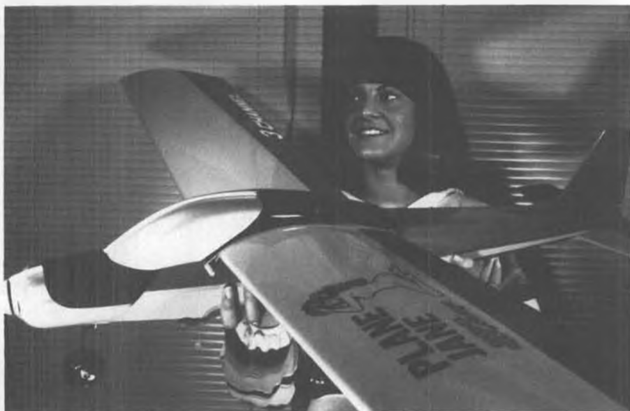
Lovely Denise Viosca with Charlie's Plane Jane. Kit is highly prefabricated, comes with pre-built and sheeted wings, pre-built fuselage and tail surfaces. Takes a .15 to .25 size engine.
