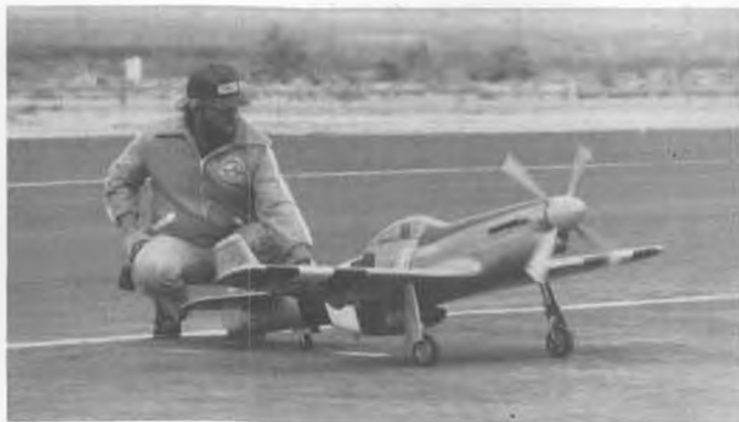
Impressive P-51 with belt-reduction driven 4-blade prop, .61 power. A prototype for Byron Originals kit. Smooth flier.
