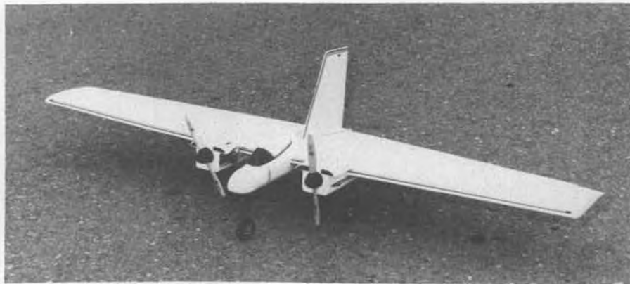
"Scimitar", by Bill Evans. Powered by two K&B .19's with individual throttles, uses five channels of radio, one for nose wheel only.
