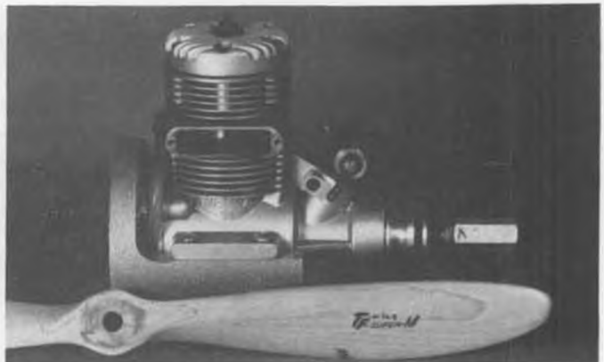
Pump-equipped .91 installed in CB Enterprises' new CB .90 engine mount. Engine runs better than ever.
