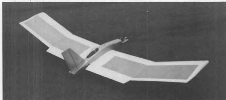
Gross Vogel before the lettering and trim had been applied. Model is very stable in the air, requires careful ground handling when wind is blowing to avoid ground looping.
