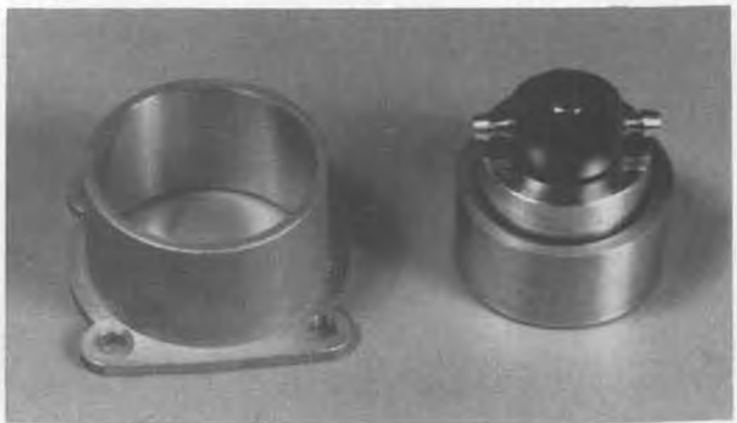
Machined backplate components ready to be pressed together. Procedure is explained in text.
