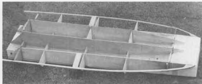
The framework on the foam building jig. Map tacks work well in holding the framework to the jig.
