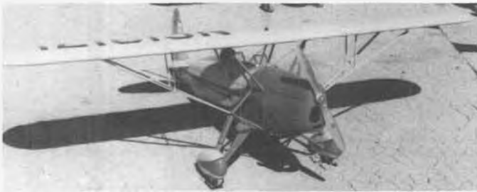
Best Scale entry, Fairchild 22 by George Harlan, Irvine, Calif., 22, lbs., McCulloch engine, 98-1/2" span, not yet flown.
