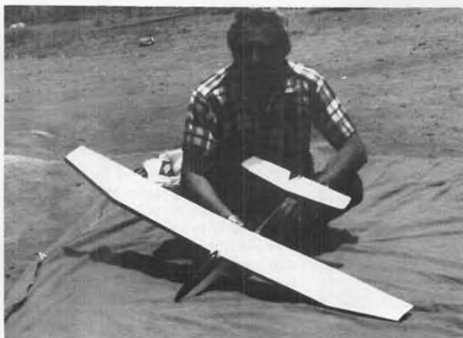
Al Bendet's as yet unnamed one-meter bird follows more closely the layout of conventional thermal sailplanes than the model at the top of the page. Photo at left shows how it all comes apart for easy transport. Can also fly without the plug-in tip panels.
