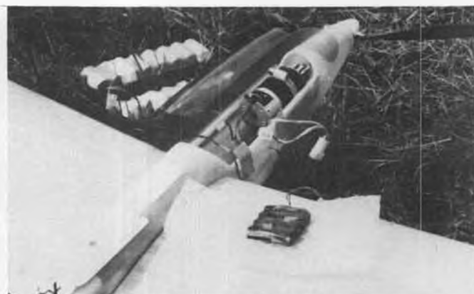
Motor and battery installation in Bremer's TW. Motor is a Keller (as were most) 50/24 with 24 cells, turning a 13X9 folding prop. Span of the model is 100 inches, weighs 6 lbs.
