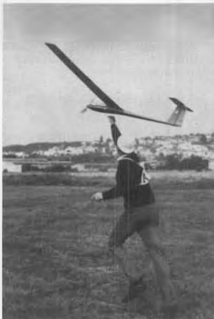
Robbe Diamant placed 6th in FAI for Karl Stroher, used E-Max motor with 16 cells, turned a 16X10 folding prop.
