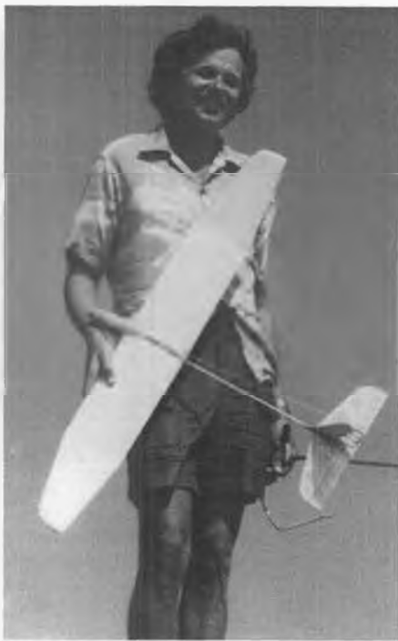
Noel Jones (left) and buddy Jack Chambers collaborated on this neat one-meter sailplane, actually little more than a scaled-up F/F HLG. Weight is only 10 oz. Should be great for R/C HLG events.
