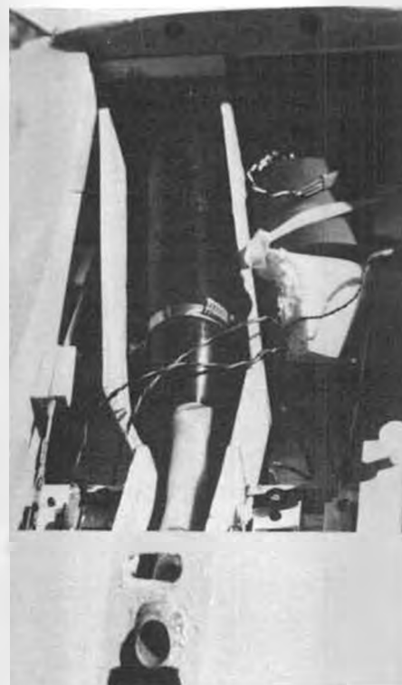
Tuned pipe runs back through fuselage, exits aft of lower wing. Ducting around pipe is necessary for channelling cooling air and also to protect radio from excess heat.
