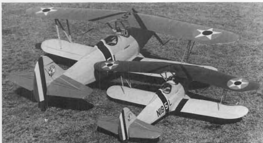
The author's biggie, all 93 inches of it, poses with his smaller 2'=1' scale (57 inch span) Sig Liberty Sport. Surprisingly, both are powered by HP .61's . . . shows what a belt drive can do.
