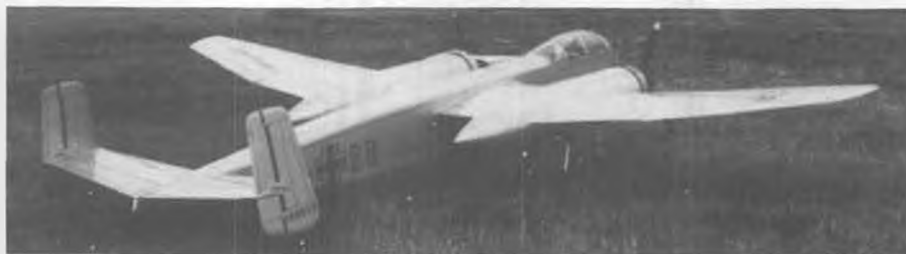
The Electroflight Champs included an event for Electric Scale, one of the entries in which was this HE-219 night fighter by Aloys Zimmerman. Two Keller motors, 46 (!) 1.2 Ah cells.
