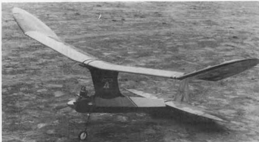
Photo No. 2. John Pond's Parmenter "Swoose" uses Orwick .64 and shielded Ace radio system. That 50% tail makes it a real floater!
