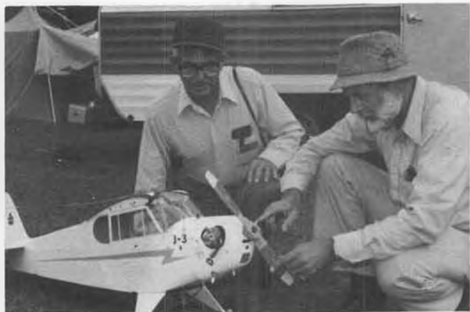
Bill Pinckard (right) explains the finer points of his 1/4-scale J-3 Cub to Joe Laberge. O.S. 120 Gemini twin is fitted with a 77 Products ignition system and distributor.
