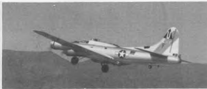
B-17G is modeled after Confederate Air Force "Sentimental Journey", weighs 50 lbs, uses 4 K&B 61's. Simprop radio.
