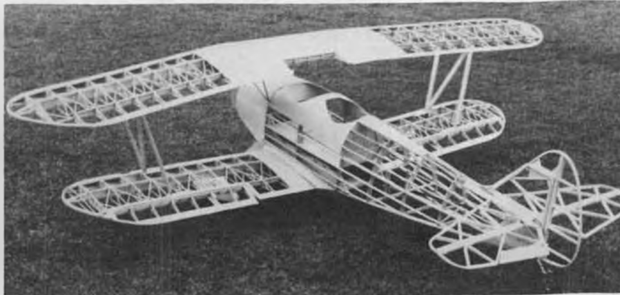
Completed structure shows very light construction. Ready-to-fly weight is just 18-1/2 lbs., with on-board plug battery and smoke system. Some beef-up required for chainsaw type engines.
