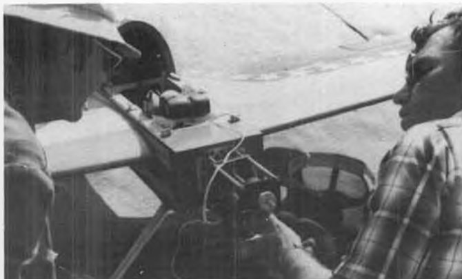
Jim Cline, studies his product, the Master Climb reduction unit, on Dean Koger's Laser. Note extra cooling head on Dean's engine.
