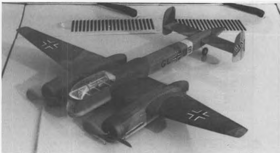
Fernando Ramos's Arado 240 is unusual for a rubber twin, in that the props are not counter-rotating to cancel torque. Best time to date: 26 sec. He plans to build another, lighter version.
