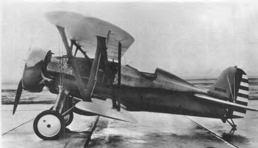
PR photo of the first production P-12E. "BOEING" on fin was removed before delivery. Bulkhead aft of pilot sloped more than on F4B-3, giving Army pilots a bigger cockpit. Boeing photo.
