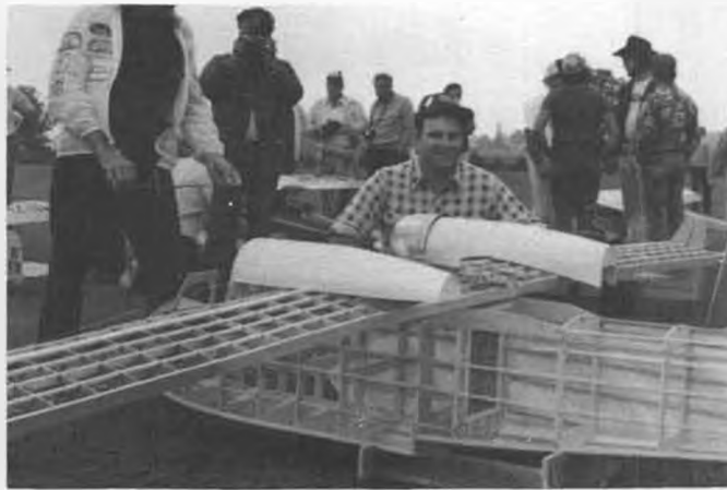
Another Canadair fire-fighter, but much larger, is this one being constructed by Rudy Mayer. Ship has 13-foot span, will be equipped with two Quadras. Unsheeted wings really droop!
