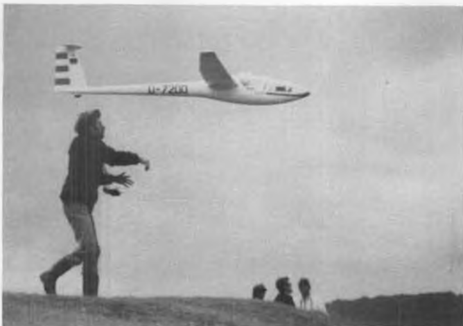
Germany's Knut Bauer is the proud designer/builder/pilot of this lovely 1/3-scale DG-200, which he flies regularly at Kirchheim-Teck. Model is apparently launched with Tx antenna only partially extended, then is fully extended after launch. Note model's VHF antenna in photo at right.
