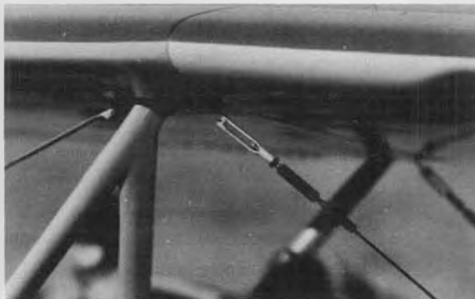
Rigging wire attachment showing the Kavan turnbuckle (could also use those made by Proctor) with Kwik-Link and lock nut.
