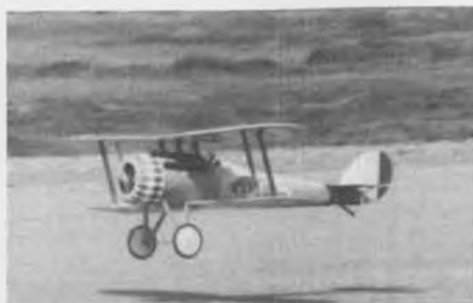
Granger Williams' Proctor 1/4-scale Nieuport 28, about to touch down on its shadow. Uses OS 90. Modified J&Z 18 x 5 adds 500 rpm.
