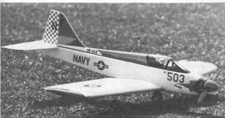
Peter Hopper (Freeville, NY) sent this picture of his Kougat. It is powered by a S.T. 46 and his Goldberg retracts. He wrote, "This is my second Kougat and have over 100 flights logged. I copied the Navy color scheme from an A-4 carrier fighter that I saw at a full scale airshow last summer. This is my favorite sport RC aircraft and I plan to always keep a Kougat around to demonstrate aerobatic flight."
