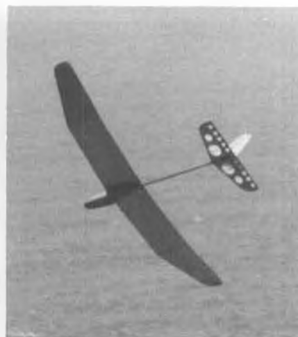
Noel Jones (left) and buddy Jack Chambers collaborated on this neat one-meter sailplane, actually little more than a scaled-up F/F HLG. Weight is only 10 oz. Should be great for R/C HLG events.
