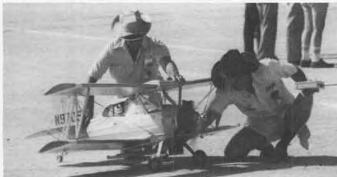
Bob Seigelkoff tunes the Kawasaki engine in his Grumman Ag Cat, built from R/CMB plans. Carries twin radios, sprays powder.
