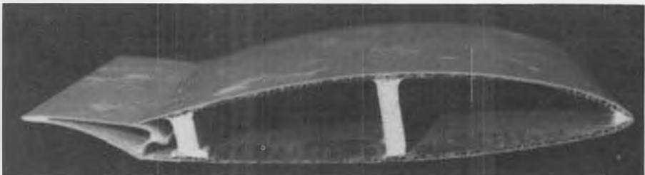
The wing section on Sommer's LS-3 and Barracuda is the Wortmann FX-62-K-131, same as on the full-scale LS-3. Cardboard liner gives the fiberglass skin extra rigidity.
