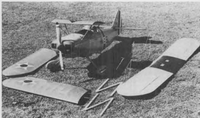
Complete model broken down for transport. Landing gear also comes off. Assembly for flying takes less than 15 minutes.
