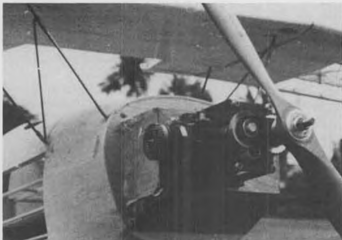
HP .61 is mounted on a DuBro belt drive unit, provides plenty of oomph for vertical maneuvers. Prop is Top Flite 20X10.
