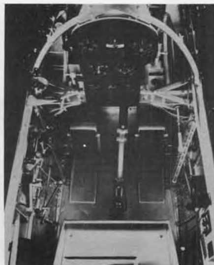
Cockpit of the P-12E was simple, with only 8 instruments to occupy the pilot's attention.
