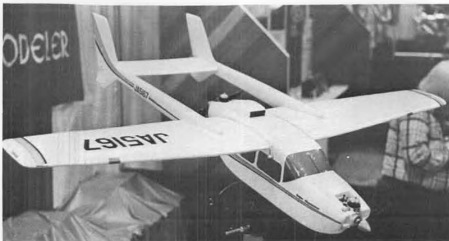
Cessna Skymaster from Airtronics, for two .049 engines. Will fly on one.
