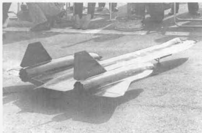
Lockheed SR-71, by Bob Gales, Hemet, CA. Two K&B 7.5s with Jet Hangar fan units. Futaba radio, not yet flown.
