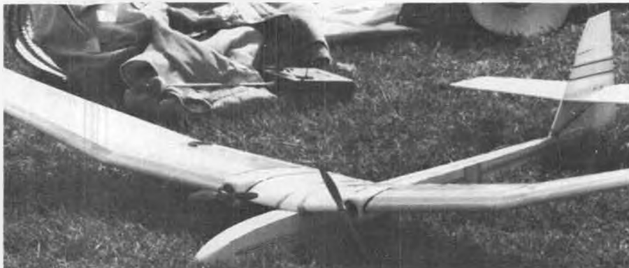
Doug Taylor's Open Class F3E is a modified Craft-Air Windrifter with two Astro 05 motors. Placed 3rd. No one-engine cuts in electric!
