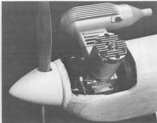
HB 40 engine bolted in place (four bolts for running, less for picture taking!). Vertical mounting simplifies starting operations.
