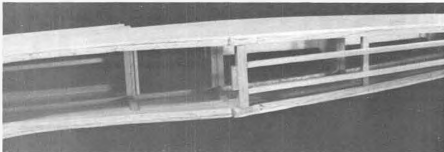
Bottom stringers butt into cross-piece at aft end of wing opening, then rest on outside of cross-pieces going back to tail post.
