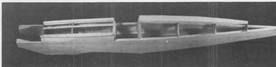
Rear deck is formed by curving, gluing, and beveling sheet backbone to bulkheads. Side pieces are then curved and glued in place prior to final shaping.
