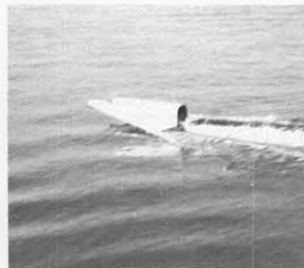
Modified Northwind, Kroker Sea-Wasp 12, 24 G.E. NiCds. Speed 35 mph plus.
