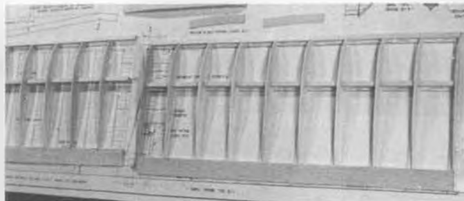
Like the rest, wing construction is simple, light, but strong. Plans show alternate aileron wing for shoulder mounting.
