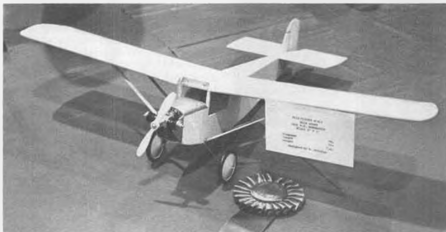
Randy Wrisley's scratch-built, one-inch scale Alco Sport free flight with Cox Pee Wee .02 engine. Second cylinder is epoxied-on dummy.
