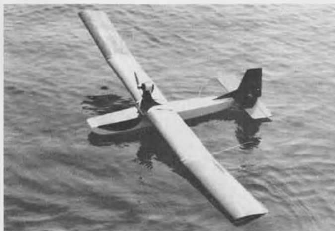
Mitch's O.D. water glider with Astro 05XL, Ace foam wings. Strictly hand launch and water landings only! Six ft. span, 44 oz.
