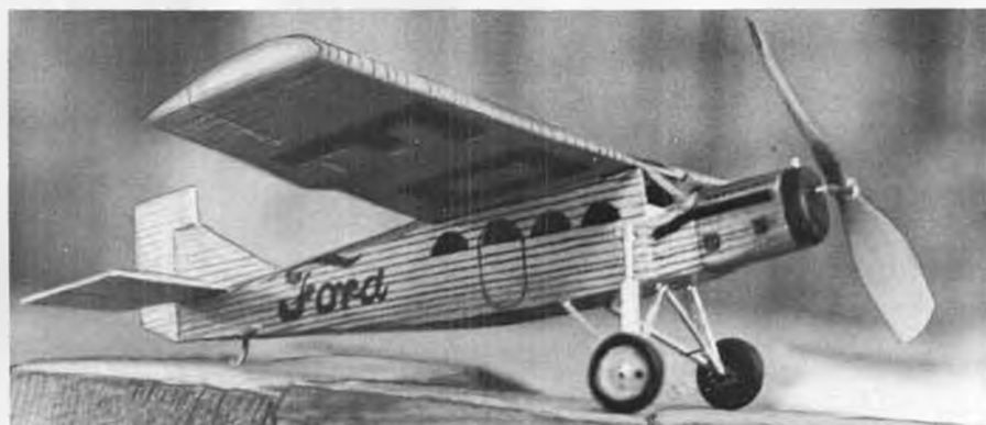
Fort 2AT Peanut by Florida's Doc Martin. Nine gram model has flown 53 seconds indoors. Silver dope over condenser paper. Dave Linstrum photo.
