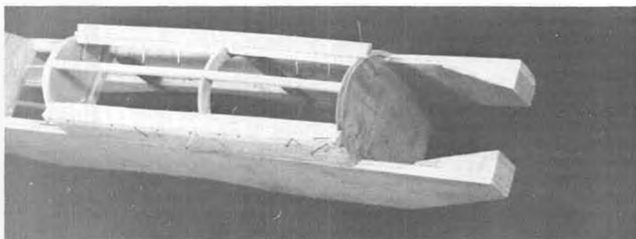
Stringers on top of fuselage forward deck provide joint backing for three planking sheets which are wet-bent formed before gluing.
