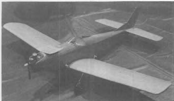
The Sterling "Lil Roughneck", oldie kit, with Cox .010 and Cannon Super Micro on rudder and elevator. Weighs 7-3/4 ozs. total.
