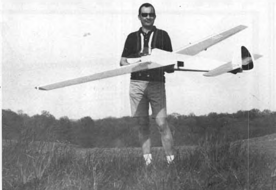
Looking back to around 1967, this was our semi-scale Schweizer 1-21 with drag brakes in the fuselage (note open door just behind wing trailing edge. Hand glides were fine, but first winch tow caused considerable damage. Still have all parts, wings have been repaired. Quadruplex radio.
