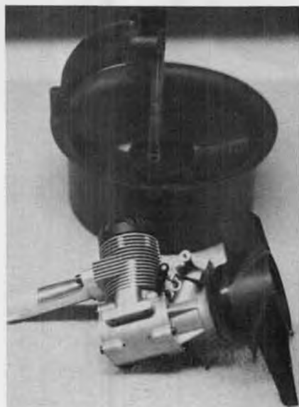
Fan and header pipe on engine. Fan shroud with engine mount in back.
