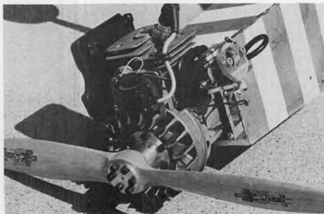
Al Willaert's "Ugly Tree" on its back for pictures. This 3.1 Whirlwind engine is very short-stroked. One flip starting.
