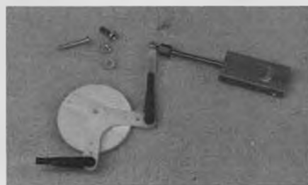
Bellcrank, links, and machined aluminum horn clamp control horizontal stab.
