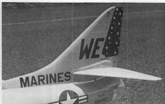
Fin, stab, and rudder detail. Note streak of light on fuselage in stab's shadow indicating small gap present.
