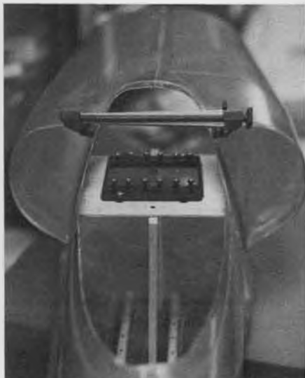
Rudder and elevator servo tray showing props between tray and fuse bottom.
