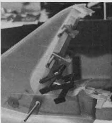
Foam fin post clamped inside fin while epoxy cures. Note bellcrank's shadow.
