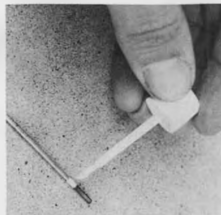
Step Two: thread with die tool, then use correction fluid to mark end of threads.
