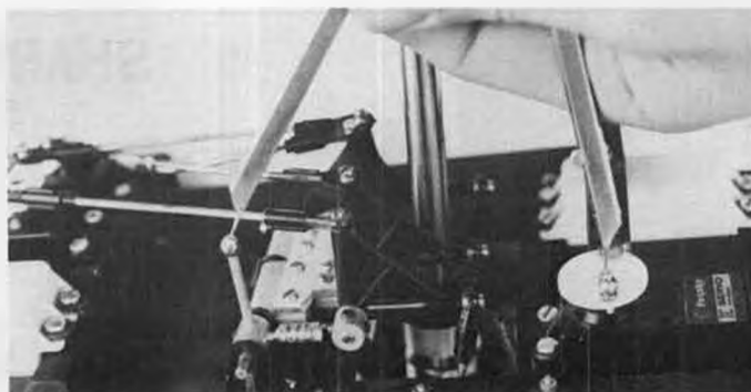
The first step in making a replacement pushrod: measure the distance from ball center to ball center with dividers.
