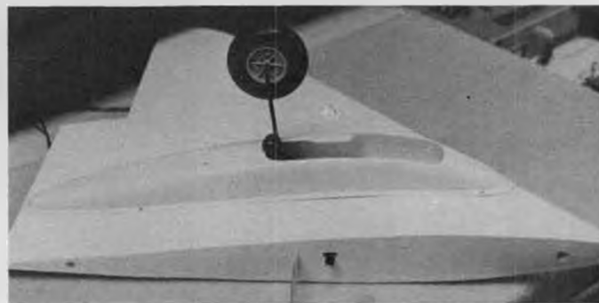
Main landing gear retracts are faired over by molded plastic fairing. Servo is buried in foam wing.
