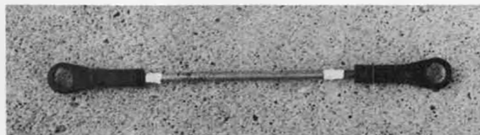
Step Four: completed pushrod. Link on left is completely screwed in. Link on right is not, to allow for adjustments.
