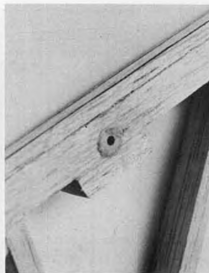
Tail surface "hard-point". Balsa drilled out for 1/4-inch dowel. 4-40 bolt hole.
