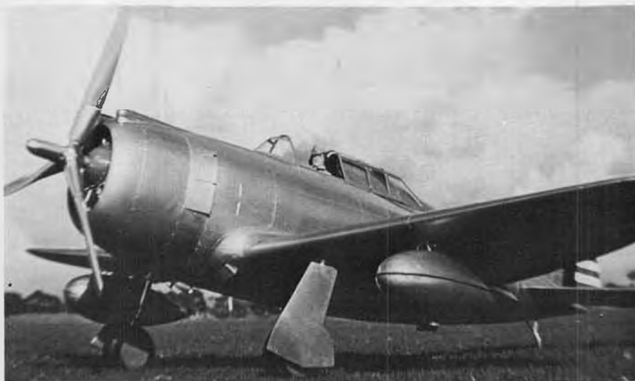
Drop tanks are early 75-gallon types. Ship weighs just 20 pounds, with Quadra engine. Model and original both flew from grass fields.
