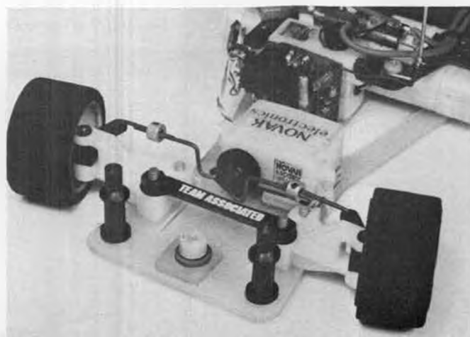
Front end of Kent's car. Note: lightened body posts, graphite cross bar, no servo saver (!), steering links on bottom of arm.
