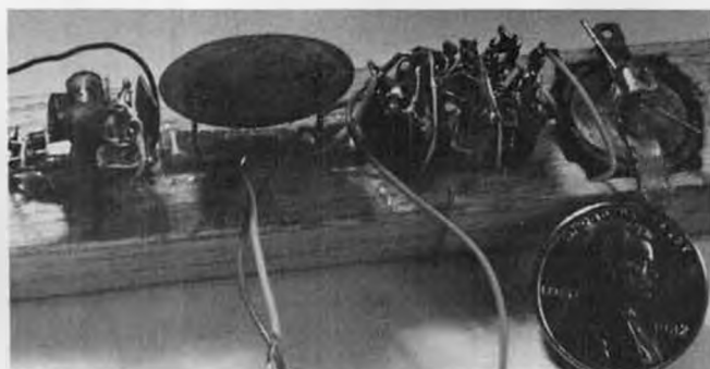
Fritz Mueller's experimental pulse receiver and actuator. Weight is a mere 27 grams including alkalines!
