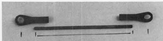
Step Three: subtract the non-threaded area of each link from the first marks. Cut rod to length, then thread it.
