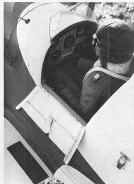
The cockpit of the Jungmeister is as finely crafted as the exterior. Note cockpit door and luggage compartment latches.
