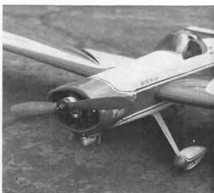
Saito 120 four-cycle, turning 15x10 Zinger cut to 14 and thinned, 15% castro, 5% nitro.
