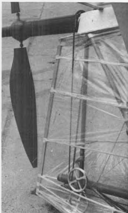
The Bionic Bat 's propeller is concentric with the tail boom. The prop's six-foot diameter is driven by a bicycle chain, does 250 rpm.
