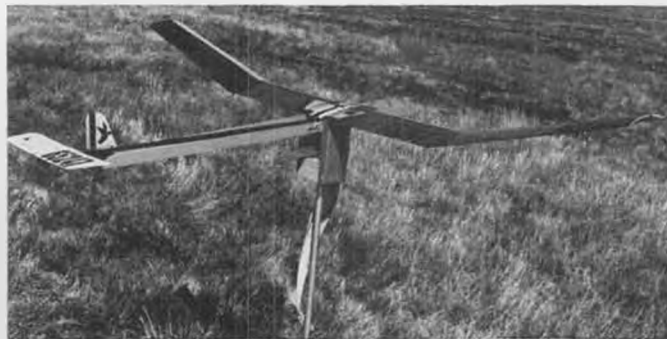
Wayne Drake uses this launching stooge for his A-2 glider, the Cold Duck No. 9. The model is supported by thin rails mounted on a support that swivels to allow launch in any direction.
