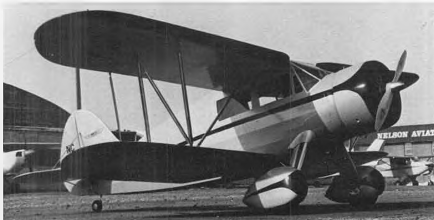
LEFT: Noal R. Hess built this super Waco YKS-6 from Bob Morse plans. At 35 pounds, it's kind of a heavyweight, which keeps the Kioritz 2.4 working hard all the time. Noal does nice work!
