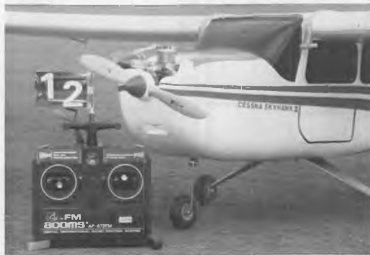
LEFT: An ACOMS FM four-channel R/C system was used for test flying the Skyhawk II. Controls used are the four normal functions, plus nosewheel steering.
