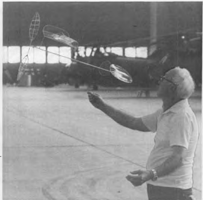
RIGHT: Earl Hoffman flies his FAI duration model. Earl's models often turn out underweight. Earl is famous for his Easy B record of 24 minutes. The prop was built-up and covered with very thin sheet wood.
