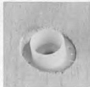
The nylon guide, in the wooden dowel, in the wing core. Use epoxy glue.
