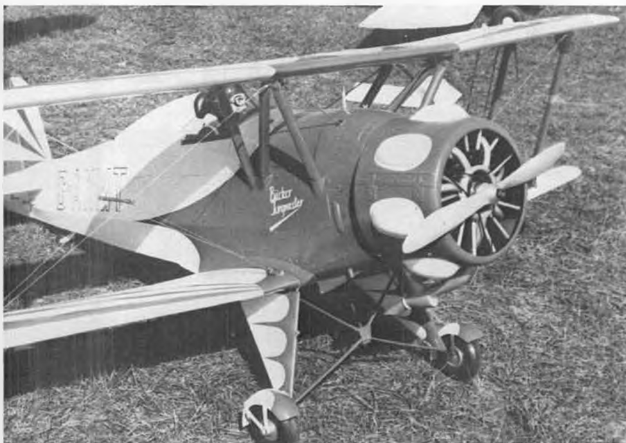
One of the precision quality models at the Kitchner was Mario Sabi's red and white Bucker Jungmeister . At 13 pounds, the model is powered by a Webra .91, and was built from Svenson plans. Just recently finished, and not yet flown, it looks like Mario hasn't yet made scale prop.
