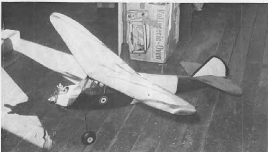
8. Clyde Austin's Commodore in final stages of restoration by Gordon Coddling, Kingman, Arizona. Thirty year old structure and covering is very dry and brittle.
