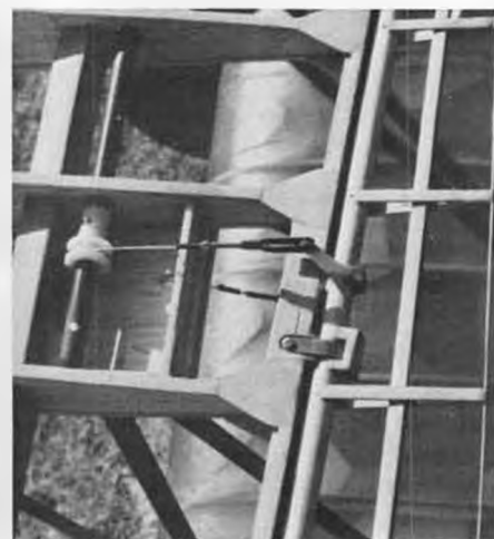
Cable controls drive the ailerons of Graham Ireland's Fokker D-VII. A combination of torque tube and cables does the job.
