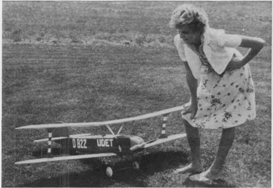
Tracy Keneagy admires Heinz Koerner's Udet Flamingo. A Keller 50/24 SL with Jomar Speed Controller and 20, 1.2 amp-hour cells powers this scale biplane. The prop used is an 11-7. The model weighs 7-1/2 pounds, has a 67-inch span, has a 1200 sq. in. wing. John Hickey pic.
