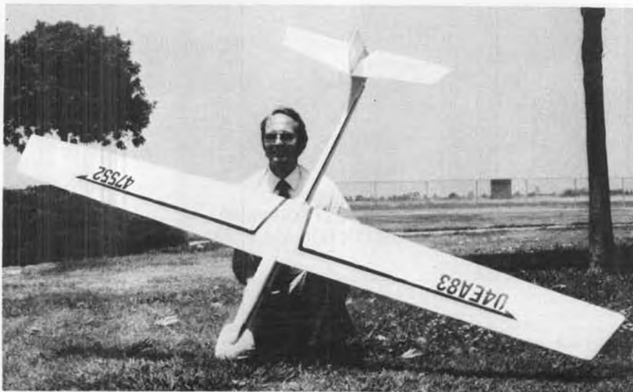
LEFT: Daryl Butcher, of La Habra, California, designed and built this multi-task model totally from scratch (including airfoils). Wing's built-up structure features transitioning airfoil sections from root to tip. ABOVE: Airborne shot of the U4EA83.
