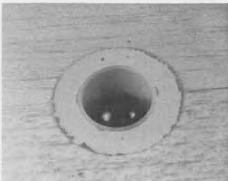
The finished fitting. Epoxy/microballoon mix is used to fill in around nylon guide, sanded off.
