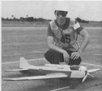
Terje Eltvik, of Norway, placed 45th. Note single retract wheel and wing skids.
