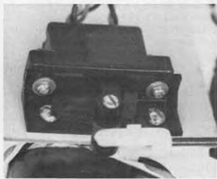
RIGHT: Internal switches are always best. Here's a close-up view of the D&D Bulkhead Switch Mount as used in the Cessna Ace R/C has this part.
