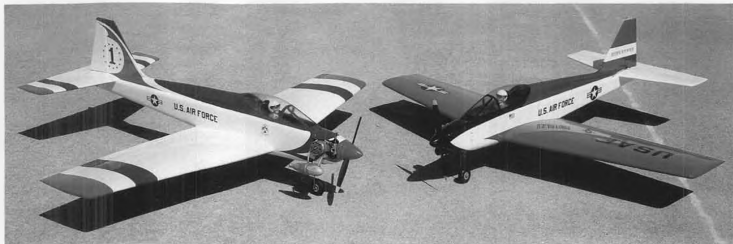
One of the notable qualities of the Kougat has been its fine low speed handling. The same built-in wing washout that contributes to this characteristic has been incorporated into the King Kobra. As this picture shows, it can also be slowed down for easy, nose-high touchdowns on the main gear.
