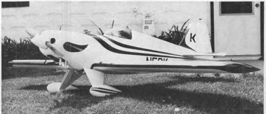
Clark Foy, of Ontario, Canada, cranked out this flawless, 27-pound Super-Fli from the Ohio Superstar kit. He used two-ounce fiberglass cloth and resin and acrylic enamel to get the finish he wanted. E. T. pilots the Quadra 50 powered model.
