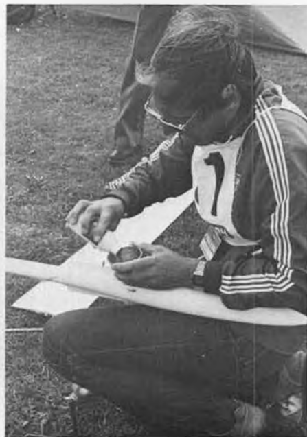
Kåre Schanche loads ballast shot into the side of the KITT-193 . Trap door provides access.
