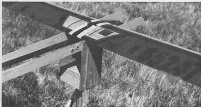
This close-up view of the stooge shows how wires are used to hold the model on the rails prior to launch.
