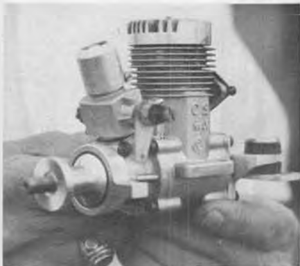
Vibration mounting and intake silencer on Tom Prossers O.S., cut down on dBs.
