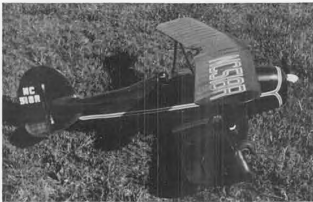
came out weighing 14-1/2 pounds with Quadra engine aboard. The model was covered with silk and finished with nitrate dope.
