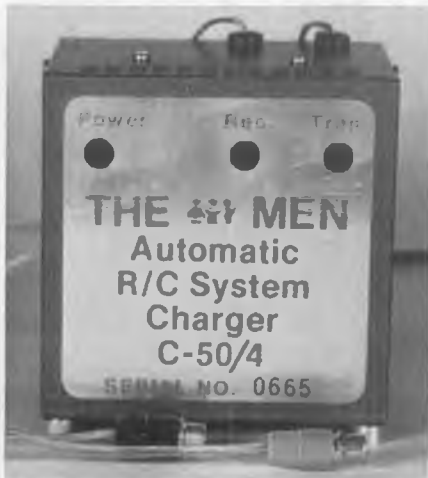
Although it isn't new, the M.E.N. C-50/4 pulse type charger for RX & TX works well.
