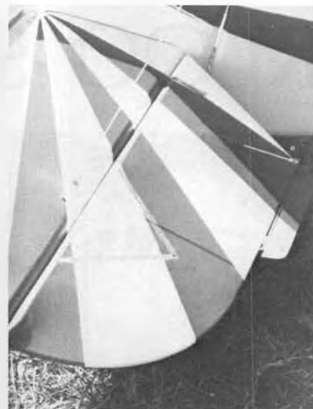
The elevator and fuselage (not shown) of the Jungmeister feature zippered inspection flaps with real zippers. Note trim tabs.
