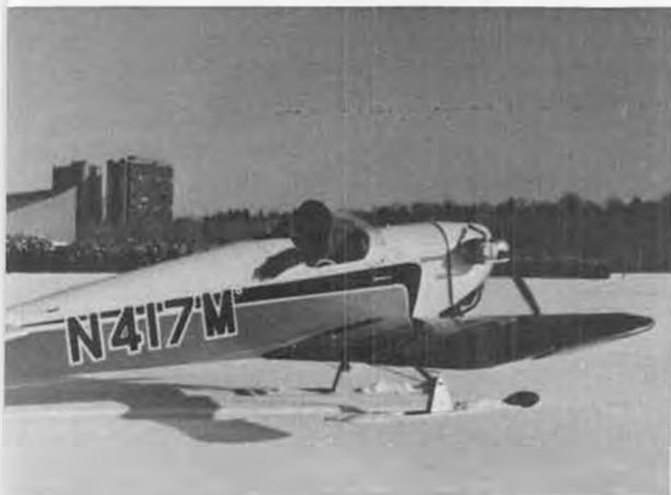
RIGHT: Ikon N'wst Porterfield Flyabout . It handles well, both on the ground and in the air, and has that "different" look. Now all I have to do is get Neely to put pilots in his cockpits. Enya .90 four-stroke powers the model.
