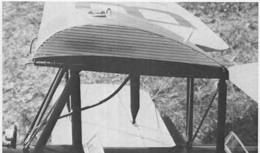
ABOVE: The wing tank of the Moth is constructed of aluminum printing plate which has been corrugated in a simple jig. World championship quality is obvious.
