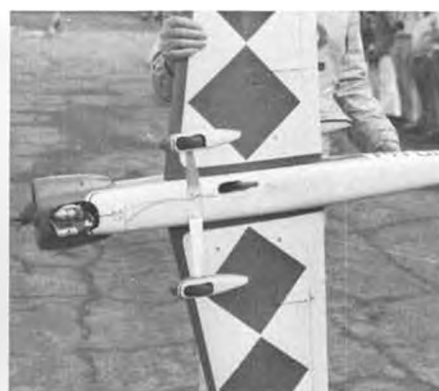
Underside of Van Beek model, showing Cessna-type gear, exhaust in plug-in wing screws.
