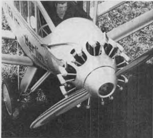
The dummy engine on Steve Gray's Bellanca WB2 conceals a Quadra. Note custom spinner and 6-bolt hub. Pilot looks real in the air!
