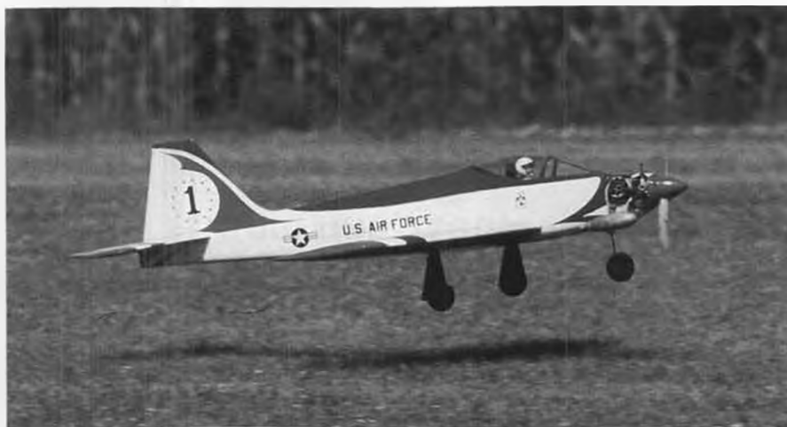
One of the notable qualities of the Kougat has been its fine low speed handling. The same built-in wing washout that contributes to this characteristic has been incorporated into the King Kobra. As this picture shows, it can also be slowed down for easy, nose-high touchdowns on the main gear.
