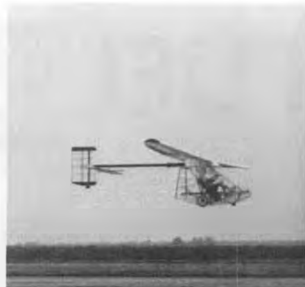
Paul Mac Ready's Bionic Bat man-carrying, electric assist airplane has won the latest Kramer prize. Initial test flights were done at night by a full moon. Silent and invisible!
