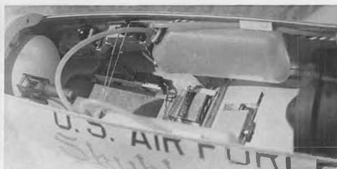
Inside of Jet Hangar F-86F, showing 24-ounce fuel capacity.
