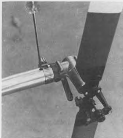
11. Allen wrench inserted into coupler's set-screw, through filed-out top groove holds tail rotor shaft in place as rotor hub is turned.
