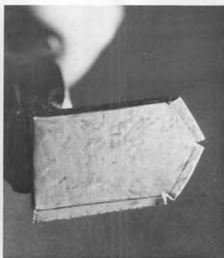
Tabs on end clamps being formed with flat-billed pliers.
