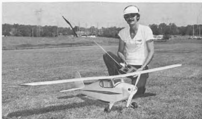
Les Adams, Arlington Heights, IL, with his 72-inch span Porterfield, Astro powered with 2.7 to 1 belt drive. Uses his own speed control.
