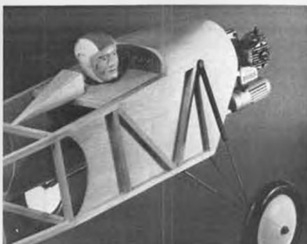
Instrument panel, Williams Bros. pilot (getting a little nosy here!) and headrest are trial fitted. Wood screw still to go through top of gear.
