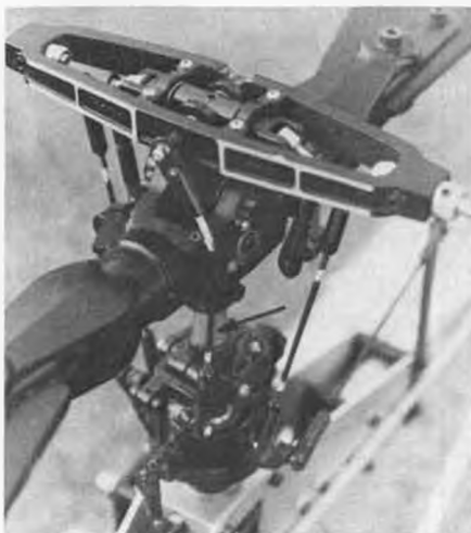
4. Hirobo rotor head used on Cobra is state-of-the-art. Author runs Hiller pushrod around yoke, not through center of yoke. See arrow.
