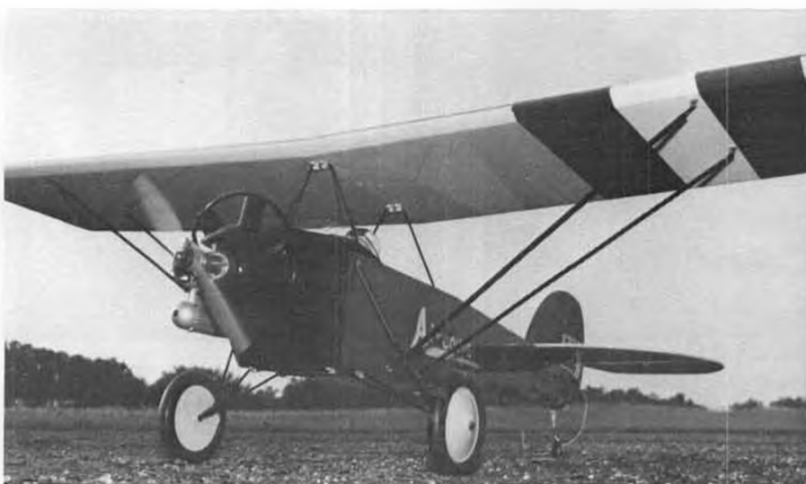
Low angle shot shows simple but functional strut attachment. They could be bolted on permanently, as the plane is relatively small and easy to transport.
