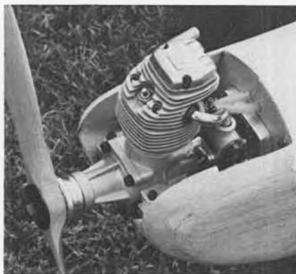
OS 90 four-stroke sticks out a little too much, but nose was not modified for kit review.
