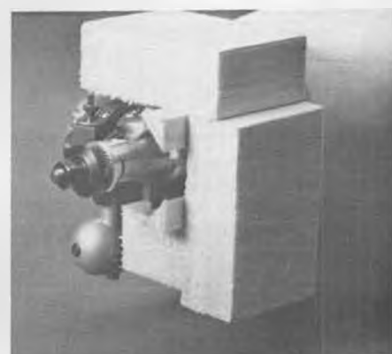
"Don't fence me in!" Engine gets surrounded with soft blocks, to form cowl. Lotts'a carving!
