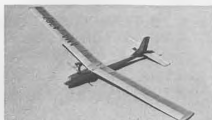
No. 1751 R/C TYRO TRAINER $3.50 Powered glider with removable .049 pow- er pod/hatch. Span 74". By Hank Cohan.
