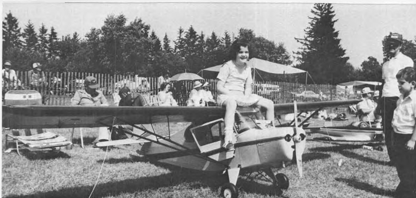
Karen Pelgrims demonstrates at the Kitchener Scale Rally that her 62 lbs. is no match for Peter Baabs' 45% size Aeronca 7AC Champ. A Jim Crawford design, the large model weighs only 53 lbs., flies on a 10 HP Chrysler out-board engine.
