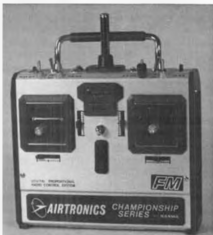
The Airtronics Championship Series CS7P transmitter, available with various plug-in mixer modules. See text for more info.
