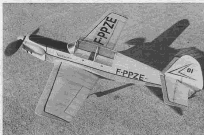
Larry Kruse placed fourth at the '84 Nats with this 3/4-ounce, 22-1/2 inch span rubber-powered Daltel DM-165.
