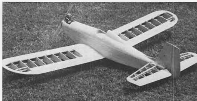
For pride in workmanship there's nothing so inspiring as a nicely sanded out balsa airframe. Very few changes from original "Hog."
