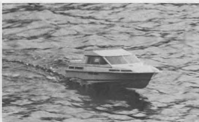
It sure goes nice in fast forward! Speed is estimated at 10 to 12 mph, which is moving right along as compared to most electric boats.
