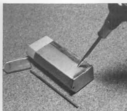
Scratch awl is used to puncture holes for brass tubing.
