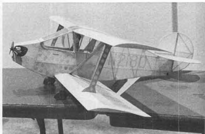
Electric powered Sorrell "Guppy" by Addie Naccarato. Similarity to Hiperbiplane and Hiperlight is obvious. Note all the lightening holes.
