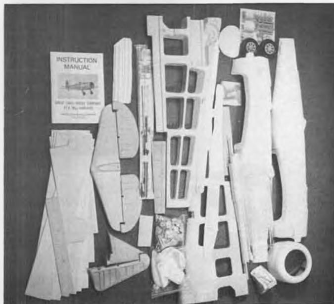
Spill-out of kit parts for the Great Lakes Model Co. AT-6/SNJ/Harvard. All molded material is urethane foam. At least 1001 fittings!
