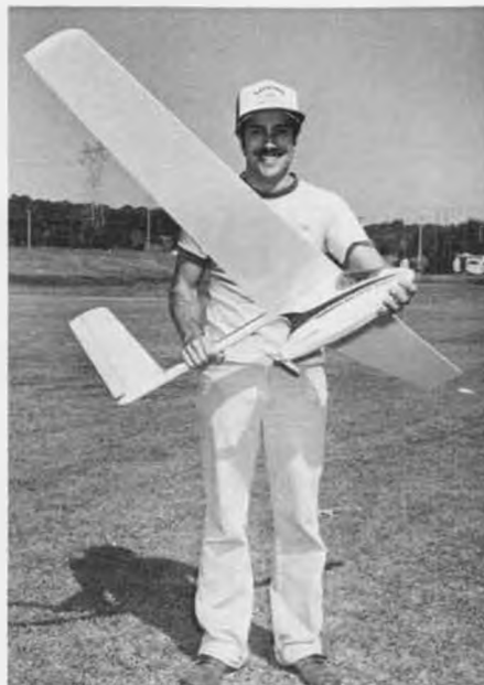
Ken Stinson, Telford, PA, with semi-scale American Eaglet. Span 80 inches, 40 ounces, Pittman cobalt, six cells. Launch with care!
