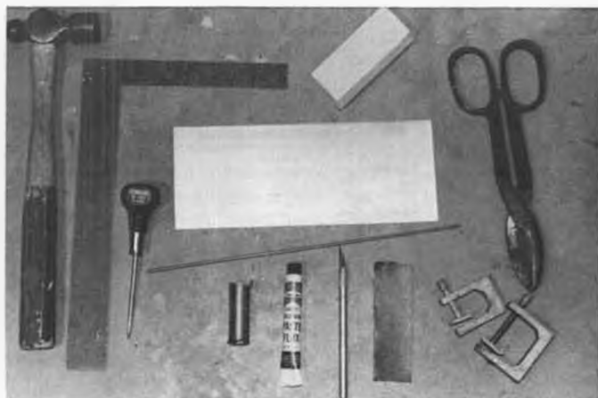
Most of the items needed to "build" a brass fuel tank. Stock tanks don't always fit the original design you created.
