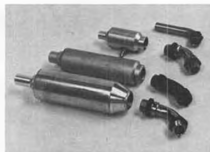
OS and Enya exhaust systems. They're pretty much interchangeable.
