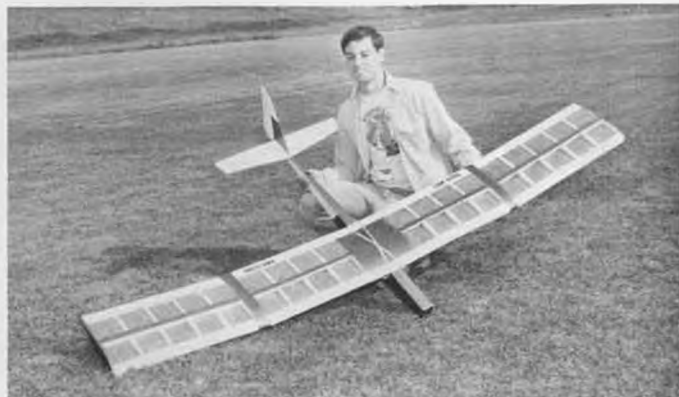
Brian Bailie, Robbinsville, NJ, with his very unusual computer designed sailplane. Its 36 solar cells produce 36 watts.
