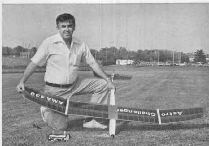
Bob 'Astro Flight' Boucher with his new Astro Challenger. Span 72 inches, 39 ounces, geared Astro 05 cobalt with seven cells.
