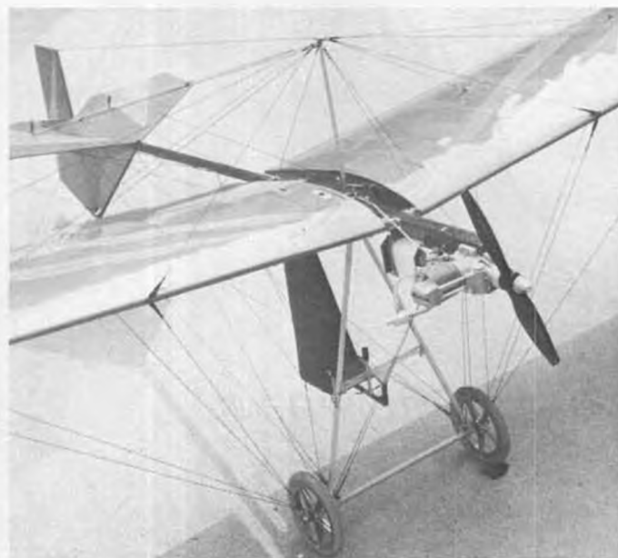
Leo Hopper, Pomona, Calif., built this 1/4-scale 'Woodhopper' ultra-light. Span 103', O.S. 61 four-cycle, weighs 7-1/2 pounds
