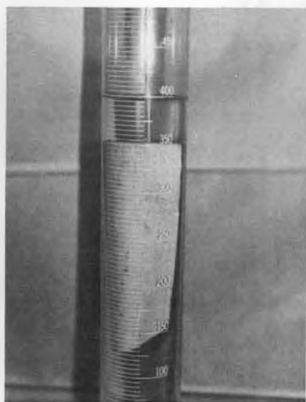
Odd shaped tank pattern submerged in graduated container to check capacity displacement.
