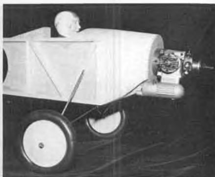
Carve recessed area to fit your engine's muffler. Later change to an Enya .19 required cutting off 'stinger' of .19's muffler. No problem.
