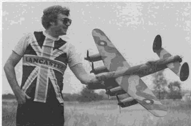
Dennis Norman with his awesome rubber-powered Avro Lancaster. All props are powered, and model has exceeded 30 secs. Scott photo.
