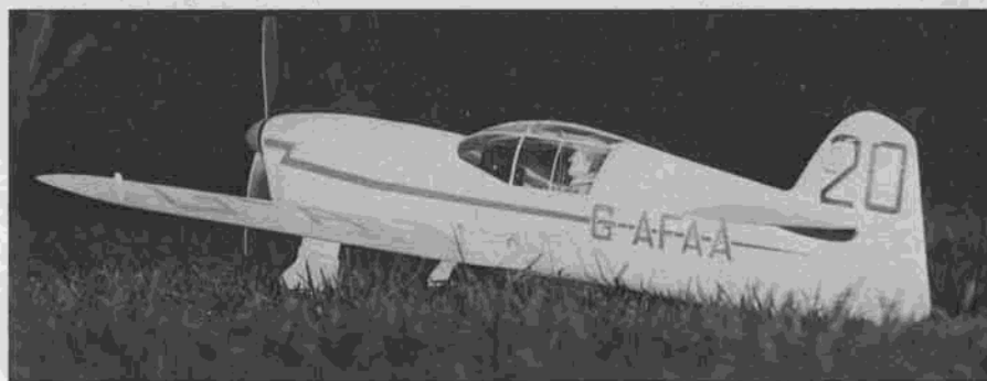
Percival Mew Gull, CO 2 powered free flight by David Deadman, of England. Has twin fuel tanks, slightly enlarged tail surfaces, weighs approximately 2-3/4 ounces.
