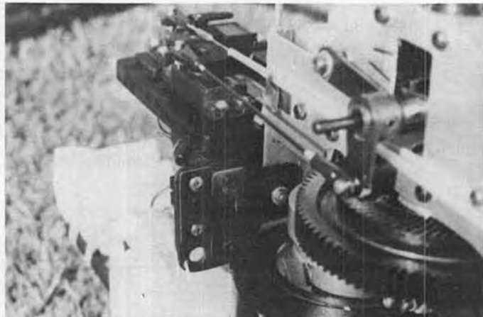
9. Add-on switch mount is shown screwed to front frame. Use pattern on next page if you wish to make one for your installation.
