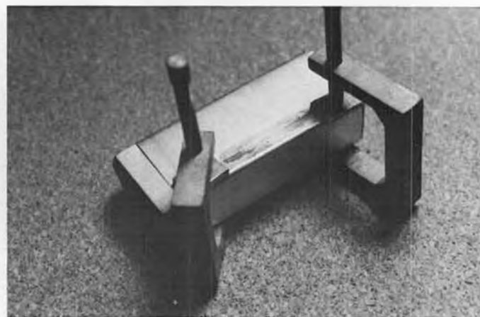
Clamps hold seam tight while middle portion is soldered. Then remove clamps and solder the remainder.
