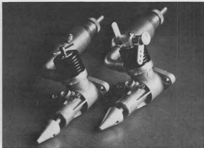
Tuned pipe versions, new and faster. "John" Racer on left turns 18 K at max power. R/C version has variable compression control.
