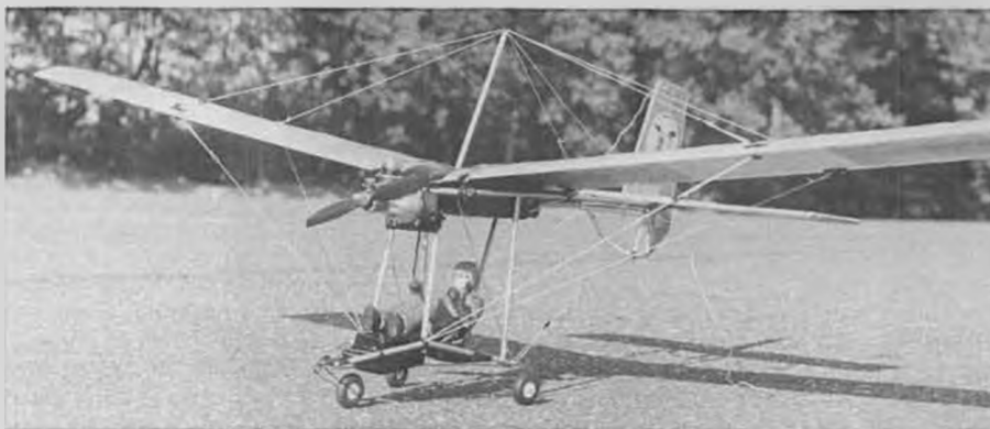
The Sky Rally takes about three hours to assemble. Scale is 1/8, giving a span of 43 inches. Power is the well-known Cox QRC .049 engine. Requires two-channel radio.
