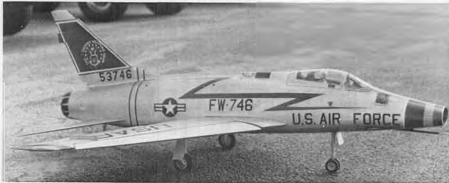
This F-100D was designed and built by Art Johnson, Delray Beach, Florida. Powered by a Rossi .81 and Byrojet fan unit.
