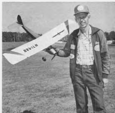
Dwight Holley, Bethel, CT, former FAI soaring world champ, with his cobalt 05 powered original design. Span is 40 inches.
