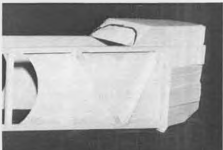
Soft 1 x 1-inch blocks cut to fit between firewall and bulkhead "D". No plastic here!
