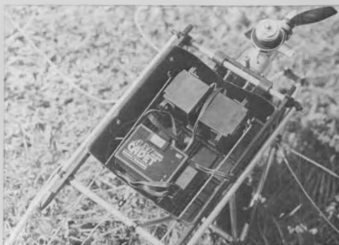
Radio gear fits in tray covered by wing. Cox/Sanwa drops right into place, using double-stick foam tape provided in kit.
