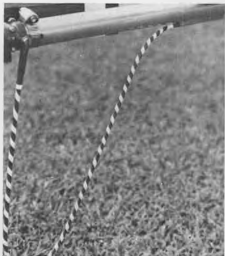
5. Modified 'stinger' is 1/8" brass tube, screwed to gearbox collar at rear, runs through tube epoxied to tail tube. Hot-Stuffed in place.
