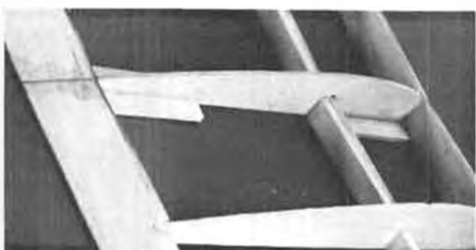
Center rib is ply, used as blank to cut others. Ply plates added to support wing mounting blind nuts. Wing not removed since finished!
