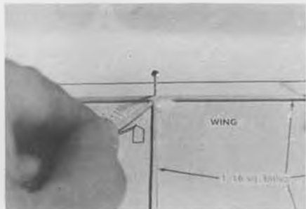
Wipe excess glue out of joints with balsa stick. Leave small fillet of glue for strength.
