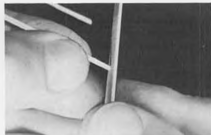
Using sanding block or sanding stick, make an angle on end of L.E. and T.E. before gluing in the dihedral. Careful, sticks are fragile.
