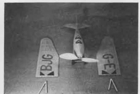
Parnall Pixie with plug-in wings unplugged.
