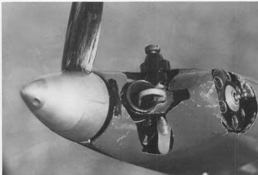
Gary Gau's QM use one-blade Bolly prop and O.S. inflight mixture control with flood-off. Bolly details coming in future Ramblin' column.
