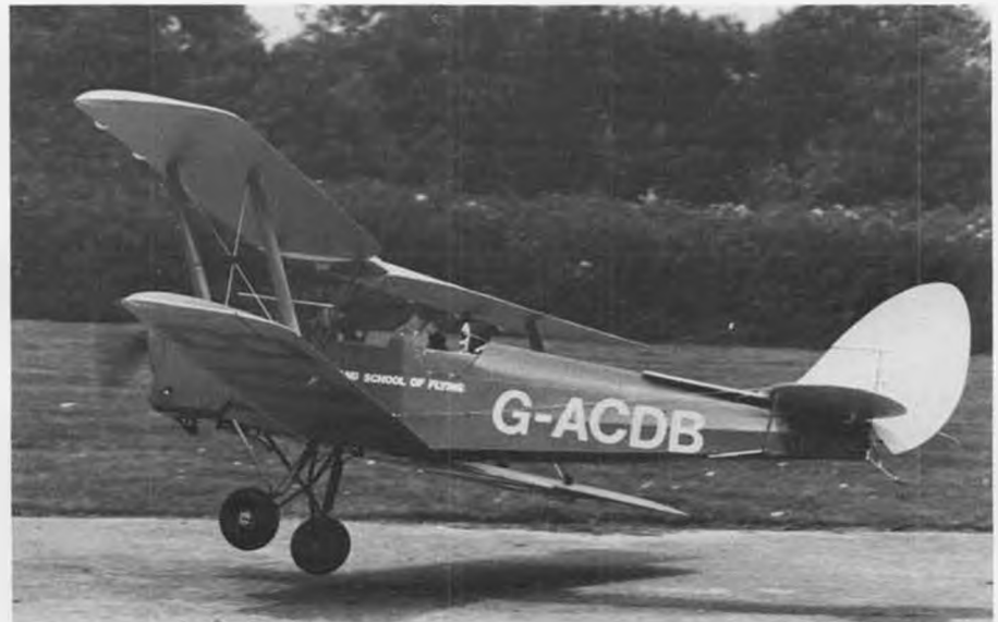
A large biplane, a narrow-stance landing gear and a sudden gust of wind on takeoff, all the ingredients for disaster. The reduction unit in this Tiger Moth, homemade, enables the plane to accelerate to a safe maneuvering speed when necessary, like in this instance!
