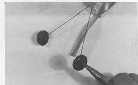
Bend ends of landing gear wire up with pliers to keep wheels from falling off. Wheels should be free to turn.
