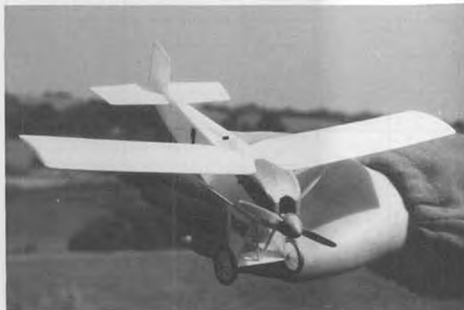
All-foam Benes/Hajn racer by Antonin Alfery is powered by a Gasparin motor of only 2 cubic millimeter displacement!
