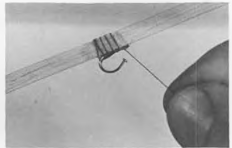
Attach special rear motor hook with glue and thread. Rub glue into thread.
