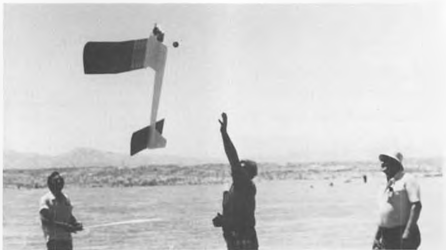
Sal Taibi launches our K&B .40-powered 900 Starduster on its first flight, at the 1976 NFFS Champs, Taft, California. That's WCN on the transmitter. Completely hidden R/C system controls rudder tab and trimmable stab platform. Tatone cutoff timer is only engine control. Details on R/C installation in next issue. See Ron St. Jean's letter in this month's text. At end of flight, we steered 'Duster back to starting spot, and Sal caught it. His comment, "How am I going to keep my trim figure if I don't have to chase it!"
