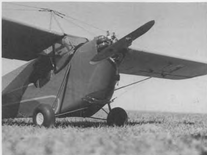
Ian Watts' Giant Scale Aeronca C-3 Collegiate used a Saito .90 twin.
