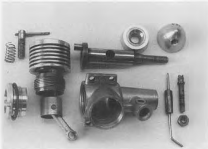
Low piece count of screw-together engine is apparent. It was mass-produced in small volume in New Zealand.
