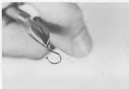
Bend pin for rear motor hook to replace the straight one shown on plan.
