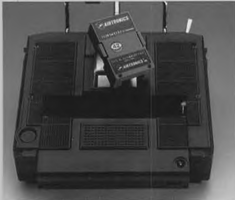
Easily accessible removable NiCd battery and RF module.
