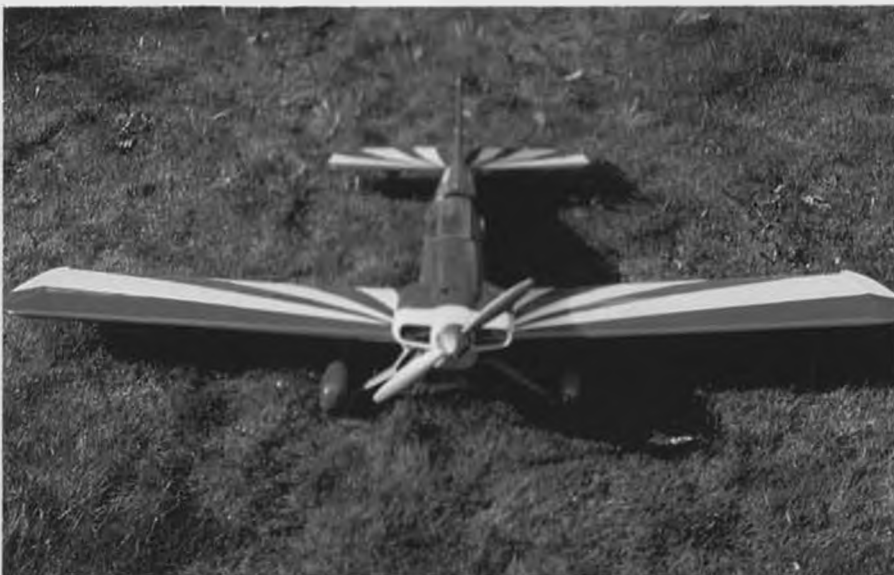
Nose detail on the Bobcat. A cowl available from Ikon N'West will fill the bill. Author advises reinforcing the entire cowl unit with 2-ounce fiberglass cloth and resin or cyano glue.
