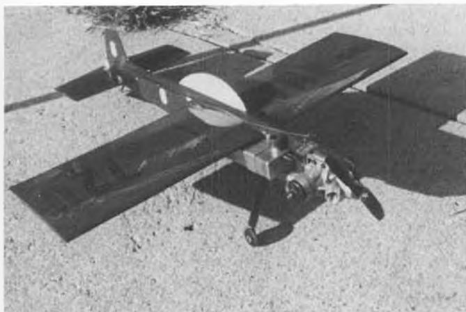
Scoville Starduster Goodyear racer built by George Lieb. Note the simple fuel shutoff installation behind Rossi engine.
