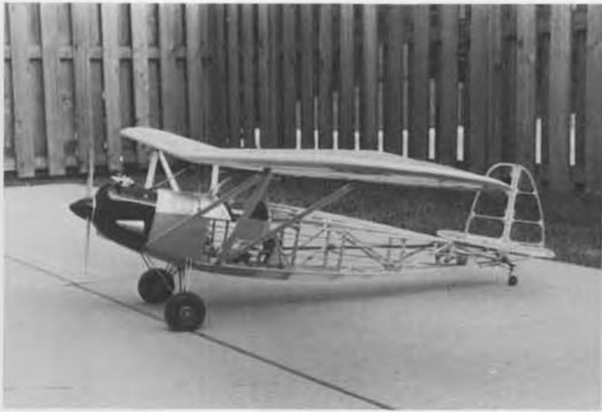
After home-brewing his Aero 94 four-stroker, Jack Moore needed a bird to put it in, so he built this Q-scale Heath Parasol LNB-4.
