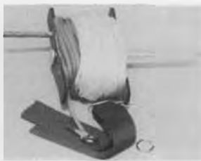
The ZIP-START — a hi-start designed for launching 1½ or 2 meter sailplanes. Includes 30' of ¼" ID ultraviolet stabilized natural latex rubber tubing, 250' of heavy duty 160# nylon line, 3 tempered steel tow rings, 8" steel stake, tow marker ribbon, reel assembly and instructions.
