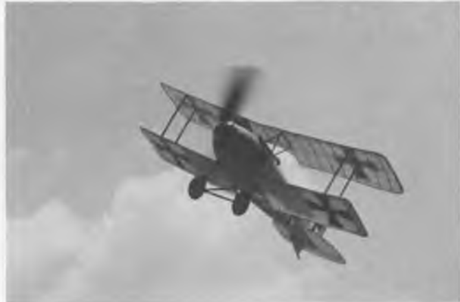
Pistachio Scale Albatros D11 by Tonda Alfery, of Czechoslovakia. It features foam styrene fuselage.
