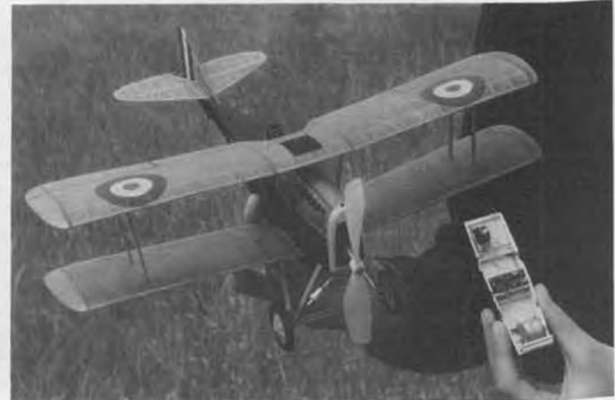
A 1/20-scale Ansaldo Ballila constructed by Antonin Alfery with CO 2 engine and R/C equipment made by Stefan Gasparin.
