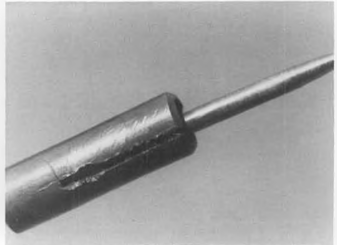
Collet on the needle valve was split with a simple saw cut.
