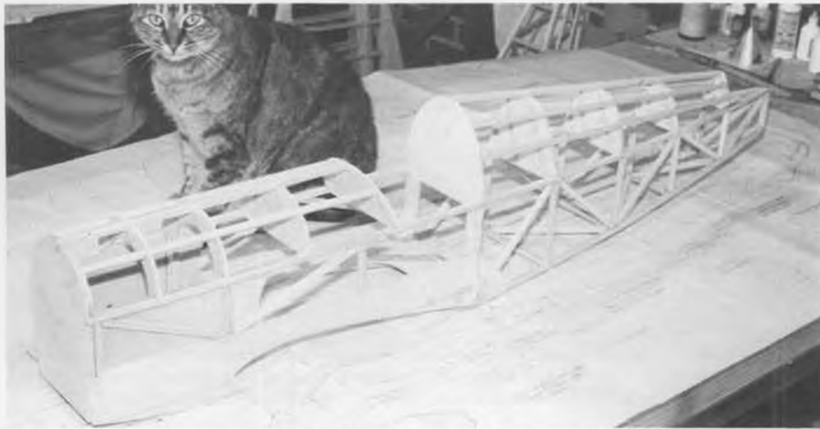
Jenny, a pretend bobcat, with the basic fuselage assembly of the model Bobcat.
