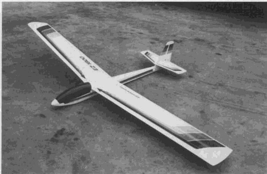
The new EZ-1800 from EZ Sports Aviation has E195 section and fully sheeted wings for efficiency. Almost ready to fly.
