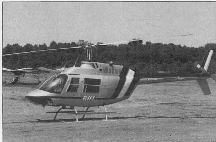
The full-size Bell 206B Jet Ranger employs a totally free teetering main rotor, which makes for a smooth ride but greatly reduced maneuverability. Text explains this in greater detail.
