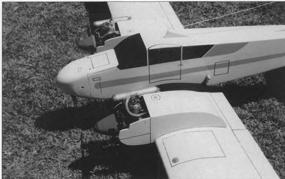
The O.S. 25 FPs are snug in their nacelles, which are not built into the wing, but are attached to the top surface only. Simple but effective.
