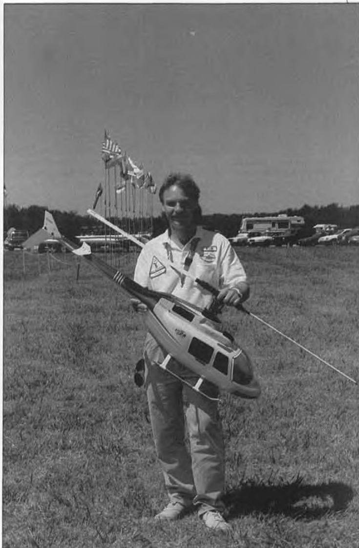
Robert Gorham's 1989 World Champs entry was this colorful Jet Ranger with GMP Legend mechanics, Elite rotor head, 58-inch rotors, Enya 60 XLF IV engine, and Hatori tuned pipe. If you decide to use Legend mechanics and want to retain the belt-driven tail rotor (Robert used a TSK wire-drive unit), the stock Legend tail boom will have to be mounted inside the fiberglass shell.
