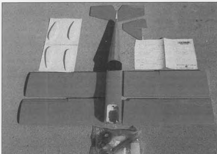
This is the way it comes out of the box, and that's real Top Flight...er...Great Planes Super MonoKote covering film. Construction is primarily balsa and ply.
