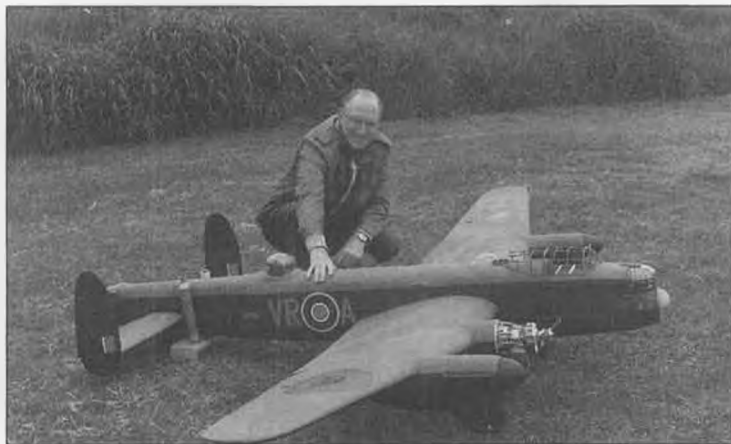
Len Bosman and his 137-inch span, 36-pound Avro Lancaster Mk I powered by two Quadra 40s. Outboard props are freewheelers.
