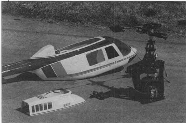
Here we see the fuselage has been painted, the canopy has been tinted, and the Competitor mechanics are ready for installation through the fuselage top. Fuselage was finished with Pactra Formula U; Testors transparent blue paint on the canopy.
