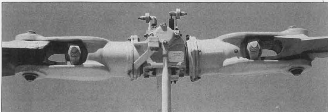
This shows the totally free teetering main rotor design on the full-size Jet Ranger. Main shaft is hollow. Doesn't it look like the GMP flybarless rotor head?
