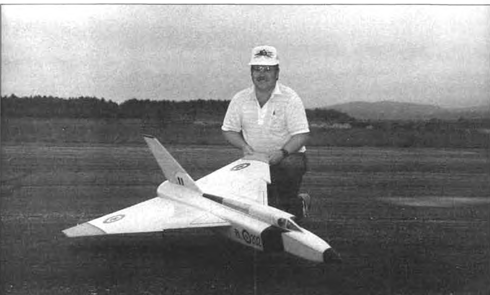
Chuck Thorton's very nice flying Parkinson AVRO Arrow 105 was evidently one of Bob Parkinson's first production kits, as it had the old fiberglass fuselage. Power is an O.S. 91/Byron fan combo.
