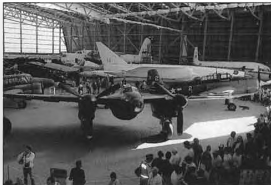
DeHavilland "Mosquito" bomber, Hangar 1 at Duxford. Made of spruce and balsa, they were fast, lightly-armed, and constructed in converted furniture factories. They could carry almost as many bombs as a B-17. Yes, that's a Grumman TBF "Avenger" with Lt.(jg) George Bush's name on it.
