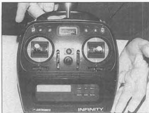
Airtronics' revolutionary new Infinity 600A transmitter is a total visual departure from existing designs. Inside resides a computer programmable sailplane radio. See text.
