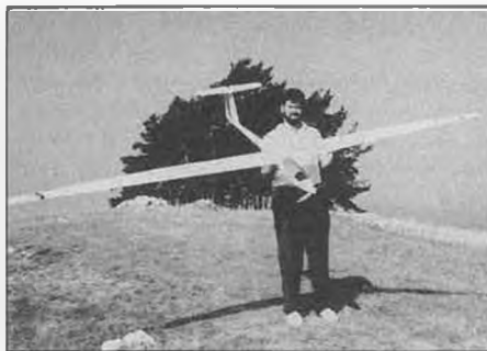
The "Vario" electric powered sail plane spans 140 inches—152 inches with the wing tip extensions in place. Another new Hobby Lobby offering.
