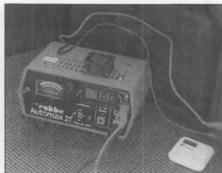
Another example of a charger cooling fan, mounted atop a Robbe unit. If your charger gets too hot for your liking, one of these 12-volt fans (a Radio Shack item) will solve the problem nicely.
