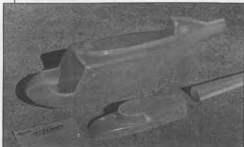
(Left) The three major pieces of the GMP Jet Ranger fuselage kit are the molded fiberglass body section, top hatch, and tail boom. It's available as a fuselage kit only, or with your choice of GMP Cobra or Cobra-Mustang mechanics. (Center) Die-cut plywood fuselage formers are nicely done and literally fall right out of their sheets. (Right) The basic Jet Ranger fuselage assembled, with the plywood formers, hardwood mounting rails, and balsa stabilizer glued in place.
