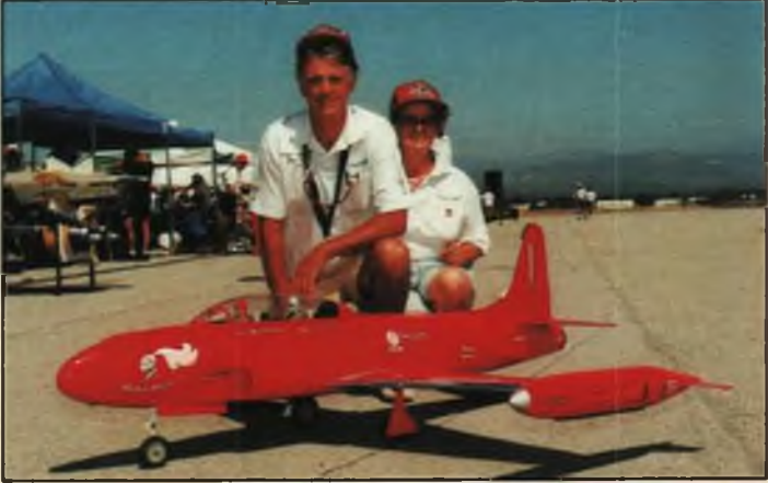
■ BELOW: LEFT Mel Santmyer's entry was this immaculately built and detailed Super Corsair racer, modified from a Byron Idt. The airplane spans 6 feet, weighs 28 pounds and is powered by a 60cc Sthl engine. ■ BELOW RIGHT: Jeff Foley's colorful "Red Knight" Lockheed T-33 earned him an excellent 4th place overall. The model spans 85 inches, weighs in at 24 pounds, uses an D.S. .91 and JR PCM 10 radio.
