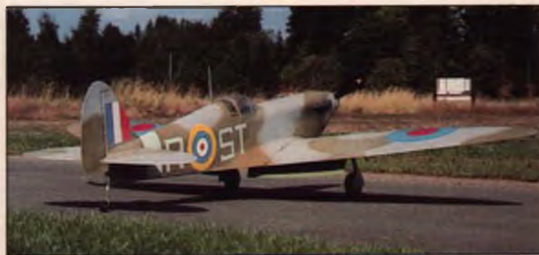
■ ABOVE: Bob's Spitfire now sports large wing root fairings and split flaps; the latter help greatly in getting this lightweight floater back on the runway. ■ BELOW: Underside view of the flap installation. Because the wing was already built, it was easier to install an individual servo for each flap; starting from scratch, it should be easy enough to work out a reliable single-servo installation.
