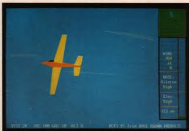
The high-performance electric glider on a low pass. The readout along the bottom shows the plane is 20 feet away (DIST), is flying at a true airspeed of 100 mph (TAS) at an altitude of 8 feet (ALT).
