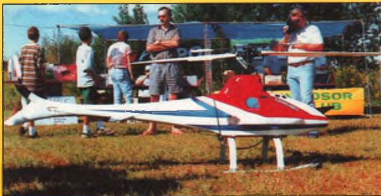
The huge cropdusting helicopter manufactured in Japan by Hirobo/Yamaha. Rotor diameter is 8 feet, and the flying weight is 100 pounds—too heavy to be permitted to fly at the Schluter Cup. It sells for around $35,000.
