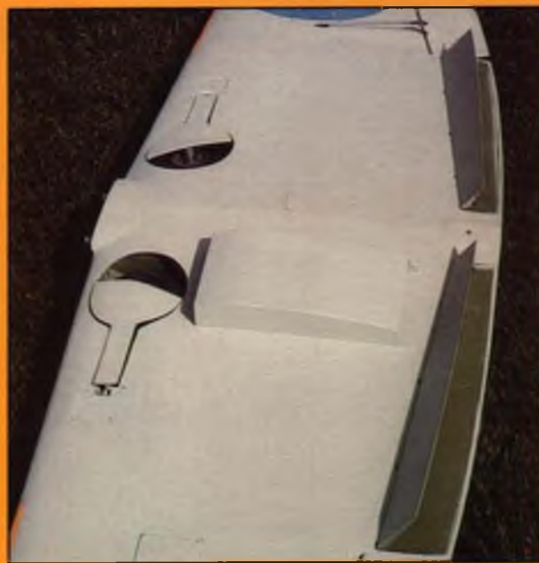
■ ABOVE: Bob's Spitfire now sports large wing root fairings and split flaps; the latter help greatly in getting this lightweight floater back on the runway. ■ BELOW: Underside view of the flap installation. Because the wing was already built, it was easier to install an individual servo for each flap; starting from scratch, it should be easy enough to work out a reliable single-servo installation.
