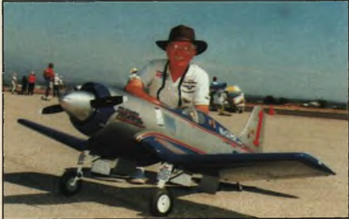
■ BELOW: LEFT Mel Santmyer's entry was this immaculately built and detailed Super Corsair racer, modified from a Byron Idt. The airplane spans 6 feet, weighs 28 pounds and is powered by a 60cc Sthl engine. ■ BELOW RIGHT: Jeff Foley's colorful "Red Knight" Lockheed T-33 earned him an excellent 4th place overall. The model spans 85 inches, weighs in at 24 pounds, uses an D.S. .91 and JR PCM 10 radio.
