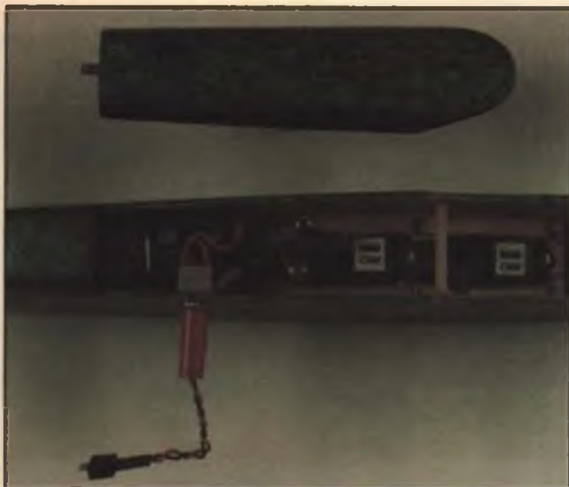
Despite the thin fuselage, there's still plenty of room for a Cirrus receiver (case), a 270-mAh battery in the nose and two DAD Tins micro servos. Aileron cable pushrods are connected to the aileron/rudder servo and the wing is bolted in place. Also pictured is the phone jack that serves both as the radio switch and charging plug—lighter and more compact than the typical slide switch.
