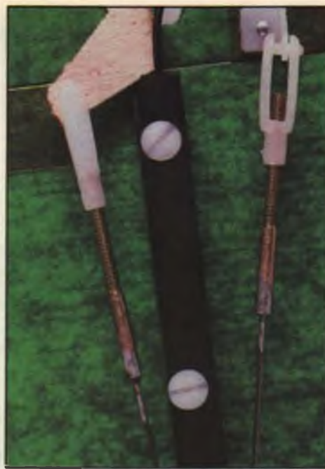
Extreme close-up of the bottom of the tail shows the pushrod hook-up and the two 4-40 nylon screws that hold the tail assembly to the carbon fiber boom. Dennis is also running his receiver antenna through the boom—usually a no-no, but he lets several inches of it hang out the end and reports no problems with radio range even at steep altitudes.
