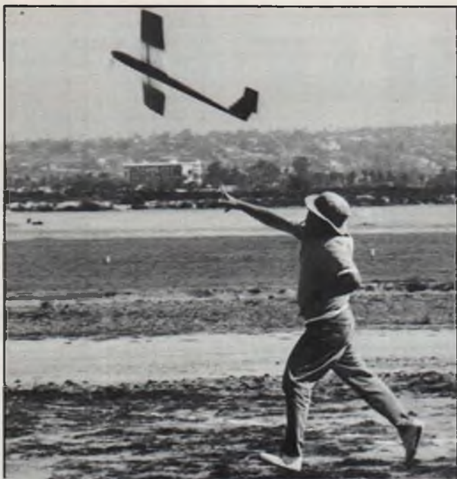
Bob Sill's ship gets a hearty heave from eventual meet winner Steve No. 1. These airplanes are incredibly fast, have very light airframes and are sized so that the surface loading comes out right at the FAI maximum of 24.87 ounces per square foot.
