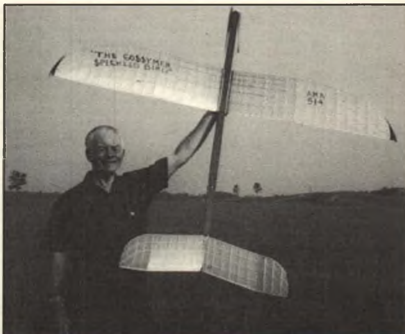
George Perryman shows off his "Cossymer Speckled Bird"—a huge and incredibly light unlimited rubber powered model. Wing and stab have lots of speckles which don't show up in the photo. More details in text.
