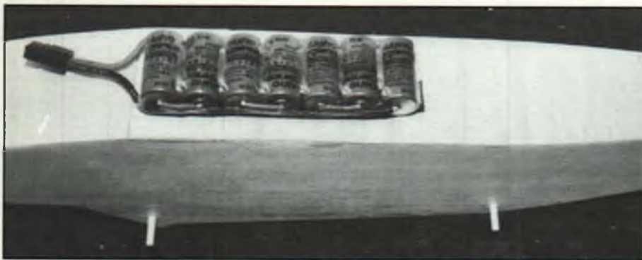
After the top and bottom of the fuselage are sheathed, a 2x5-inch opening is cut into the bottom for installation and removal of the motor battery. The pack is held to the bottom of the intermediate sheet balsa floor inside with Velcro.
