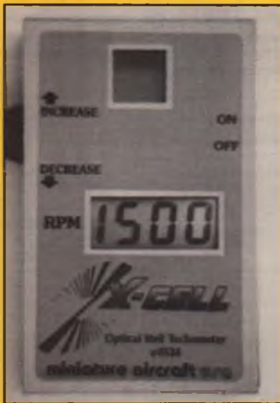
Miniature Aircraft's optical tachometer—handy for measuring a helicopter's rotor speed. Safe, accurate and easy to use.
