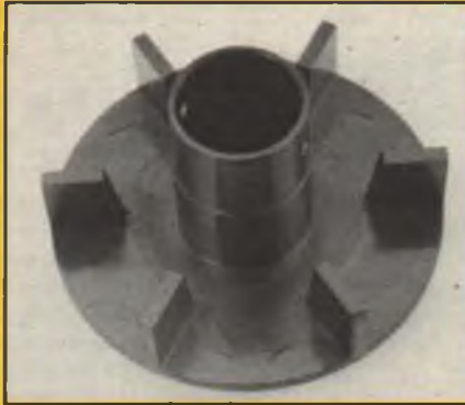
KSJ's machined aluminum throttle arm, available for the O.S. 32 and O.S. 61.
