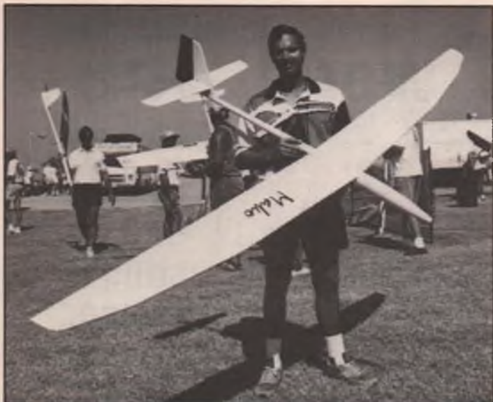
Ben Clerx now offers an upgraded Mark II Mako. The primary differences between this and the original Mako are: 1) the "Joe Wurts F3B wing planform," which has a little less tip area for higher aspect ratio and more elliptical lift distribution; 2) carbon wing skins replace the obuchi skins; and 3) carbon spar and joiner rod system. Mako II's will be available by early 1998.
