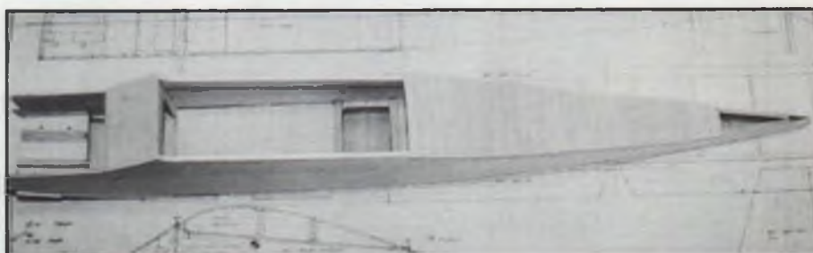
The Scout's fuselage is a simple box structure built mostly of 1/16 sheet balsa, with doublers in the wing saddle and nose areas only. An intermediate sheet balsa floor separates the cabin area into upper and lower compartments—the servos, receiver and speed control go on top, the motor batteries below.
