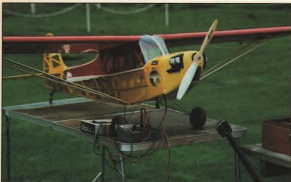
Here the Cub is coiled up and an Astro Flight Model 112 charger is in the process of charging the two series-connected 14-cell NiCd battery packs. Cutout in the cowling just below the prop is for cooling air for the motor and batteries—a necessity for any sport electric model. The Zinger 18x8x14 prop used for the initial flights has since been replaced by a Forte 22x12.
