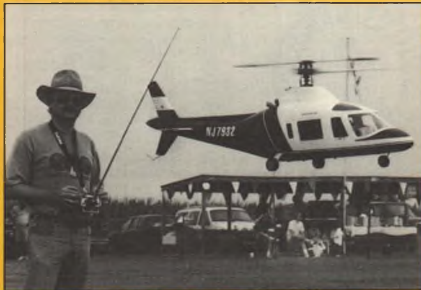
English heli enthusiast Jim Davey flying his .30-size Shuttle at the New Jersey fun-fly. Model has Hel-X sideframes and an Augusta A-100 fiberglass fuselage from Yellow Aircraft. A very smooth and scale-like flier.
