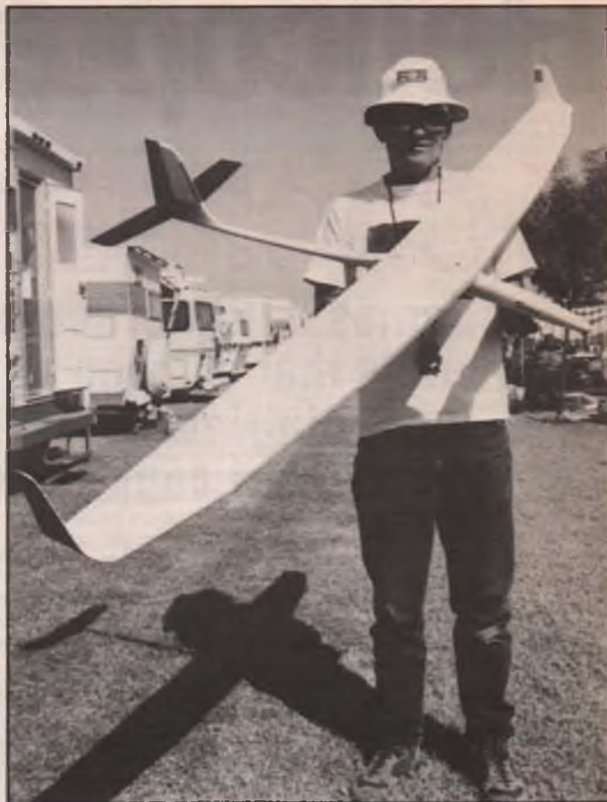
The most unusual original design was Jerry Robertson's 2-meter "Sisu" (Finnish for gutsy). The 35-ounce model featured a most unique aileron which spanned the outer two wing panels and tapered to a point on the T.E. nearest the wingtip in a kind of "rectangle/triangle" shape. This was done to eliminate any tip vortex (i.e. drag) formed by aileron deflection. Other performance-optimizing features included tiplets to increase L/D and a drooped nose to minimize fuselage drag. The 585 square inch, 34083 wings are custom cut from a combination of gray and Spyder foam, then vacuum-bagged inside carbon fiber skin by Fred Sage.
