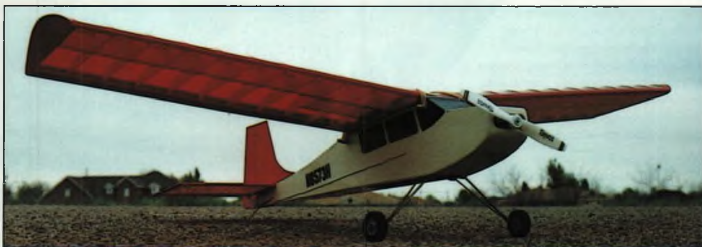
From any angle, the Electric Scout is a fine looking model. Author's prototype is covered with a combination of MonoKote and Ultracote. Keep it as light as you can for best performance.
