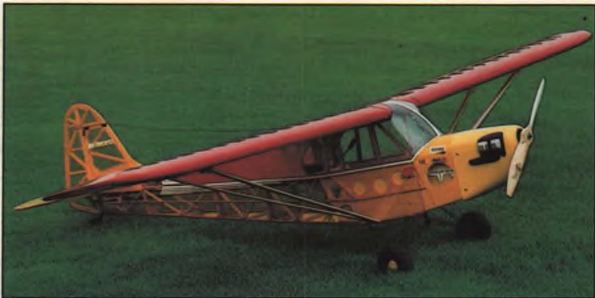
What better subject for an electric Big Bird than the venerable J-3 Cub? Bruce picked up this frame-up but unfinished Bob Hoover 1/4-scale Cub at a local hobby shop and with the help of a couple of buddies, successfully converted it to electric power. Cow! is from Fiberglass Specialties and has the dummy Continental engine cylinders milled in. Bruce says the most difficult part of the project was the windshield, as he had no patterns to work from.
