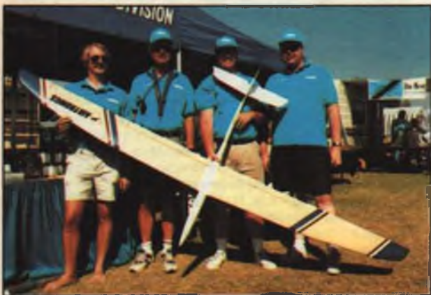
Team Airtronics (Specialty Division) is always improving their product line. Now for 1998 is the Sapphire, with a span of 118 inches, area of 868 square inches, and 87037 airfoil. What sets this one apart from the 1995 Peregrine is a new triple-bay planform, new fuselage with slip-on nose cone and all holes pre-drilled, 1/2-inch diameter CF joiner rod, built-up stab, and a molded fiberglass fin post. From left: Joe Wurts, Strip Miller, Tim Renaud, and Bob Renaud.
