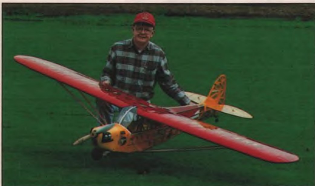
Bruce wanted something other than the standard all-yellow Cub livery, so he used Goldberg's new transparent Ultracote, orange and yellow, with white trim tape separating the colors. Unusual and attractive. Final flying weight is an even 18 pounds.
