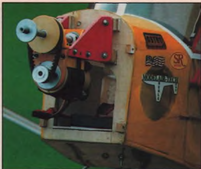
Astro Flight's Cobalt 60 electric motor fits nicely into Modclair-Tech's H-1000 belt drive unit, which is here is mounted to the firewall via homemade fiberglass brackets. The speed reduction ratio on this particular unit is 2.15:1; other ratios are available to fit a variety of model requirements. On the bottom of the housing are the battery charging plug and the all-important arming switch.
