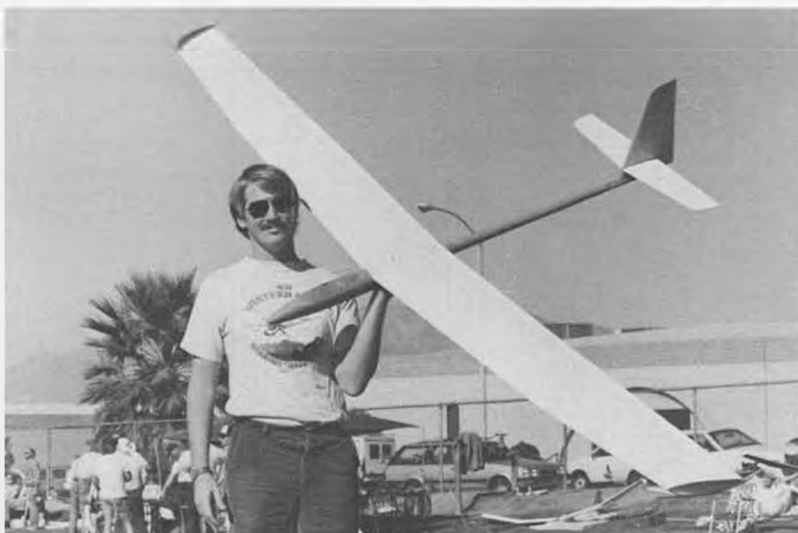
The man to beat, Joe Wurts, shows off his latest creation, called "Ariel", at a recent SC 2 meet at Riverside, California. Structure is almost 100% composites, very little wood used.
