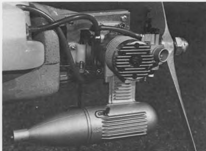
Side mounted O.S. 61 ABC is bolted to a metal plate. Tank is just a bit too high, so carb floods easily.
