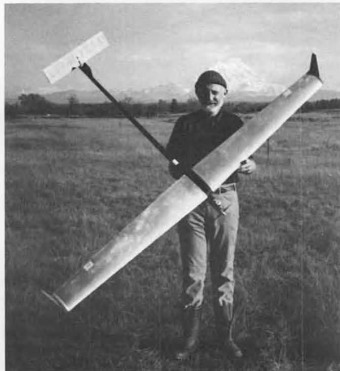
Ralph Cooney with his state-of-the-art F1C V-wing model. Note the tiplets and shallow dihedral. Text has more details on this design feature. Site is Harts Lake Prairie, in Washington. Stalick photo.
