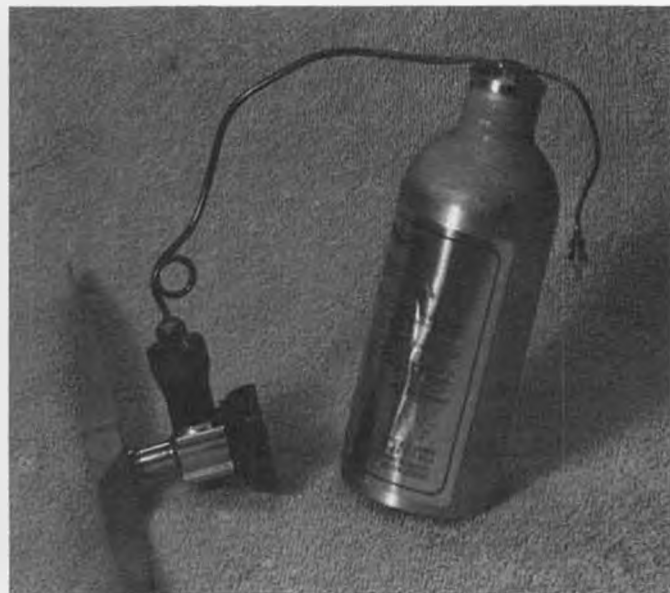
Nifty .049 CO 2 conversion with 150cc jumbo tank, from Davis Diesel Development. Can turn up to a 14x6 at useable rpm.
