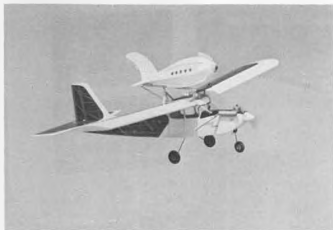
Skip Ruff's "Martian Spaceship" F/F glider being piggybacked to altitude by his Sig Kadet Seniorita. Photo at right shows the glider in free, stable flight. By doubling the fin area, stability has been much improved. Stay tuned...
