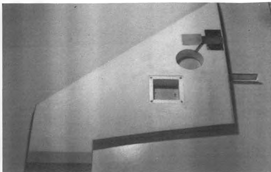
Bottom view of one of the Bullet's wing panels reveals cutouts for the landing gear and aileron servo. Molded foam parts were fiberglassed and finished with K&B epoxy paints.
