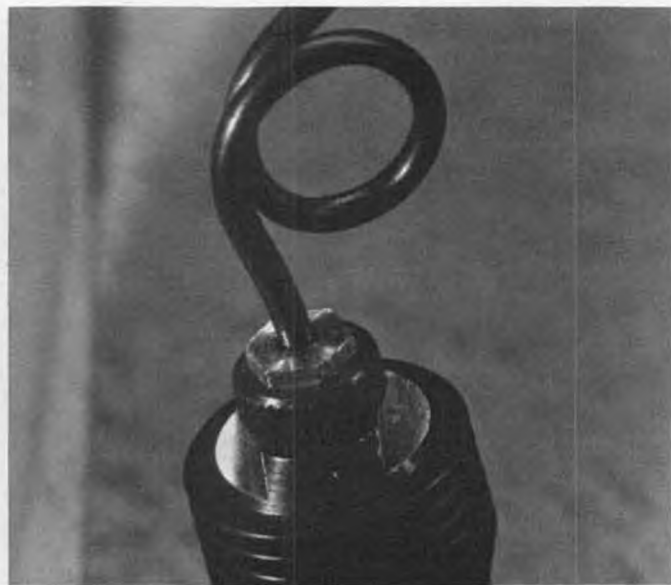
Close-up of the speed adjustment knob on the .049's CO 2 conversion head. See text for more info.
