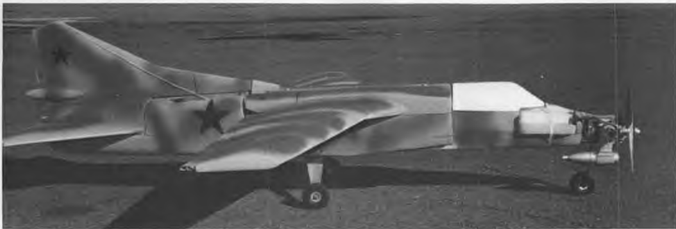
This month's subject sits on the flight line in full battle dress. It's the Mig-27 Flogger D, made by RS Systems originally as a target drone for the military, now being made available to the modeling public. This one has the optional tricycle landing gear installed.
