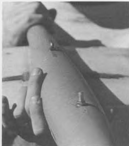
Ariel's landing "skid" is actually the end of a bolt, which digs into the grass and/or dirt and brings the model to a screeching halt. Simple and effective, but is it safe? Our columnist doesn't think so.
