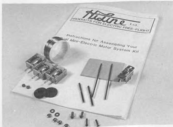
HiLine's do-it-yourself electric motor kit, complete with all the hardware required to make a geared power system.
