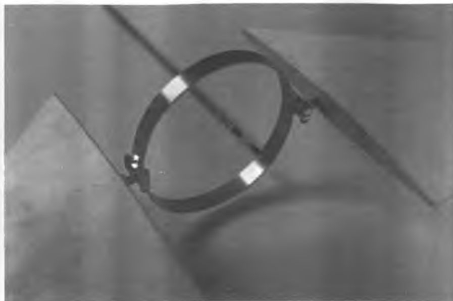
Stabilizers are controlled by a metal ring that fits around the exhaust tailpipe. Provides a very rigid mount for the tail surfaces and does not interfere with the jet exhaust.
