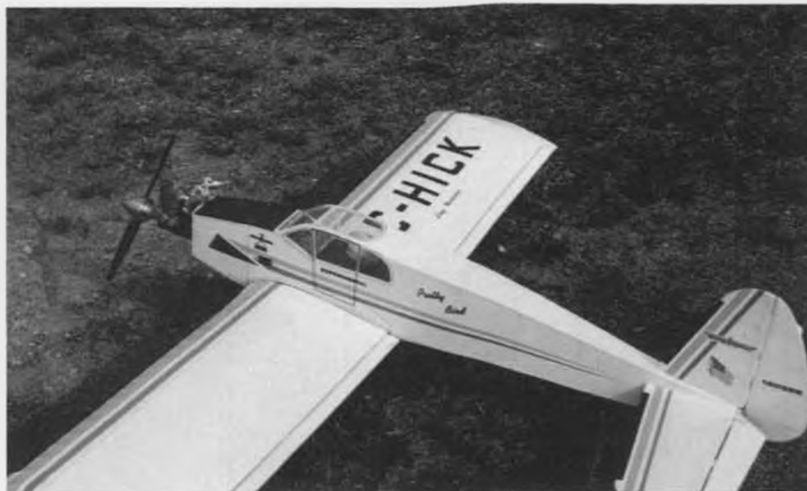
Pretty Bird's squarish lines show up well in this photo. A very functional airplane. Note how the top of the cabin is covered with clear plastic to simulate a "greenhouse" type of canopy.
