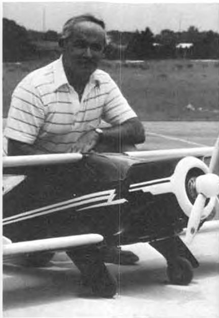
Photo at left shows Miami's Frank Reyes and his gorgeous black and white Beechcraft Staggerwing, built from the Byron kit. Frank installed a complete cabin interior, then found that the seats he'd put in were keeping the wheels from coming all the way up. His solution was to hinge the seats so that they are actually pushed up and out of the way by the retracting gear. Above: Every model gathering has to have at least one Cub. This clipped-wing version by an unidentified builder/pilot was probably built from the 1/4-scale Sig kit.
