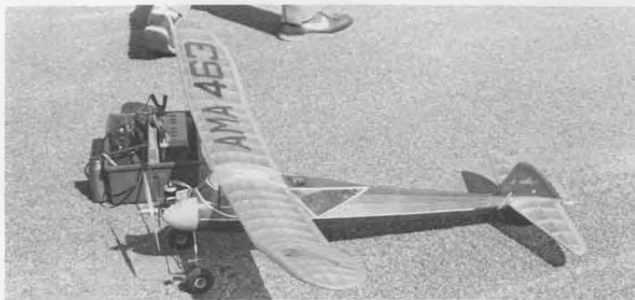
7. Andy Peterson's 1939 "Cruiser", reproduced by SAM president Jim Adams. Features a high aspect ratio wing and quite a long tail moment. Jim's flies with an O&R 23.
