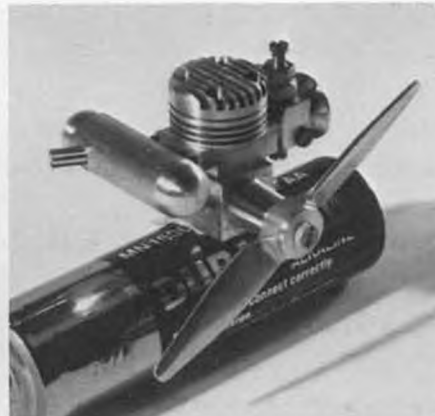
If you thought the old Cox .010 was tiny, have a look at this! Handmade diesel from Germany has about 1/8 the displacement of the .010. More details in text.
