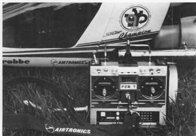
Webra powered Schluter Champion, one of the many test bed used by our author in his world helicopter speed record attempt project. Photo at right shows the Airtronics Spectra PCM7 radio used.
