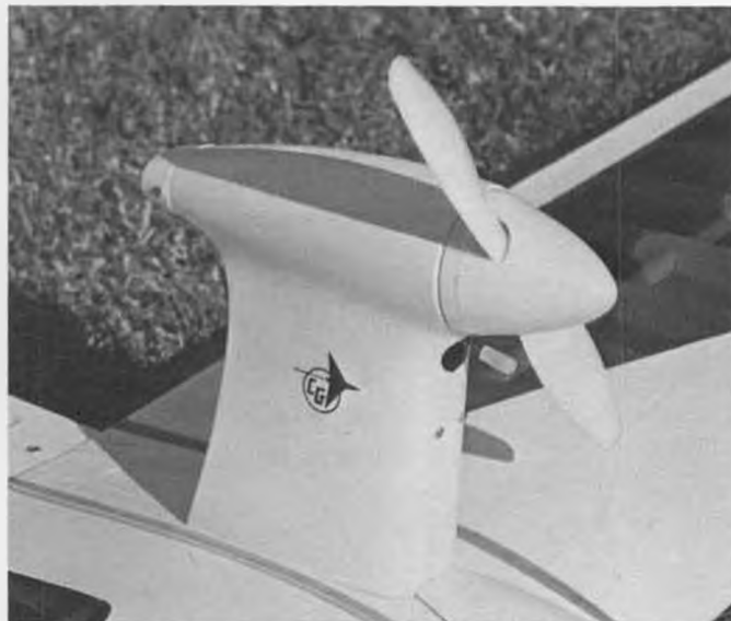
Plastic shells do a nice job of fairing in the motor pylon. Note the prop brake just below the spinner; improves glide by keeping the prop from free-wheeling when the motor is off.
