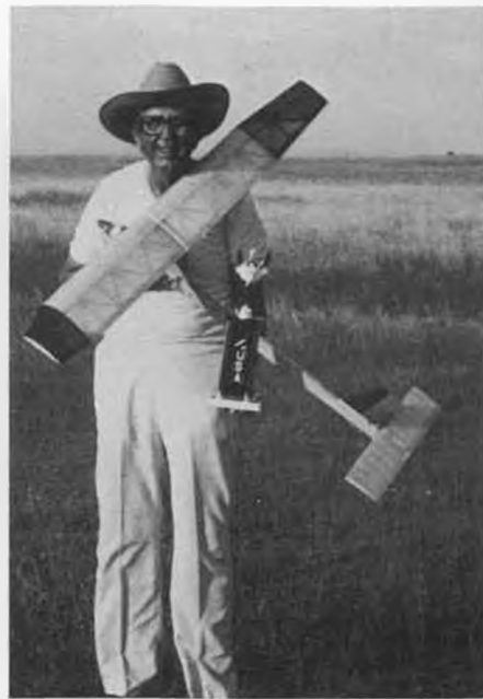
"Shocer Treatment" by Don Hughes won 1st in Class A Electric at '88 U.S. F/F Champs. Uses a Kyosho AP-29 motor, six cells.
