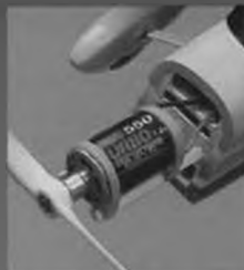
A standard 6 or 7 cell puck powers the shock-mounted Turbo 550 motor.
