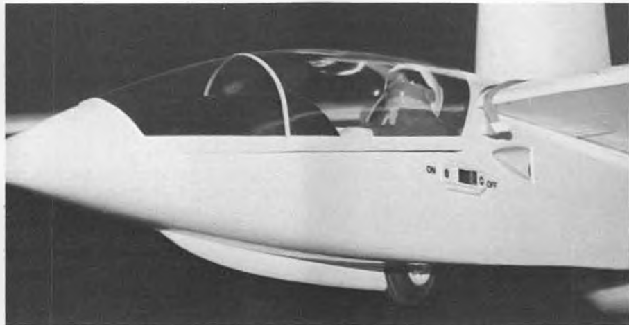
Note the air inlet scoop just under the wing i.e.; even though not shown on the plans, this is a necessary addition to provide proper battery cooling. Skip also added a wheel and skid, which help save the underside from damage when flying off of anything other than a grass field.
