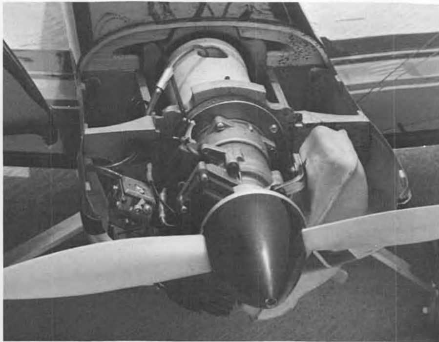
Engine installation details in Bob Godfrey's latest, the Ultimate 10 Dash 300S. Zenoah G-62 mounts on the front end of a piece of 4-inch-diameter PVC white plastic pipe, which in turn is held into the model by a series of rubber rings. In-flight smoke tank is inside the pipe just behind the engine; fuel tank is also in the pipe but farther aft, right at the model's balance point. Cleverly engineered mount reduces vibration transmitted to the airframe and radio.
