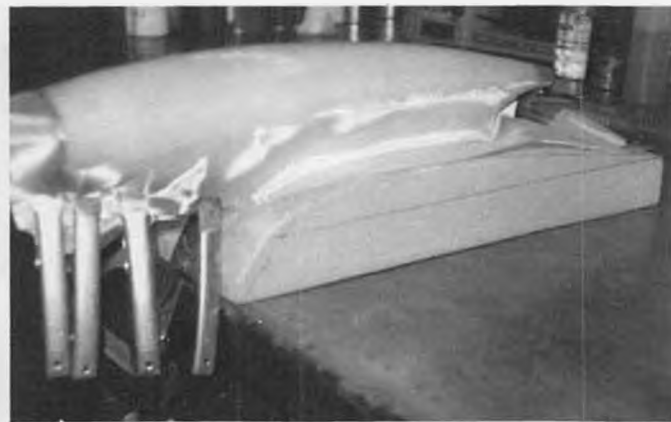
Fiberglass cloth draped over foam nacelle, ready for the epoxy bonding coat. Clamps act as weights to keep cloth in place.
