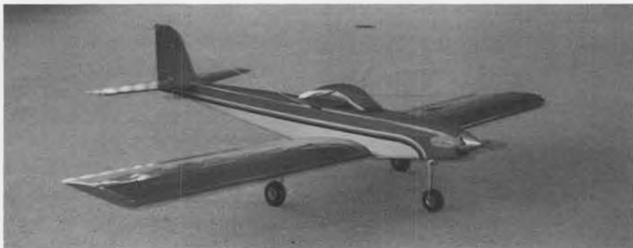
A nice building job on this Warlord 40 by Mike Kometz, powered by an Astro 40 cobalt. Electric conversion of the Bridi kit required no major mods.
