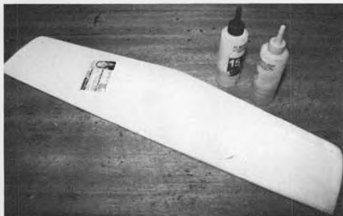
Our columnist uses plastic wallet cards — in this case an old driver's license — to squeegee epoxy into fiberglass cloth.
