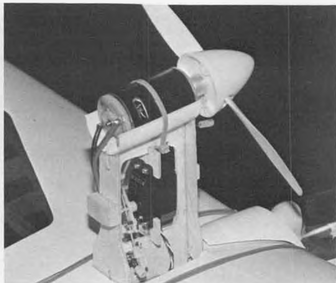
Motor control / prop brake servo is mounted inside the motor pylon. Makes for a bit of a squeeze but everything does fit. Power pod kit includes motor, prop, spinner, on-off switch, fuse, connector, etc.
