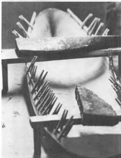
Photo 1: Sheer "horses" hold hull to eliminate twist while sheer clamps cure.
