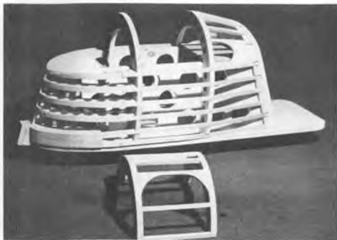
Uncovered framework reveals rugged construction that is a little unfamiliar to airplane modelers. Nevertheless, note lightening holes.
