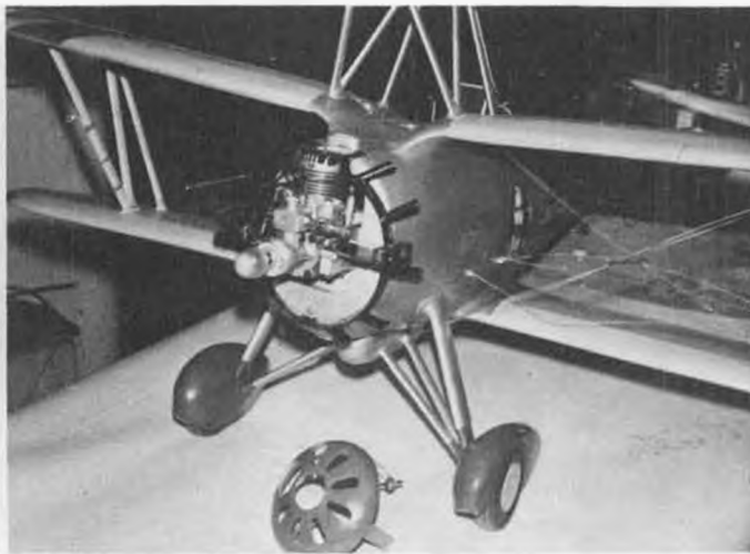
There's the Enya! Note exhaust ring. Fuselage is strip-planked over bulkheads. Shroud (foreground) is made from balsa.
