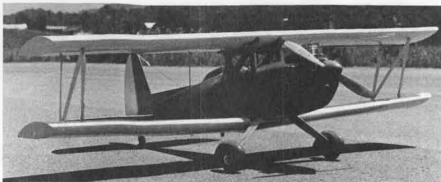
Another Stephens photo. This one is of Gary Paar's original Apex (Are you sure those cabanes are strong enough?). Cardboard-over-foam wings, 1/32 ply fuselage, OS .50. Materials cost $20.
