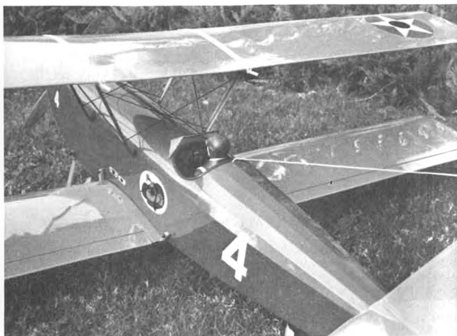
Another shot of John Pahlow's Big John, showing strip ailerons and canted cabane struts. Wings also have very slight sweepback. Nice covering job.
