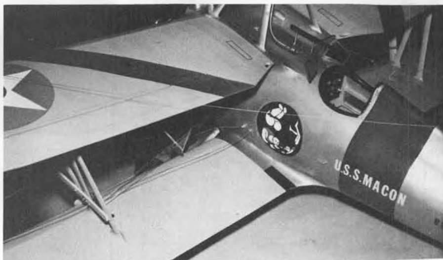
Note ailerons in upper wing only. Bottom wing has slight negative dihedral (anhedral), possibly to improve chord/gap ratio. Portions of wings covered after assembly. One-piece airplane.
