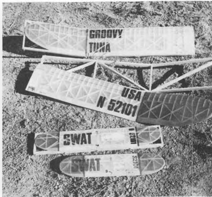
Wings and stabs are kept in jigs to prevent warps. A little extra care goes a long way. Note two sizes of stab; 44% and 33%. See text.
