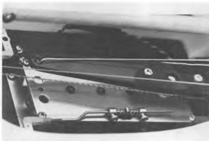
Operating lever to sail control limit switches is located between two adjustable override springs, to prevent servo burnout.
