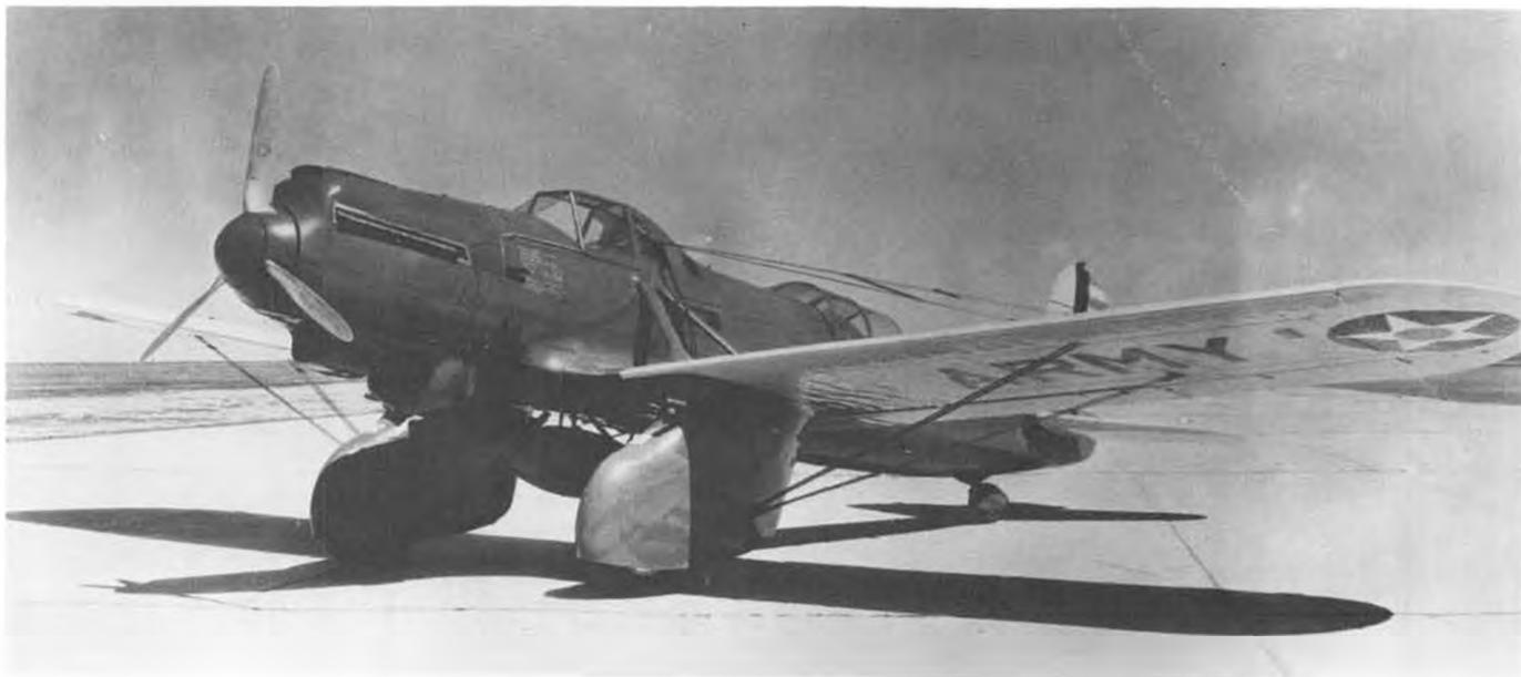
The Y1A-8. Two Browning .30 caliber guns were located in each massive wheel fairing, with 600 rounds for each.
