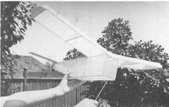
Built-up airplane kite, designed by the author, features model airplane-type construction. Open fuselage gives boxkite stability.
