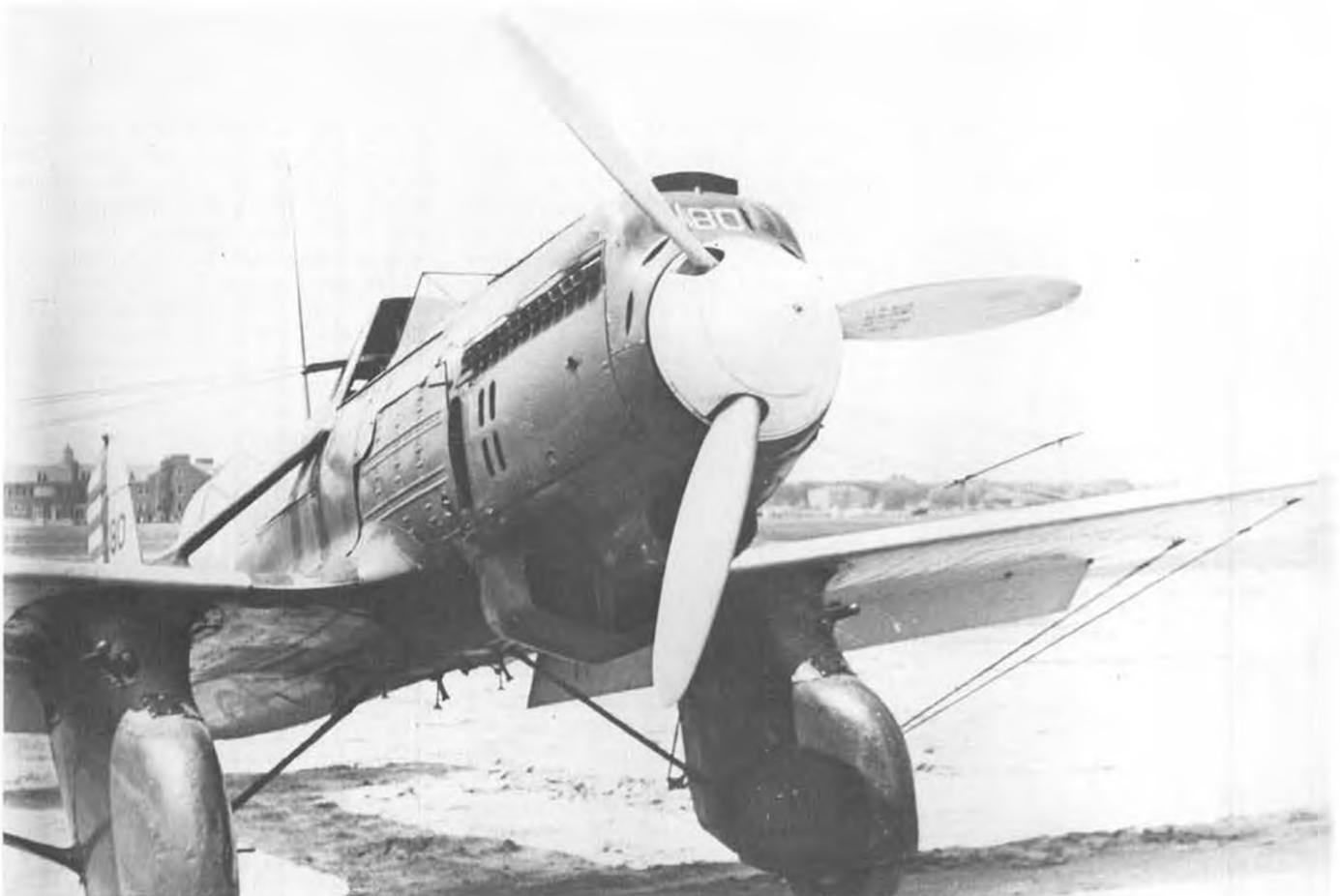
The A-8 was a tough, capable looking airplane. Oil tank was located on right side to obtain additional cooling. Fully cantilevered wings were still to be in the future. The A-8 was first Air Corps aircraft to have flaps and leading edge slats.
