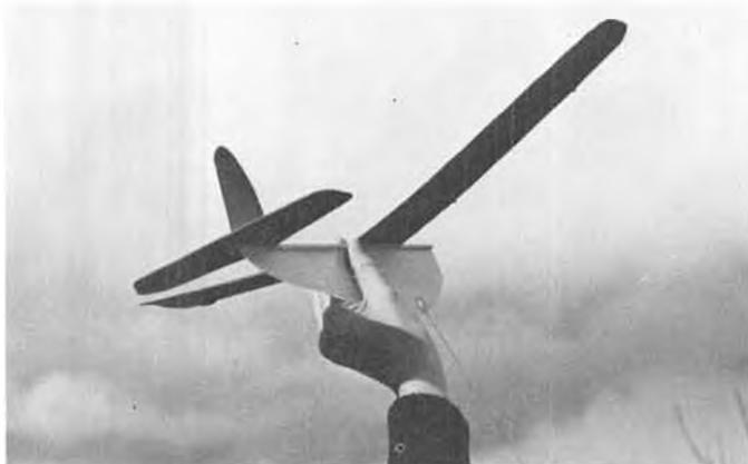
Scratch-built airplane kite designed by the author features balsa wing and tail surfaces. Flexible keel/fuselage is a sheet of typing paper.
