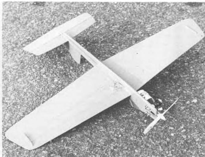
Control linkage, engine mount, and tank installation are all "outside" and easily accessible.
