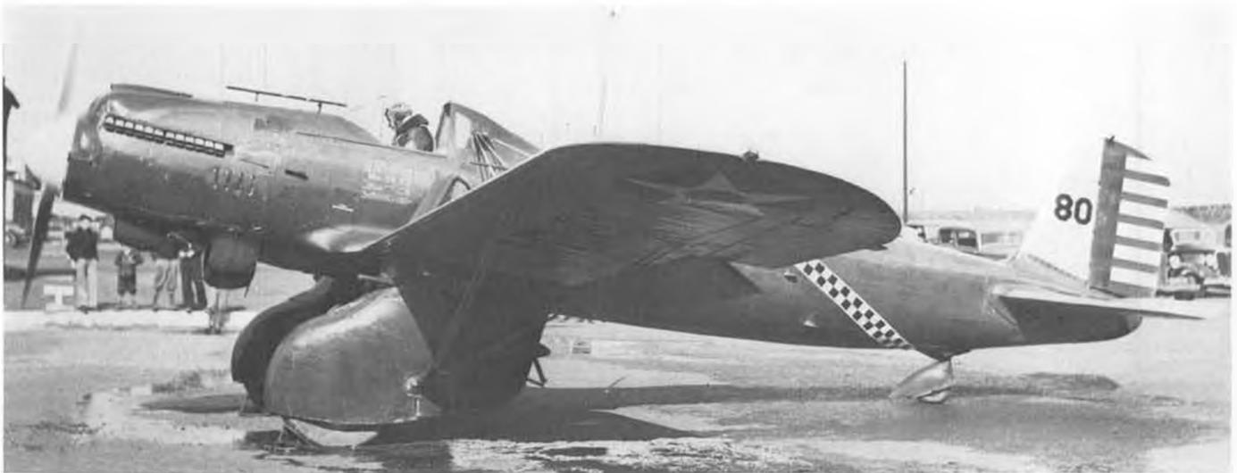
One of nine A-8's, while with the 37th Attack Squadron, Langley Field, Virginia. Note position of full-swiveling tail wheel. Control override system allowed steering when wheel was in the trailing position. See the knickers on the kids? Cars give away age of younger looking aircraft.
