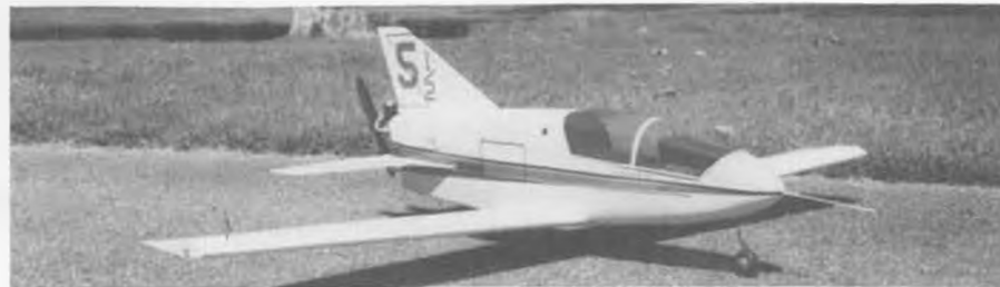
BD 5-1/2 (semi-scale) by M&H Hobbies. For 2-channel radio and TeeDee .049. Span is 43".
