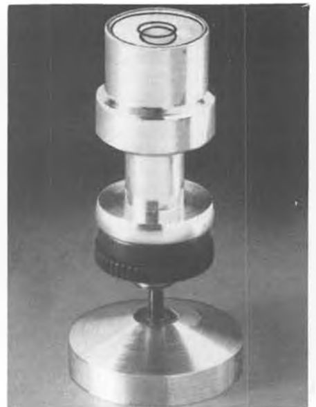
Super-scientific Bubble Balancer for props, by Howard Huebl.
