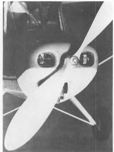
Close-up of Brown twin installation in modified Guillow Aeronca Champ, by Milan Kacha, of Czechoslovakia.
