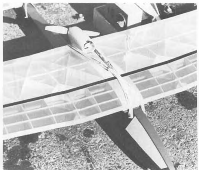
Close-up of Astro 10 mounting on Bernhardt's "Sky Sucker." Provides excellent air circulation for cooling motor.
