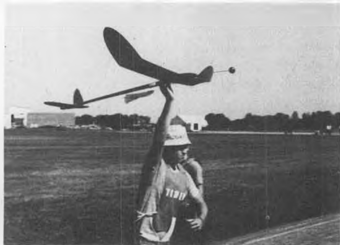
How do you add not too much nose weight, and also avoid increasing frontal area? Hang a golfball on the end of a piece of wire!
