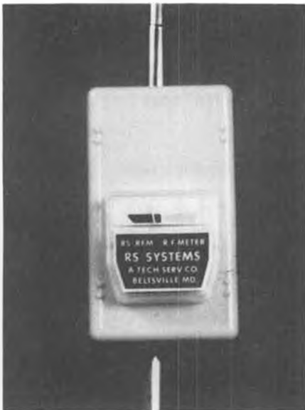
Clip-on meter for meterless transmitters, by RS Systems.
