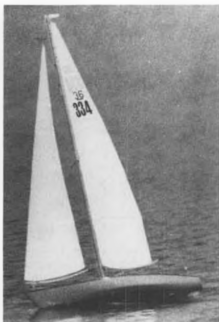
Ray Ozmun's 1976 ACCR winning 36/600 shows reasonable amount of twist in jib by shape of slot between jib leech and mast.
