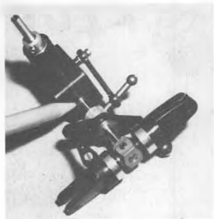
Pencil points to ball bearing in new Alouette tail rotor transmission.
