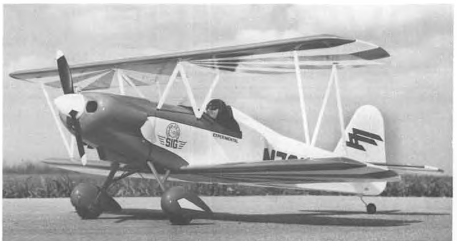
Mike Gretz designed Smith Miniplane, kitted by Sig. Span 44 inches, for .35 to .45 engines and four-channel radio.
