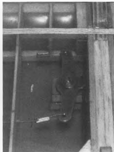
Bellcrank installation as seen through FasCal covering. Leadouts are old .018 combat lines.
